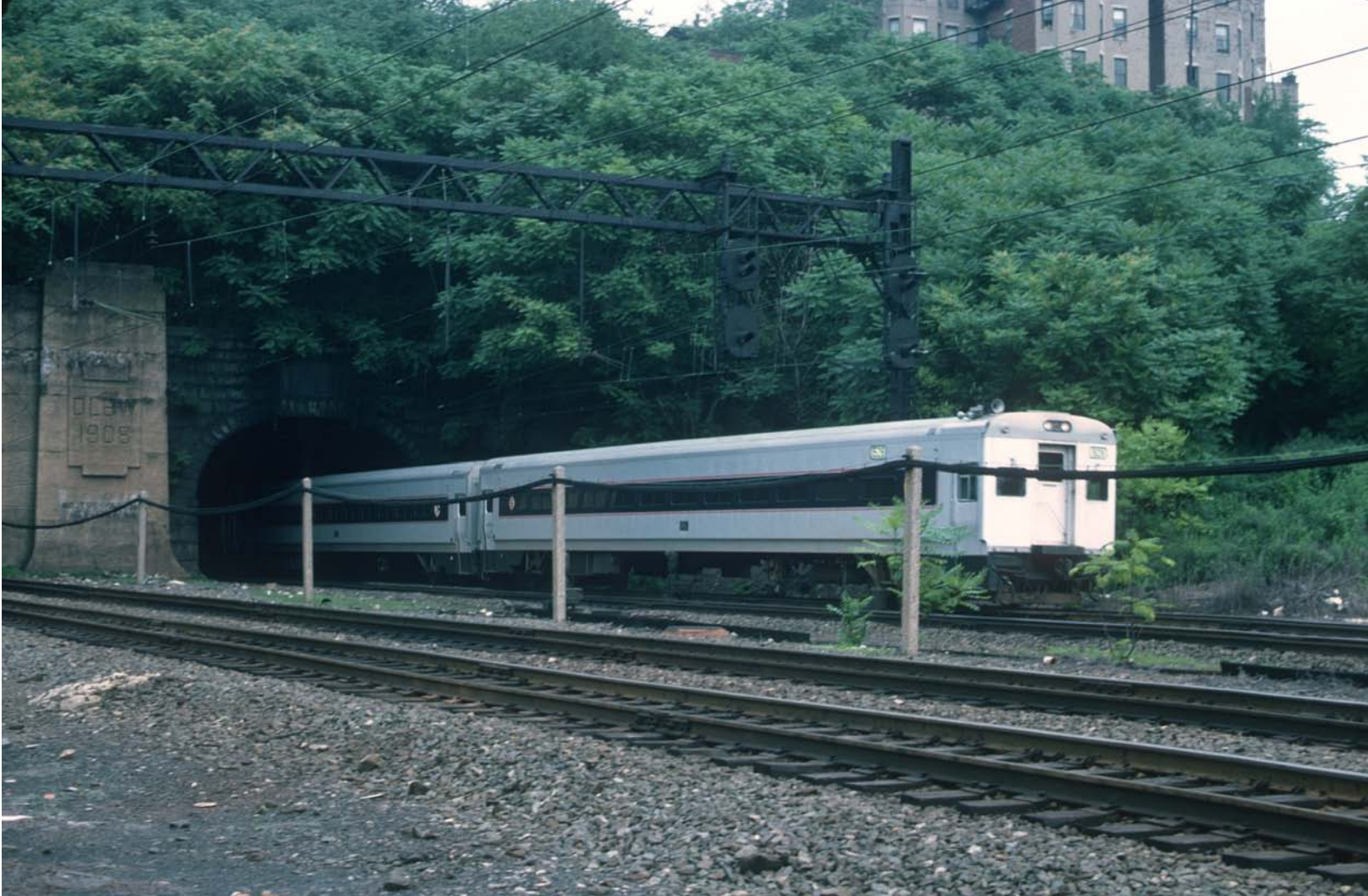
Above. (William Madden, circa 1975) An EL push-pull Comet car #1528 exits the east side at one of the two Bergen Hills tunnel portals. This train is heading toward the Hoboken Terminal in the early morning. NJ Transit commuters still travel through the Bergen Hills to reach Hoboken.
