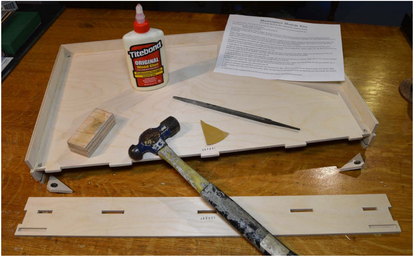
02 Above. This module kit can be assembled in one evening. File and sand all mating surfaces to make the parts fit firmly in place. Use a good quality wood glue to assemble the kit and work on a hard sturdy surface so the parts can be tapped into position until reaching the correct fit.
