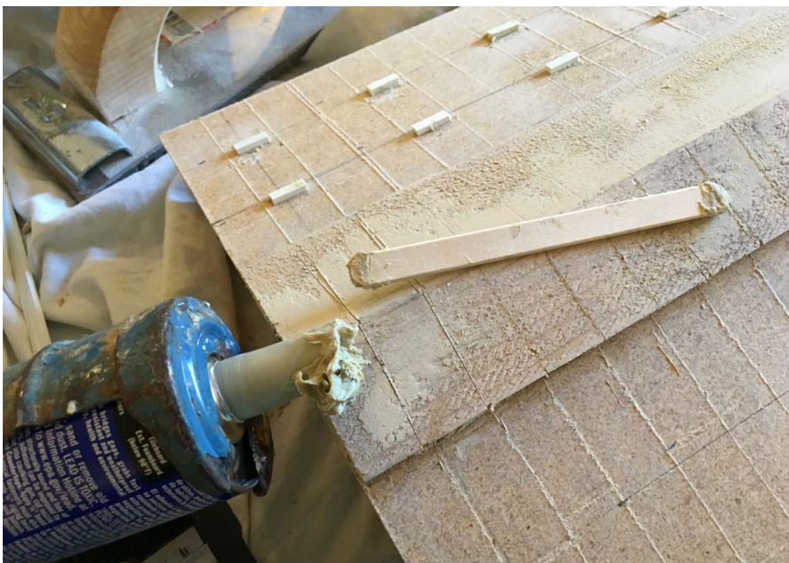
Above. Liquid nails can be a effective and affordable adhesive to attach the styrene to wood.
