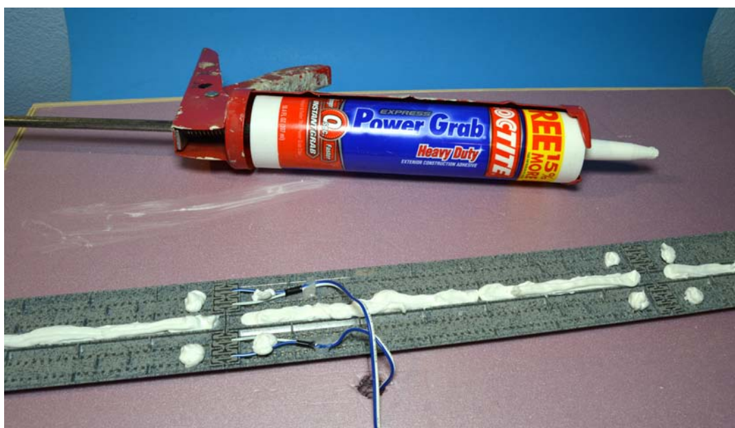
09 Left. Add a foam safe adhesive to the bottom of the track assembly at locations that contact the sub-roadbed.
