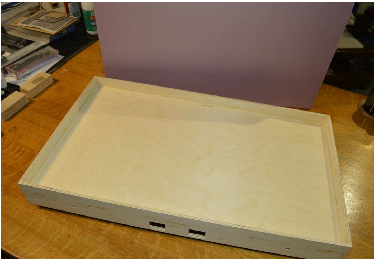
04 Above. If your using a depressed deck, cut a piece of 1" insulation Styrofoam for the recess and check for a snug fit.
