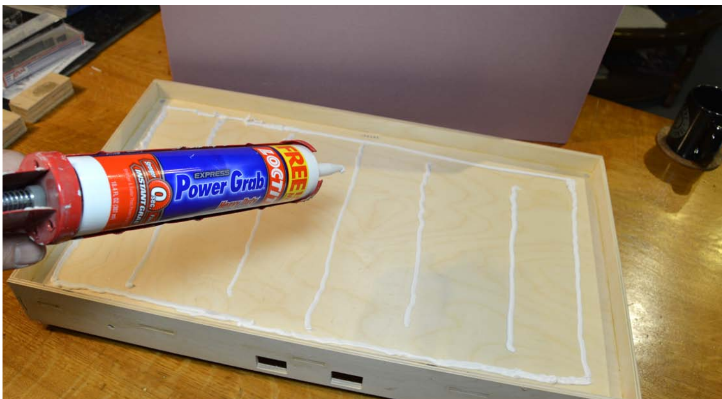
05 Above. Use a foam safe adhesive and apply a grid pattern in the recess of the module, then insert the Styrofoam
