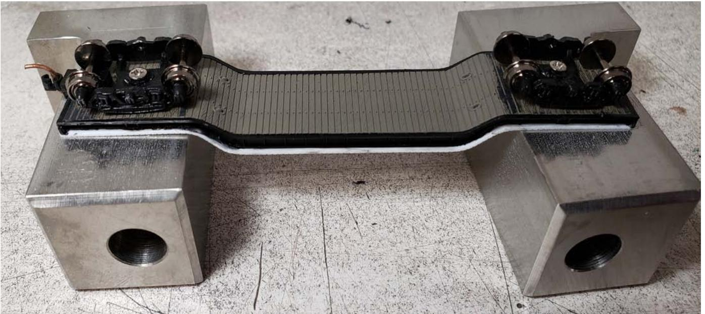
Fig 13. Here we see the couplers and trucks mounted to the car. This combo of trucks and couplers will place the coupler at the correct height.
