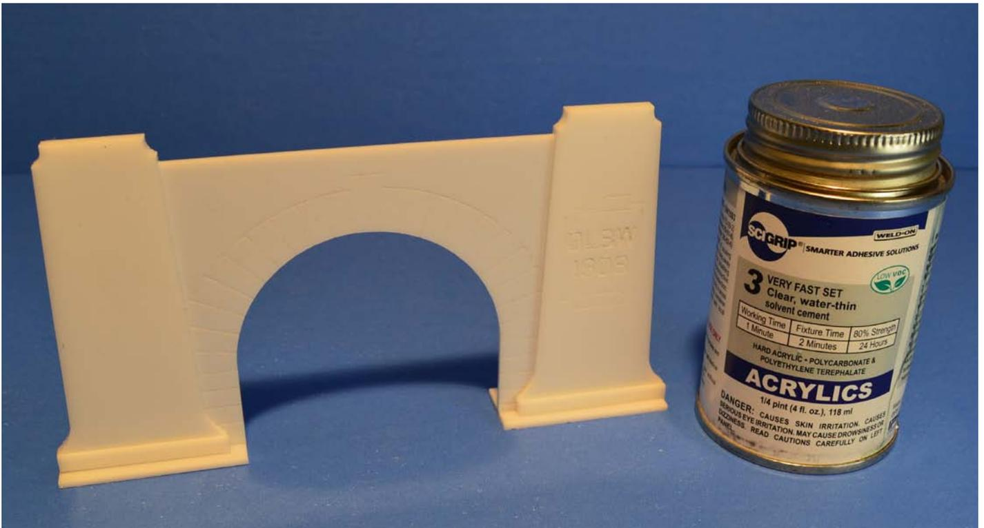
**05 Above.** Assembly. Once all the parts are manufactured, it's time to assemble the pieces. A thin paper layer that normally protects the sheet from scratches should be peeled off after the cutting process. Acrylics should be bonded with a compatible acrylic cement
