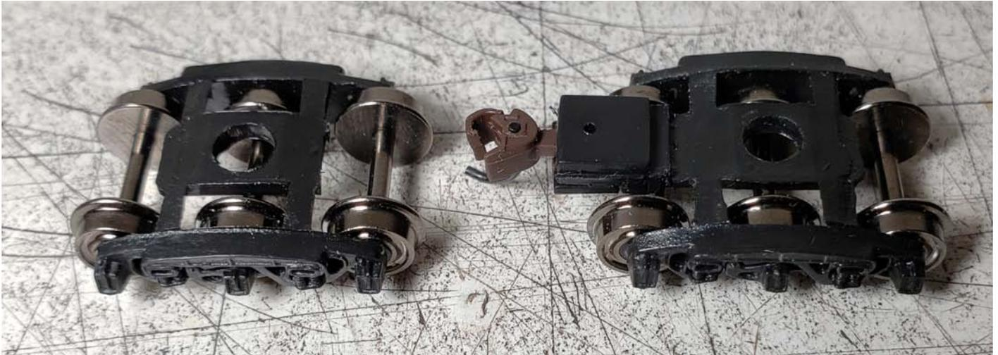
Fig 6. Lets turn our attention to the trucks now. I decided to reuse the Buckeye trucks that came with model. The side frames are a bit thick, however the relief is pretty good. Cut off the truck mounted coupler as shown on the truck on the left.
