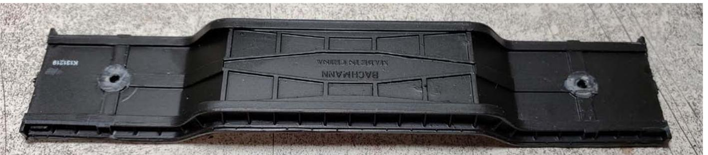
Fig 2. Flip the car over and remove the trucks. They are held in with a wood screw so you'll have to remove the center axle to access the screw. Then slice off the bolster flush with the body as shown here.
