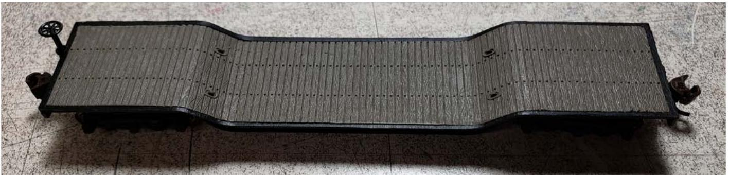
Fig 1. I didn't have any spare depressed center flat cars so I went on a quest at a local train show. Only one vendor had any, but what they had was just what I was looking for. It was a six axle undec Bachmann. These are decent cars. I like the three axle trucks. The brake wheel and couplers are a bit beefy but we'll change those.
