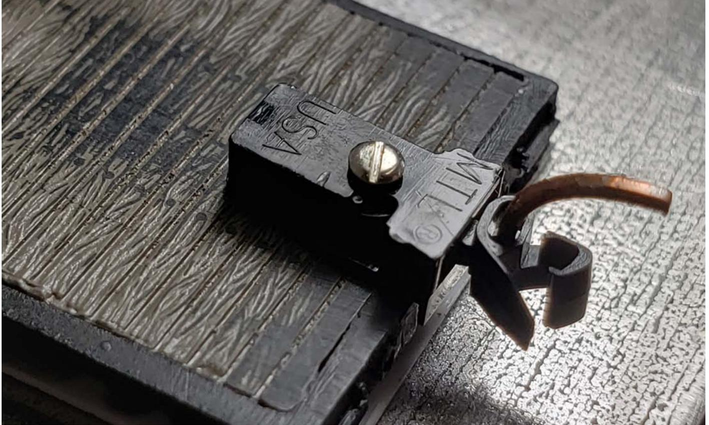
Fig 11. Lightly sand off the details on the former deck, now the underside of the car. Then mount MT 1023 couplers using a 00-90 screw that will go through the body but not hit the underside of the new deck. Nominally the screw can penetrate 3/32" into the car without touching the deck. The screws should self tap into the plastic.
