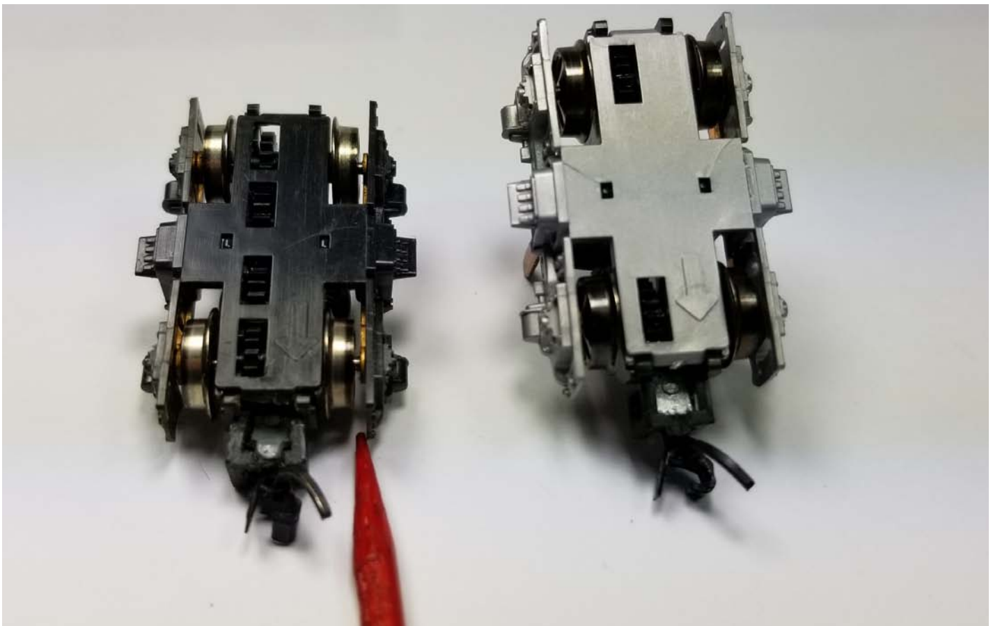
08 Above. At train shows it is very easy to spot the brass strips from the bottom of the trucks.
