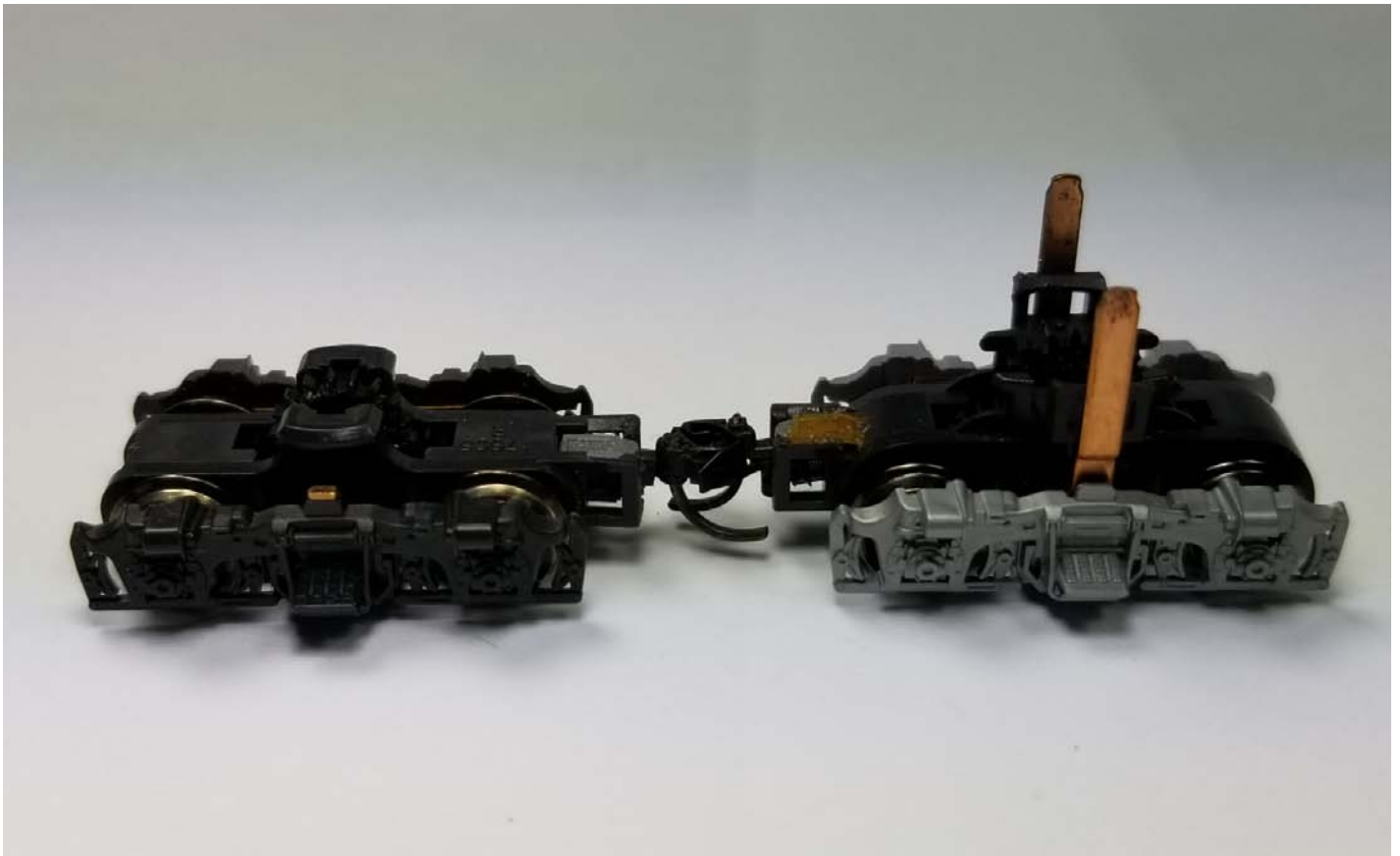
07 Above. Here are the revised on the left and the DCC on the right a side shoe shows the difference in the height of the brass strips.
