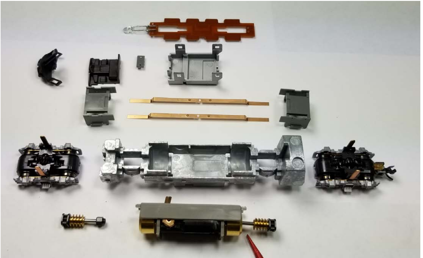
11 Above. This is the DCC unit broken down, note the one piece frame, careful not to bend the brass wipers, also this has only the outer bearing block and a joint that slides into the flywheel.
