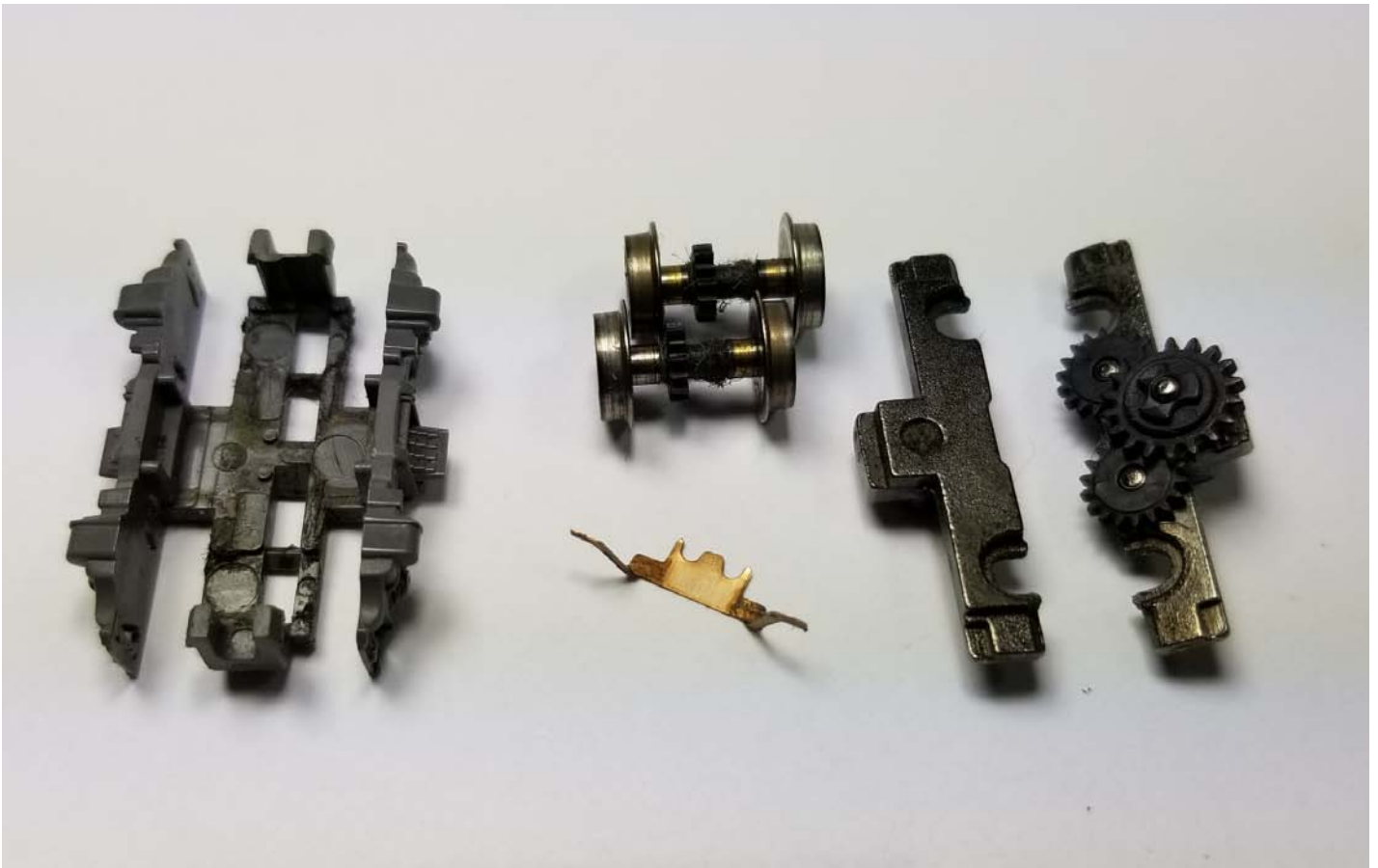
04 Above. Here is the original truck disassembled, note the brass wiper rubs the inside of only one side.
