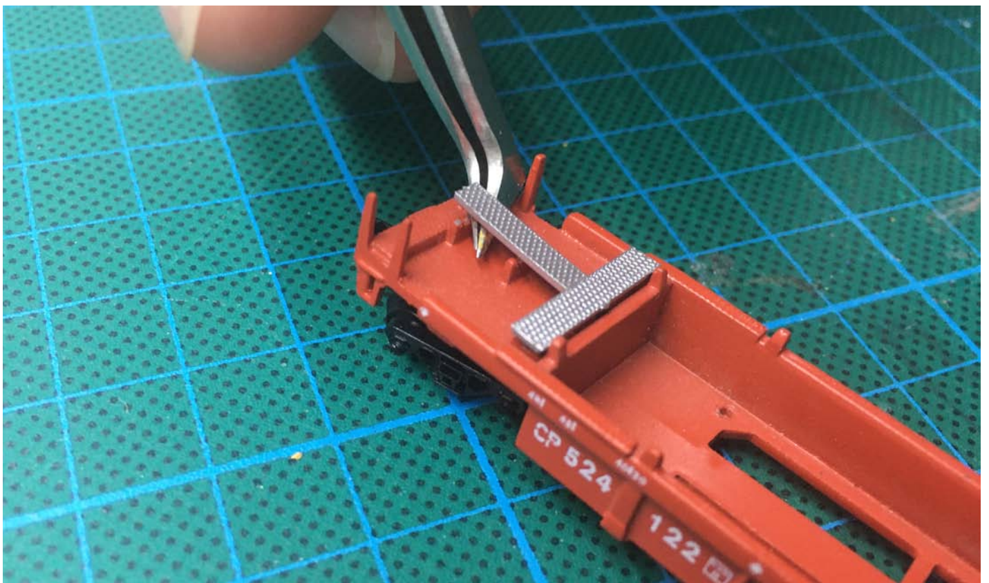
04 Above. I inserted the end of the tweezers under the old walkway and gently tipped them back, popping the old walkway's off of the supports.
