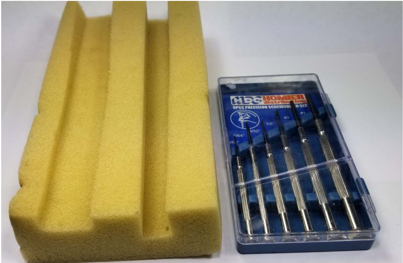
20 Above. Always good to have a cradle to keep the locomotive from moving while working on it and a small set of screwdrivers is required to work on these small engines.
