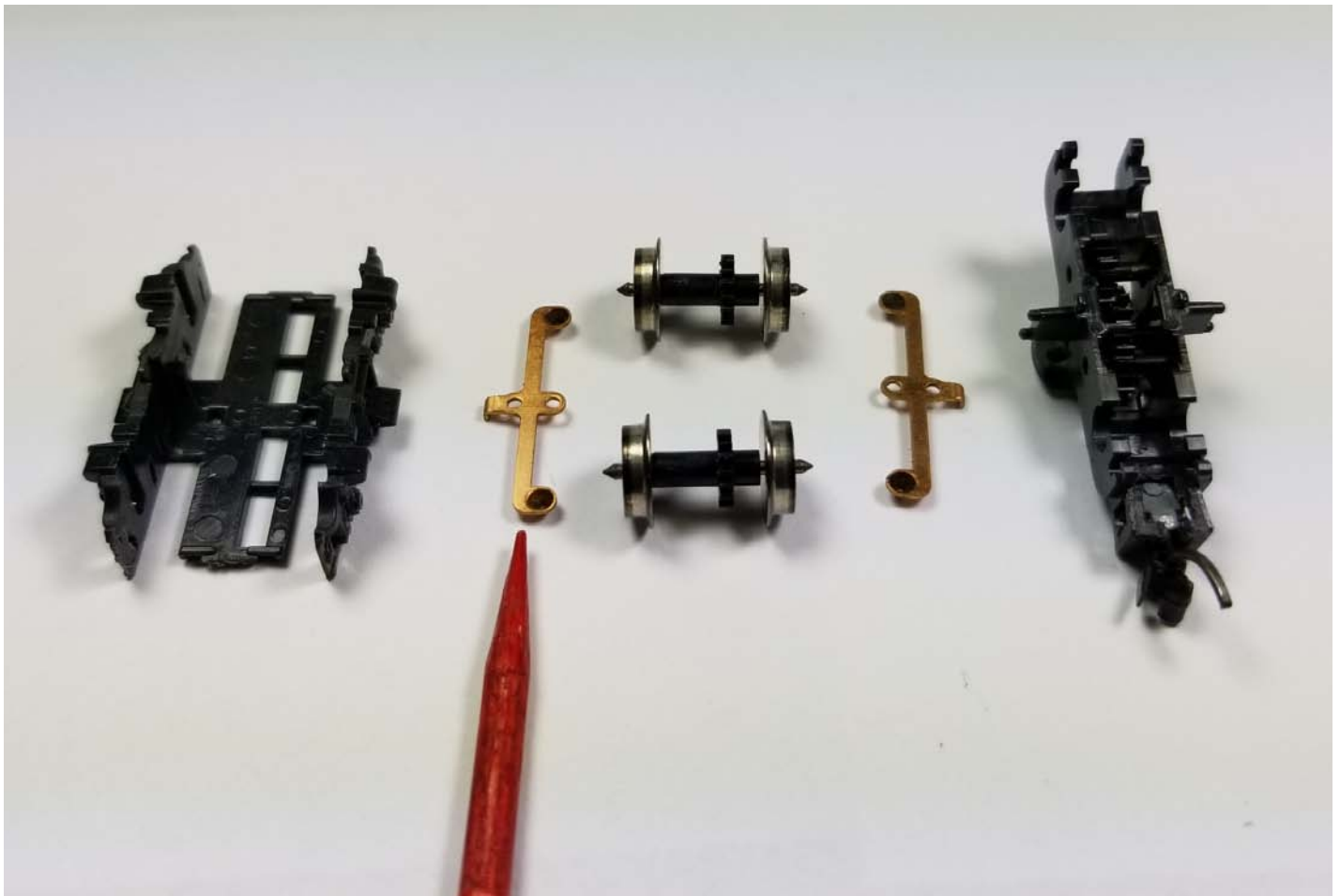
05 Above. This is the revised, note the pointer at the brass strip with the axle cups, over time these need to be cleaned too.
