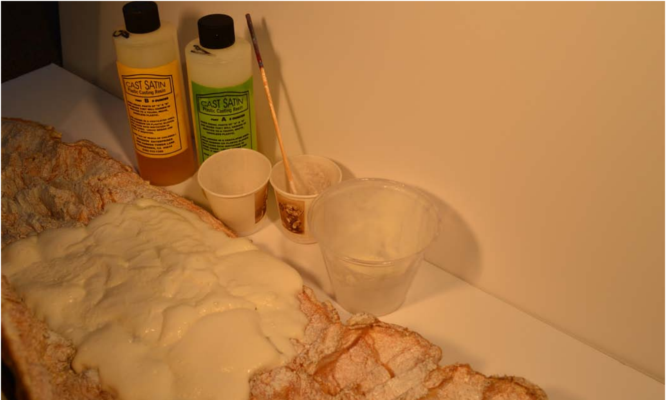
Above. I poured the Cast Satin into the mold area that I chose to replicate. I waited for the material to expand into the mold and waited for the material to set to a soft state. (5-7 minutes) I carefully started removing the cast from the mold and let it continue to harden before I started coloring the cast.
