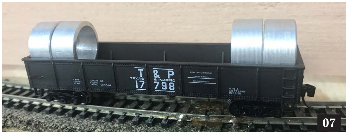
Image 07. Last step was installing a load. These coils are heavy, so four per car placed over the trucks is the way to go.
