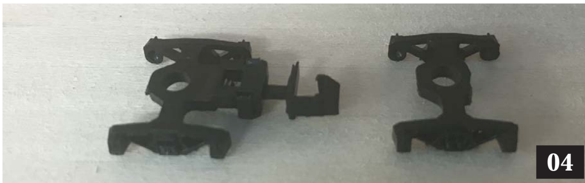
Image 04. Now I cut the Rapido couplers off of the trucks. I use a jeweler's saw. It takes less time to do it than it took me to type this text.
