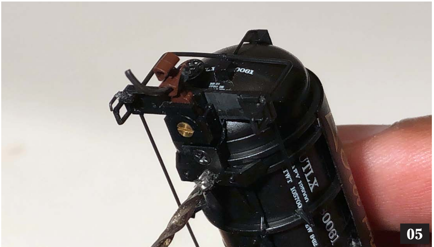
Image 05. Increasing the clearance of the bolster pin hole.
