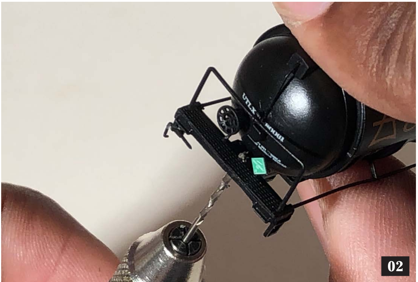
Image 02. Drilling the coupler screw hole.
