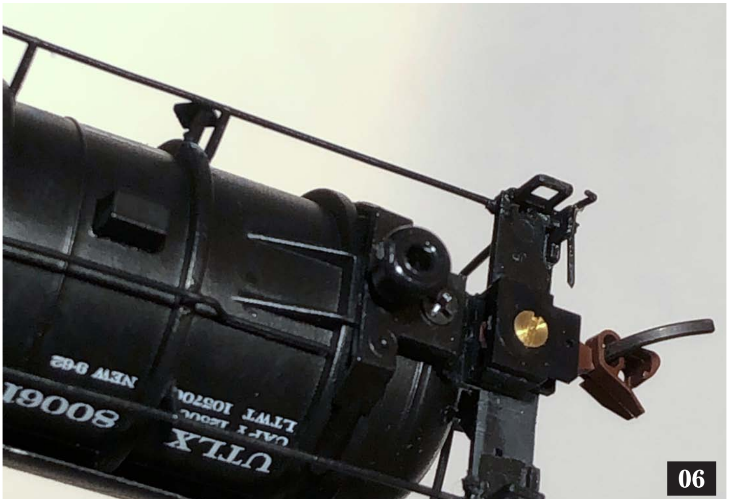
Image 06. Test fitting the Micro-Trains bolster pin.
