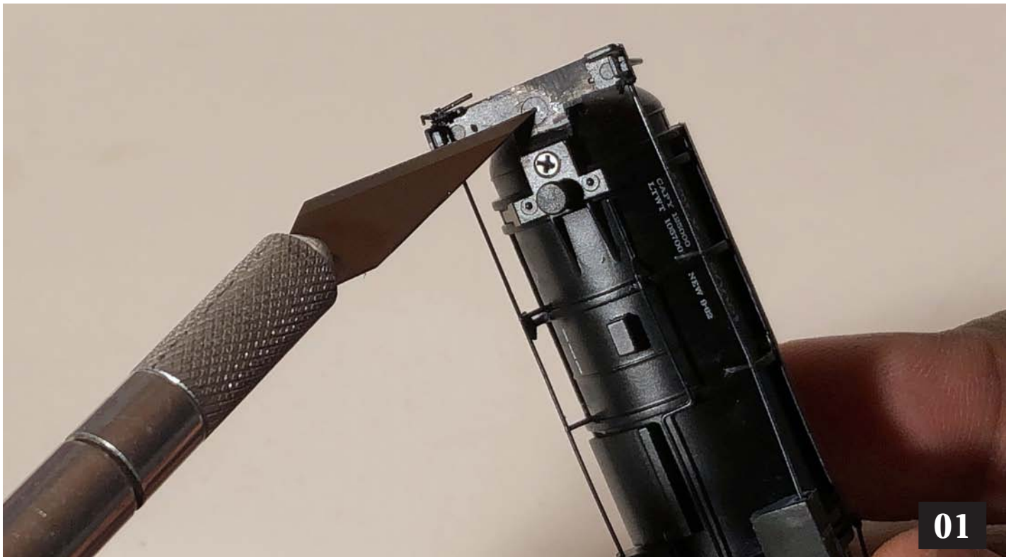
Image 01. Making the dimple for drilling the coupler screw hole.
