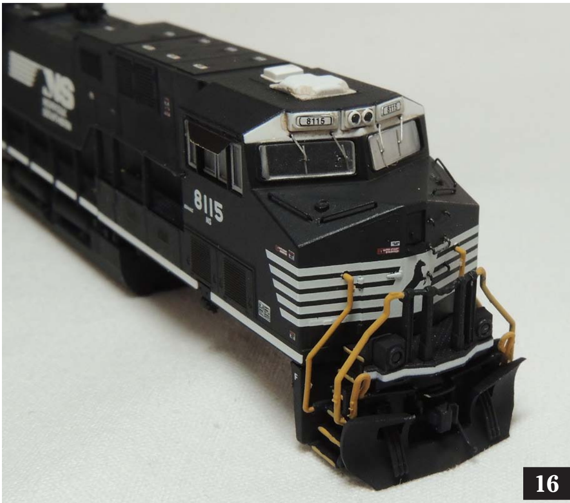
Image 16. As this was all for looks, I also swapped the couplers for Micro-Trains True Scale couplers, added TrainWorx wipers, and hit the locomotive with the Tamiya Panel Accent Fluid to start the build up of grime.
