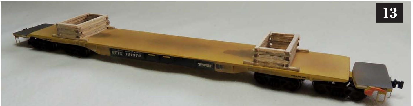
Image 13. Then I glued the cribbing to the deck of the flatcar.
