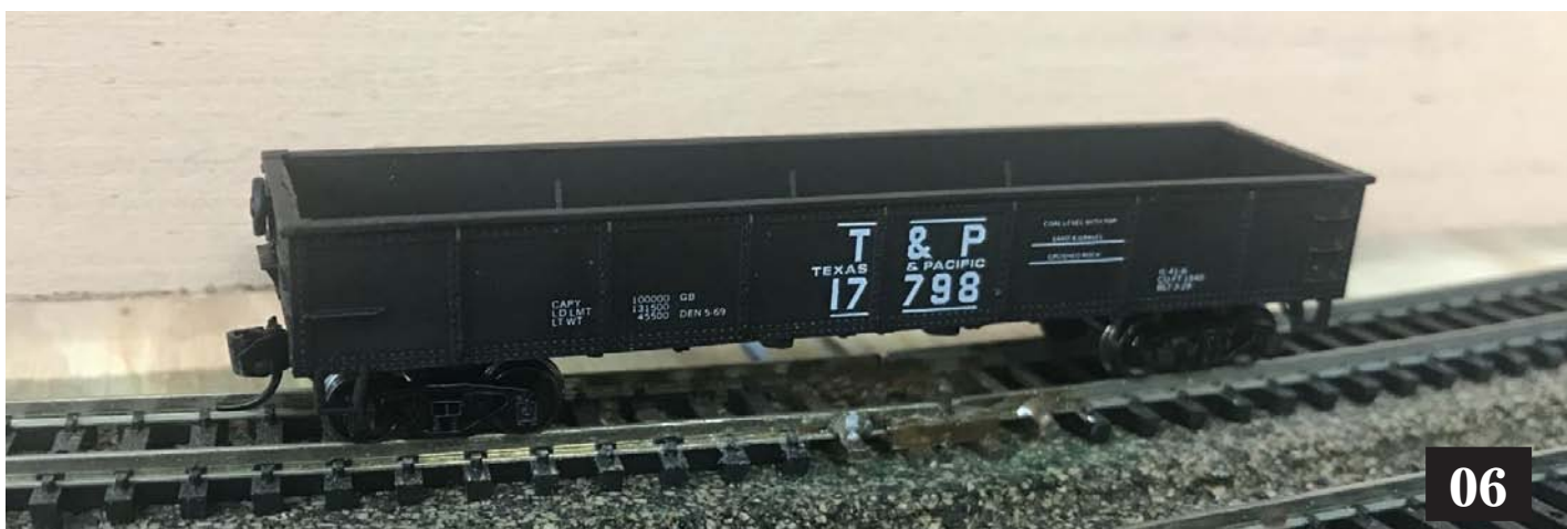
Image 06. I installed Micro-Trains 1015 couplers. The car looks much better than when I started!
