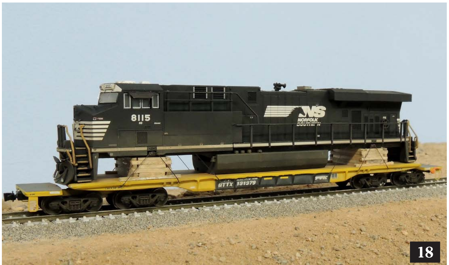
Image 18. Some black EZ Line from Berkshire Junction would replicate tie downs well. At this point the car is ready to haul this load back to its home shops for repair.
