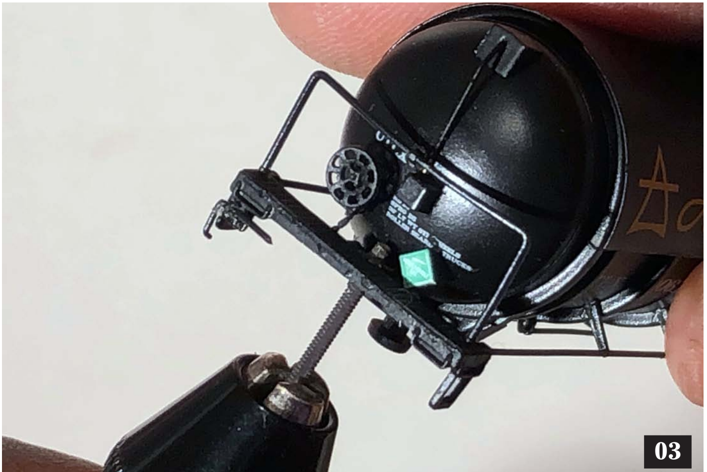
Image 03. Tapping the coupler screw hole.
