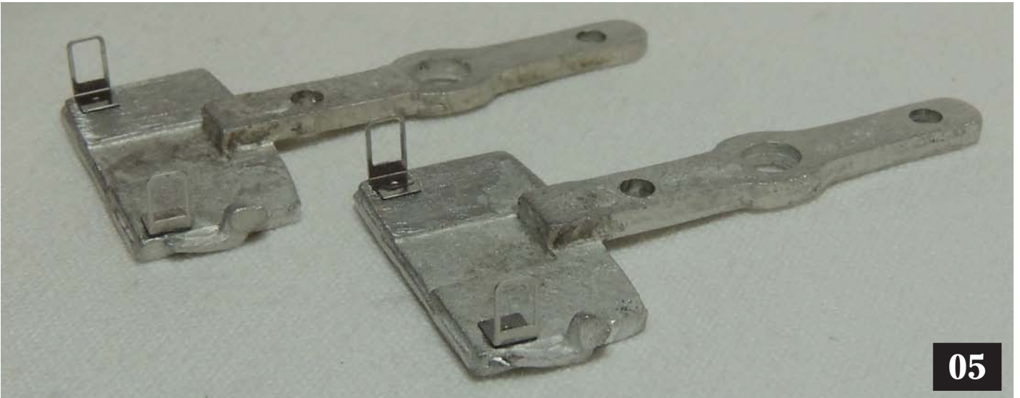
Image 05. Next, glue the etched stirrups to the end platforms.
