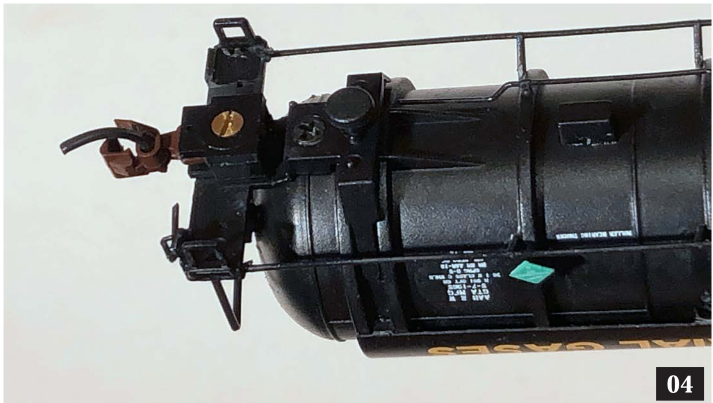
Image 04. Micro-Trains #1015 coupler installed.
