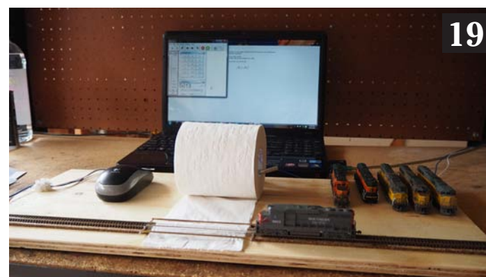
Step 19: I've placed my wheel cleaner in front of my computer that has JMRI running. I create a throttle in JMRI and put the slider to 90% speed and then my hands are free to hold the engine so it doesn't run away and I can move it laterally on the track for more effective cleaning of the wheels. Its amazing how effective this method is! ▶
