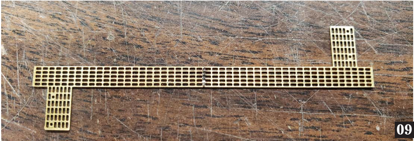
Image 9. For aesthetics its best to solder the two halves on the underside of the RB. Put a slight amount of flux on the edges of the two halves where they will be joined. Then drag a solder iron with a very small amount of solder on the tip over the joint to make the connection. Use a straight edge against the two halves to keep them in line while soldering. Using this method will keep the top side free from excess solder. File away any excess solder on the bottom.
