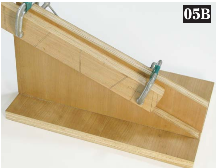
Image 05A and 05B. Make two quick jigs to drill consistent angles.
