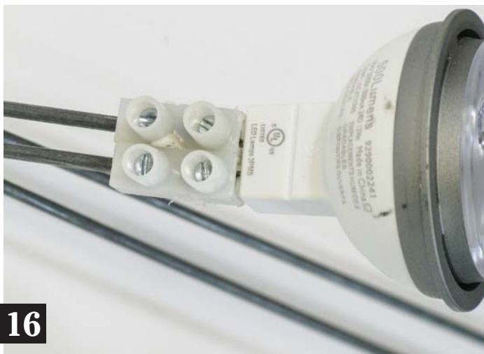
Image 16. Remove the web between terminals to fit spacing of MR-16 bulb
