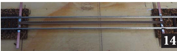
Step 14: Oh don't forget to cut a groove in the copper coating of the two sleepers in between the rails and the centre piece otherwise you'll have a dead short (Ask me how I learnt this!). My advice is to cut both side of each sleeper.
