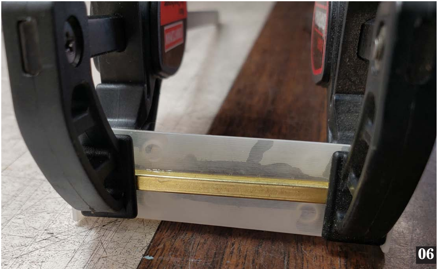
Image 6. For some reason the first batch Shapeway's printed had a bow to the roof. Ribs were added longitudinally on the underside to address that for future printing. The approach I took was to glue a 1/8" piece of square brass tubing on the underside to take the bow out. CA worked good for this application.
