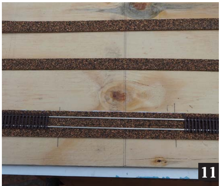
Step 11: Whilst the glue is drying from the previous step, place a piece of track over the cork and remove the sleepers across the width of the two marks made earlier
