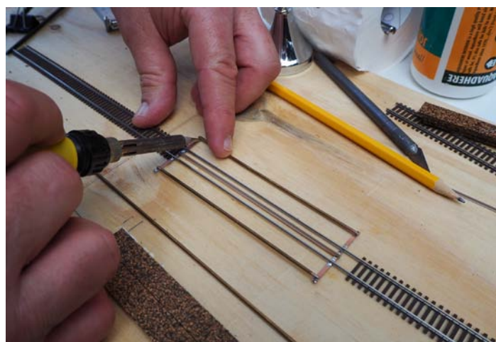
Step 15 and 16: Measure the brass round bar and cut to length of the two sleepers and parallel with the track. Then solder these on the outside of each sleeper.
