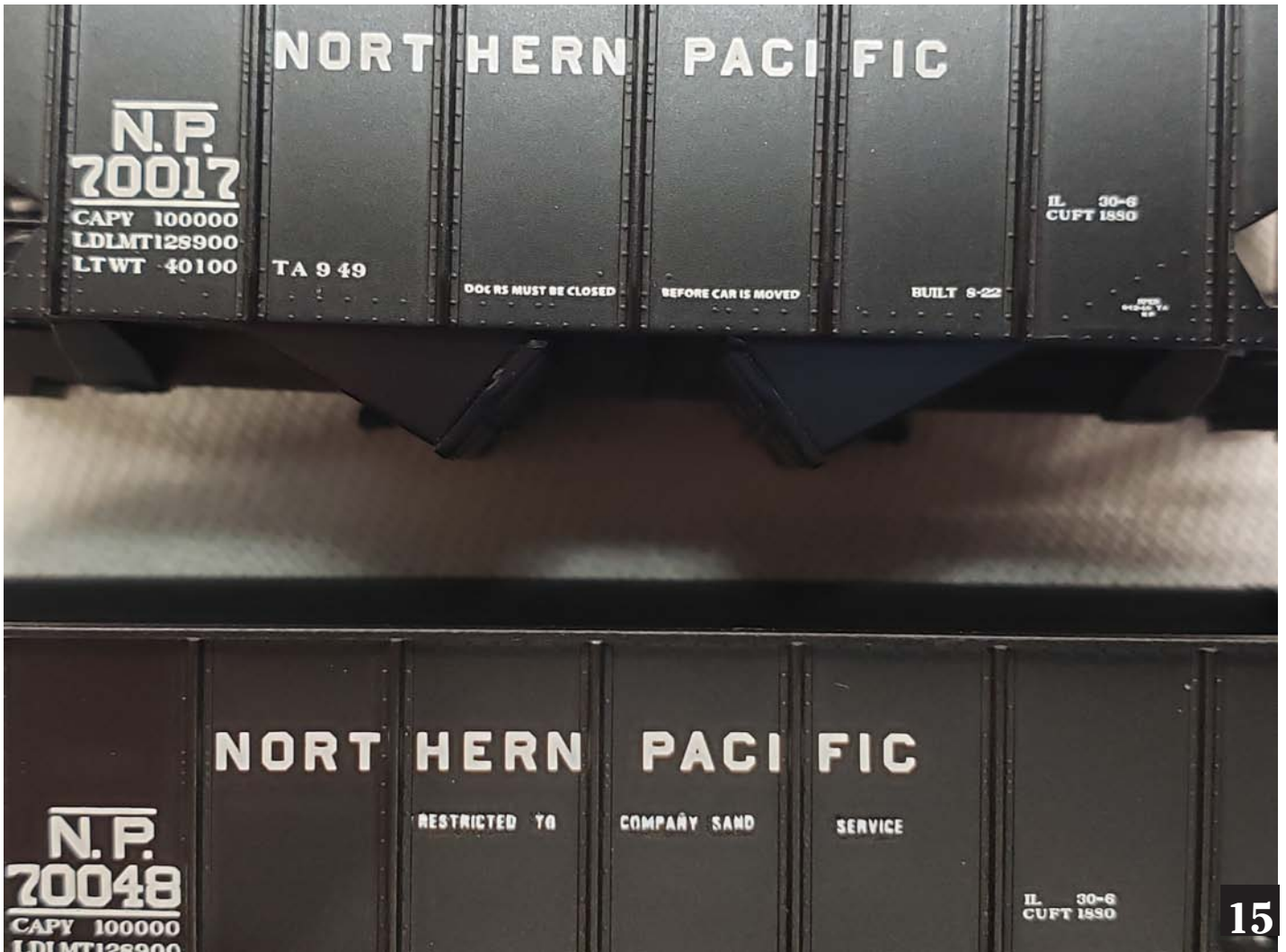
Image 15. There was one change I made to the lettering. Microscale set 60-1011, NP MOW has the decal “restricted to company sand service”. I added this to the NP decorated hoppers because it’s noticeable. Other changes you could make would be to remove the bars above and below the reporting marks. Also the correct road numbers are in the 207400 to 207448 range. I chose to do neither because the visual payoff did not offset the effort required.
