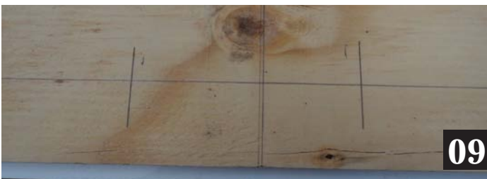
Step 09: Mark 2 lines across the center line about 12mm wider than the toilet paper on either side. Mine is slightly off set. These will be where the ties will need to be removed from the rail in a later step.
