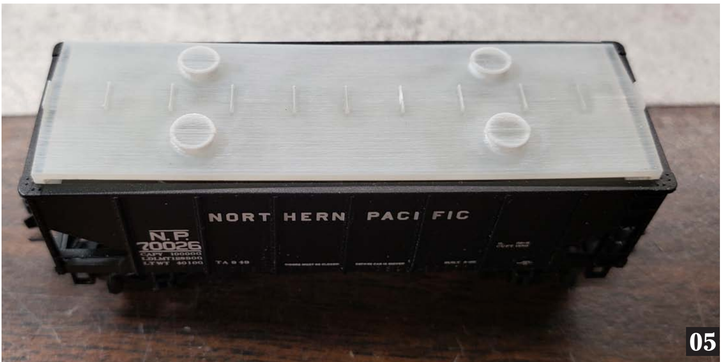
Image 5. Here is a photo of the roof partially inserted for a test fit. It's a snug enough fit I had concerns about being able to get it back out, hence only partially in for this test fit. It's not the length that's snug. It's the width of the ends that are slightly wide.
