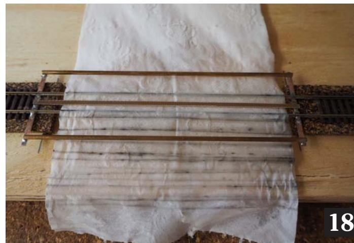
Step 18: NOW YOUR READY TO CLEAN WHEELS Apply your track power to the rails as per your normal process. You can use alligator clipped leads for a temporary fixture or hard wire as I've done for a more permanent solution. Place a locomotive on the track and run it forward to the paper. Apply your cleaning solution and away you go. This will speed up your wheel cleaning process by double and be so much simpler and easy to use. As your paper gets dirty just pull it through to a clean section.
