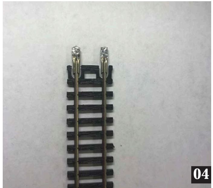
Image 04. Get out the soldering iron and tin the flattened side of the rail joiners.
