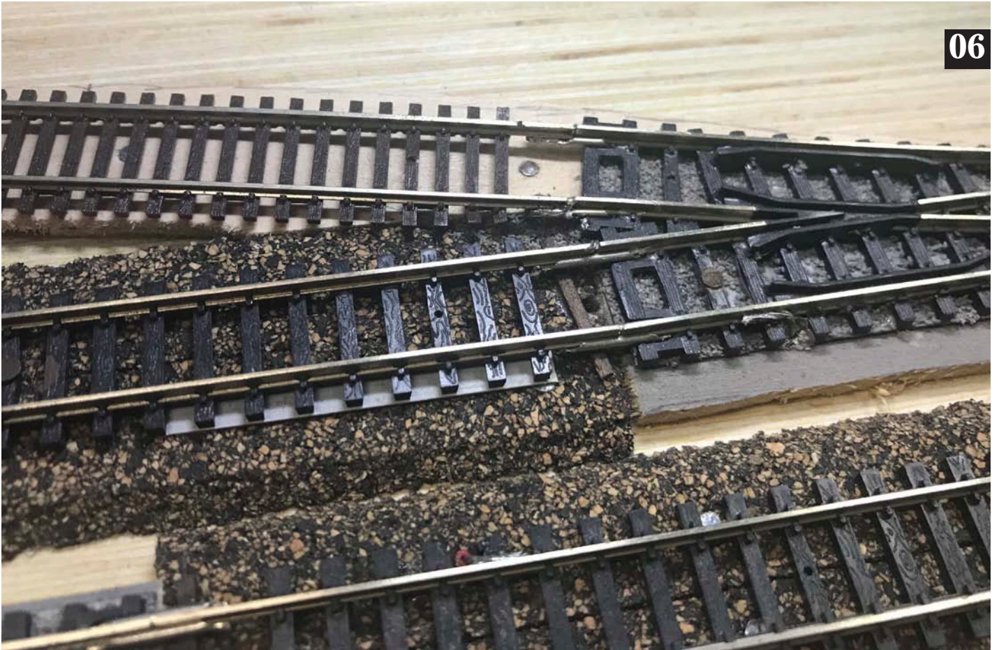
Image 06. Solder the code 55 track to the flattened rail joiners. It is easy to keep the track aligned side to side as the solder adheres and the tops of the rails will match quite well. If there is a slight variation, or bump, a couple of swipes with a file will get you on the right track!
