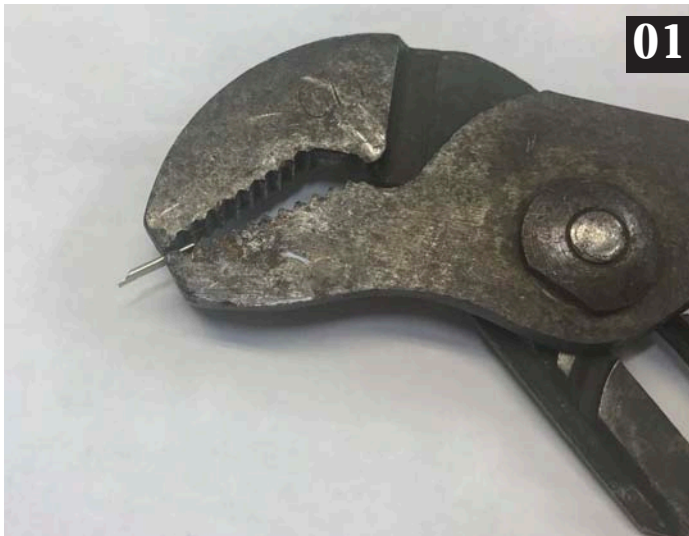
Image 01. First step is to take a code 80 rail joiner and flatten one half of the joiner with a pair of pliers. Make sure the flattened part is relatively level with the bottom of the unmodified half.
