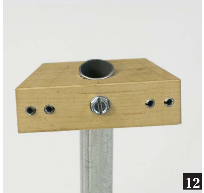
Image 12. A sheet metal screw holds the Block to the Pole
