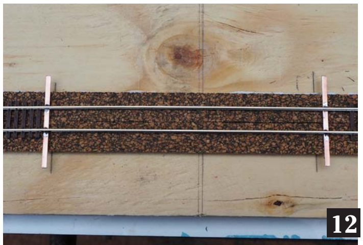
Step 12: Cut two pieces of Copper clad printed circuit board and solder these to the rails just inside of where you removed the sleepers. This will hold the rail gauge more rigid.
