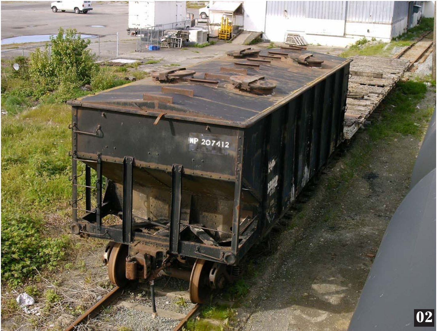
Image 2. This shows what the added roof looks like minus the running board on a retired car. It's fairly basic with 4 hatches and supports for the running board. This car is currently residing in Toppenish Northern Pacific Railway museum. (Photo by Doug Shearer, used with permission)
