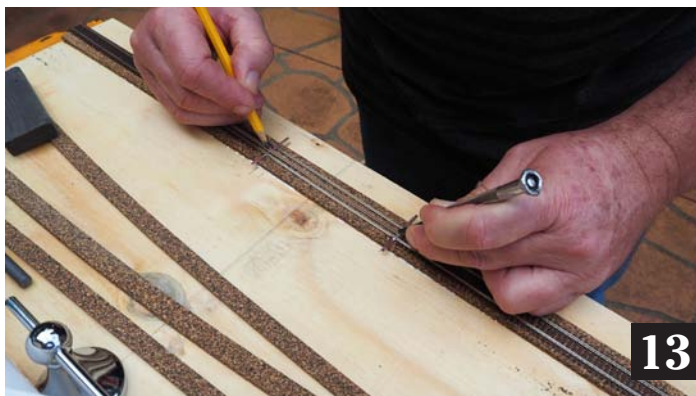
Step 13: Place a length of copper clad printed circuit board parallel with the track center line and across the top of the 2 previously installed printed circuit board sleepers. Mark this to length and cut. Place this down the centre of the track and across the two copper clad sleepers. Center between the rails and solder to the two sleepers
