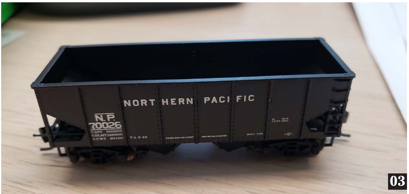
Image 3. Fortunately for us in N Scale, Bluford Shops makes just the right hopper for the base of this conversion. It is listed as a USRA 30' 6" 2 bay hopper, AKA USRA 55 ton hopper. They come in a paint scheme that is correct for the NP 70000-70048 series but is a little older than the scheme used for the 1957 conversions to the 207400-207448 series. The main difference being lines above and below the reporting marks vs. no lines. The factory coal load has been removed in this photo.
