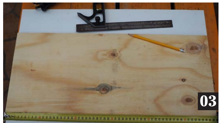
Step 03: Mark out the center line of the piece of wood sheet you are going to use. Mine was rectangular and about 500mm long by 300 mm wide. On the center line at about 50mm in from the top drill and screw on the toilet roll retaining bracket
