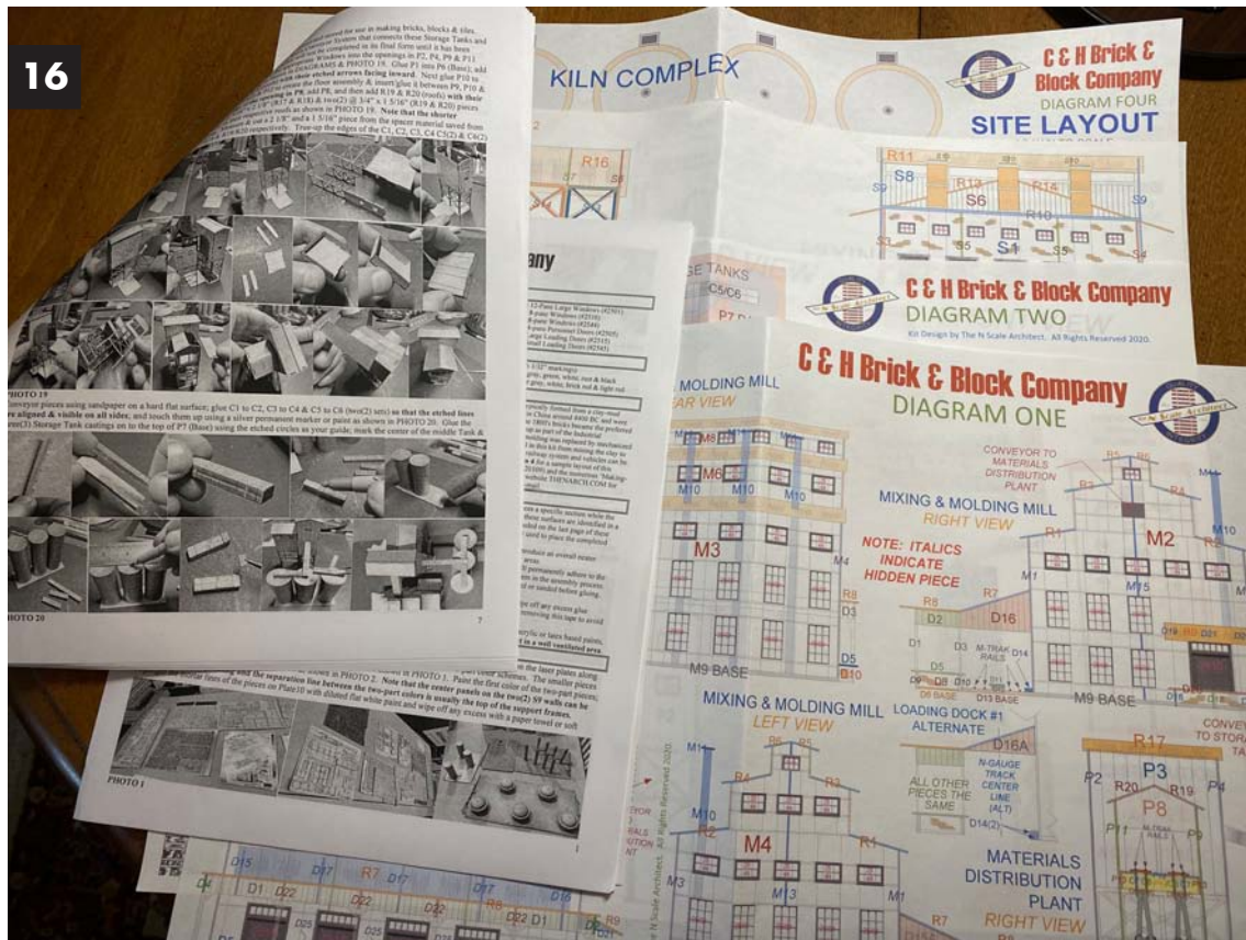
The photos, words and drawings are all part of our extensive instruction package while the test builds are not only used to check the fit of the parts but also to identify the most logical construction sequence. This sequence accounts for drying
