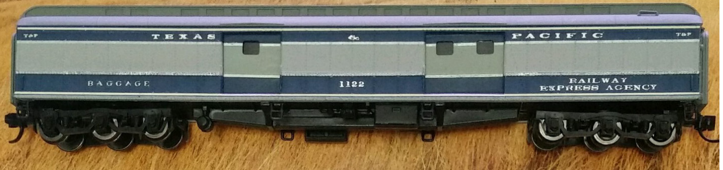
Image 03. The baggage-express cars on the Louisiana Daylight were constructed by American Car & Foundry in 1925 and numbered 1101-1132, Wheels of Time's models of these cars painted in The Eagle scheme were numbered 1117, 1120, 1125 and 1124, so I used other numbers in the series for the cars painted by Ernie Giese. This car, 1122, has had its original paneled wooden doors replaced by ply-metal doors, but has yet to be further
