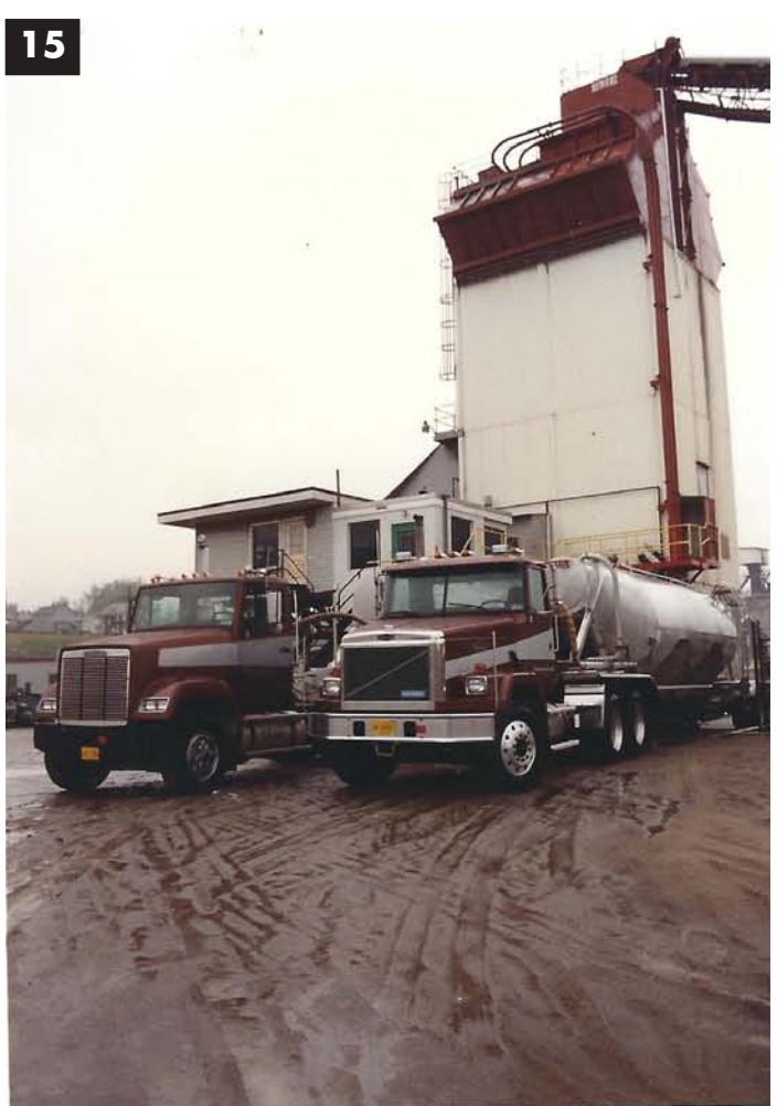
Image 15. Gloomy day in Erie, PA, again. Two tankers unloading into Erie Strayer stack up plant. Note red piping for cement going up outside of white siding. ▶
