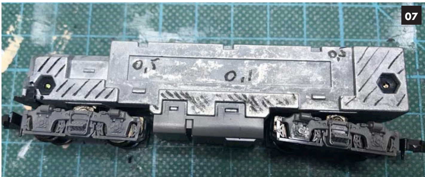
Image 07. Disassemble and prepare the Kato mechanisms. Please refer to Gordon's article in NSR #120 on how to disassemble the engines. He has provided a very detailed description of the process. Also it might be a good idea to do the basic maintenance that he has described.
