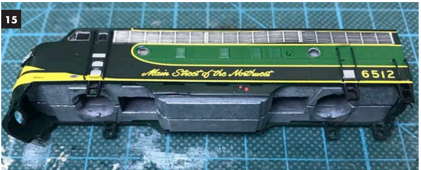
Image 15. This is what we are looking for: a nice, level fit of the shell.
