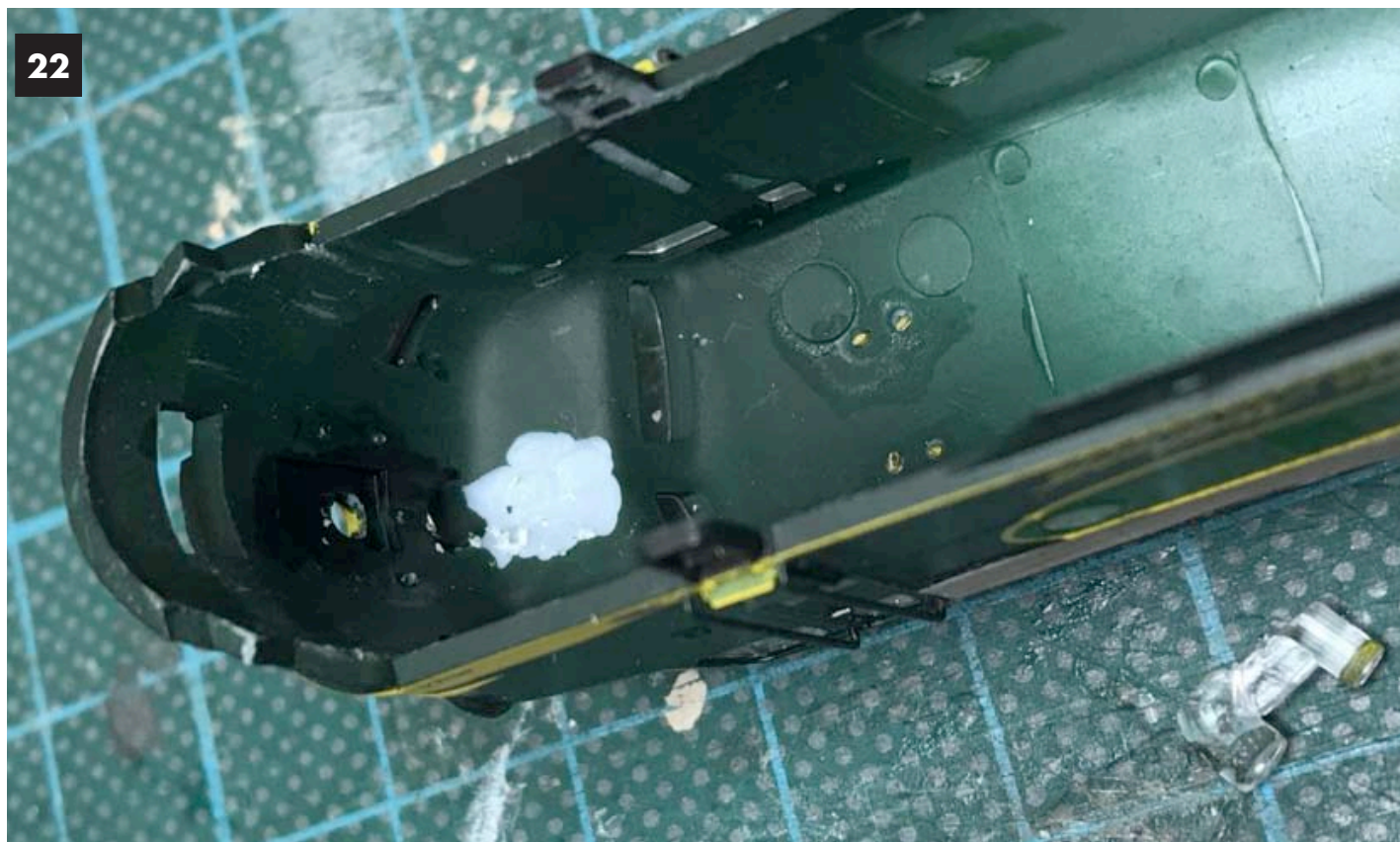
Image 22. To get the A-units to sit level after the LEDs are installed I had to remove a little bit material in the middle of the nose.
