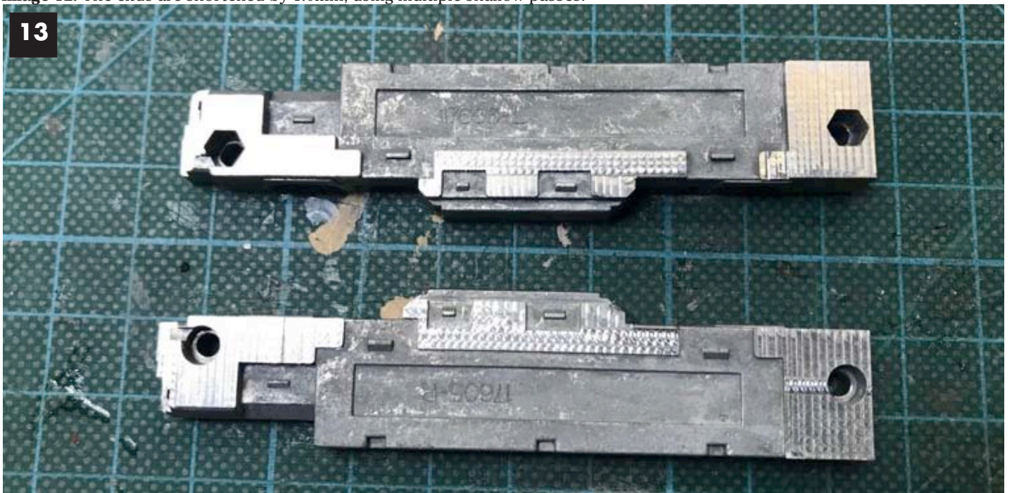
Image 13. Milled frame back on the workbench. Repeat 2 more times for an A-B-A unit. Once the mill is set up milling each frame half took me about 10 minutes, so it goes fairly quickly.
