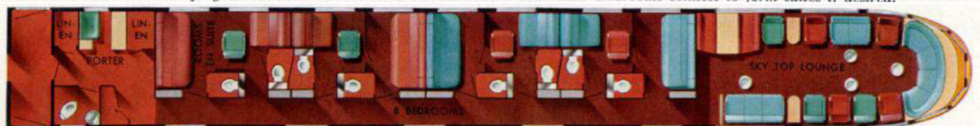
The Sky Top Lounge car includes eight double bedrooms, each with electric outlet, circulating ice water and individual air conditioning and lighting.
