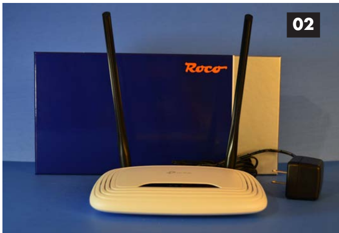
Image 02. The Z21 WLAN package is sold separately and it is designed to be a plug and play once the unlocking feature is implemented to any Z21 system.
