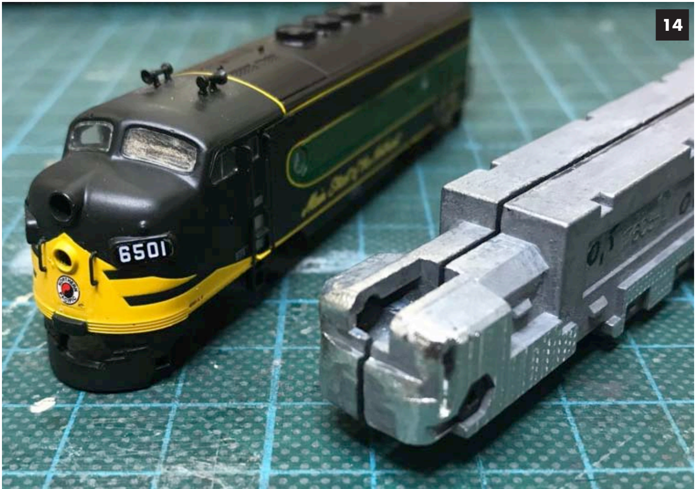
Image 14. The Intermountain unit have a slightly different nose contour, so use a jeweler's file to remove some material from the frame. Test-fit often to make sure that it will fit without a lot of pressure. The inside of the shell has a vertical raised strip behind the cab doors; I removed them for a better fit.
