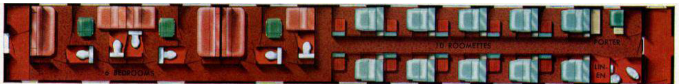
This all-room sleeping car contains ten roomettes and six double bedrooms. Bedrooms connect to form suites if desired.
