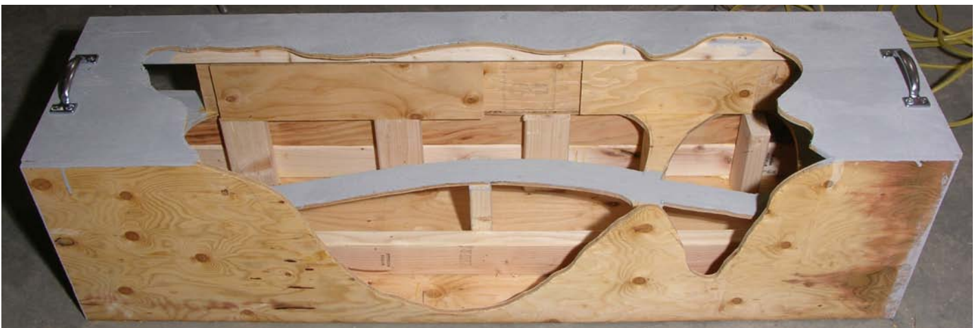
Above. Next I used scrap plywood to sheath the fascia and the top, I started conservatively because it is easier to cut material away than to add plywood. The goal is to disguise the caps. Notice the well-supported handles on the top. This will be heavy.
