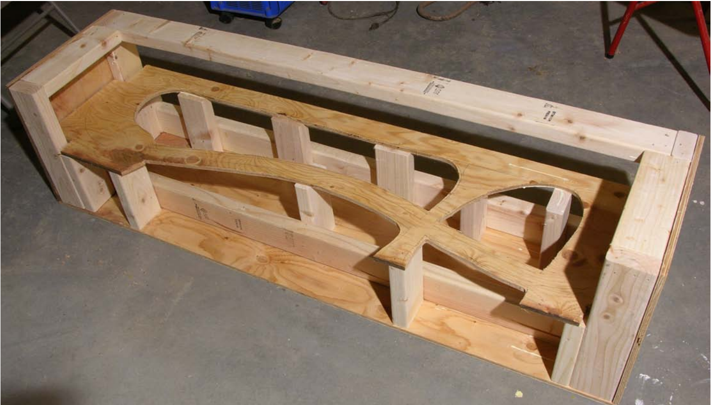
Above. I played with heights and decided a total of 16" with the track at 8" felt right. Then I built a box around it and cut 2x4s to support the sub-roadbed. This was the first time I used pneumatic tools and 4" wire nails with yellow glue. I really liked this.
