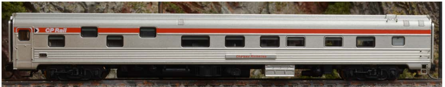
Above. Then first Chateau sleeper Richelieu. The Chateau sleeper had 8 Duplex Roomettes, 4 Sections, 3 Bedrooms, and 1 Drawing Room.
