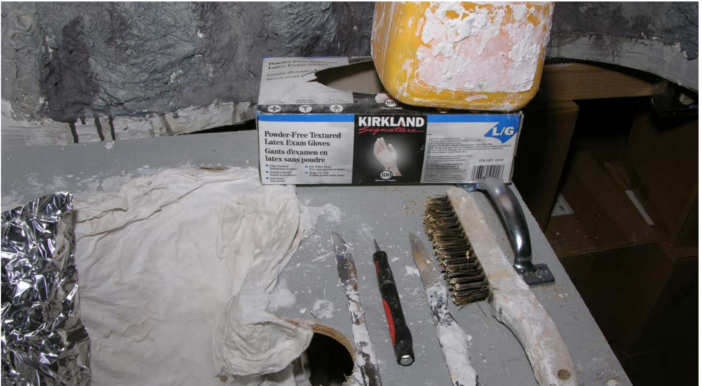
Above. The tools can be very simple: A kitchen knife, a cheap hobby blade, sometimes I use a paring knife, a steel brush, a spray bottle, latex gloves, and a flexible plastic mixing container make life easier.
