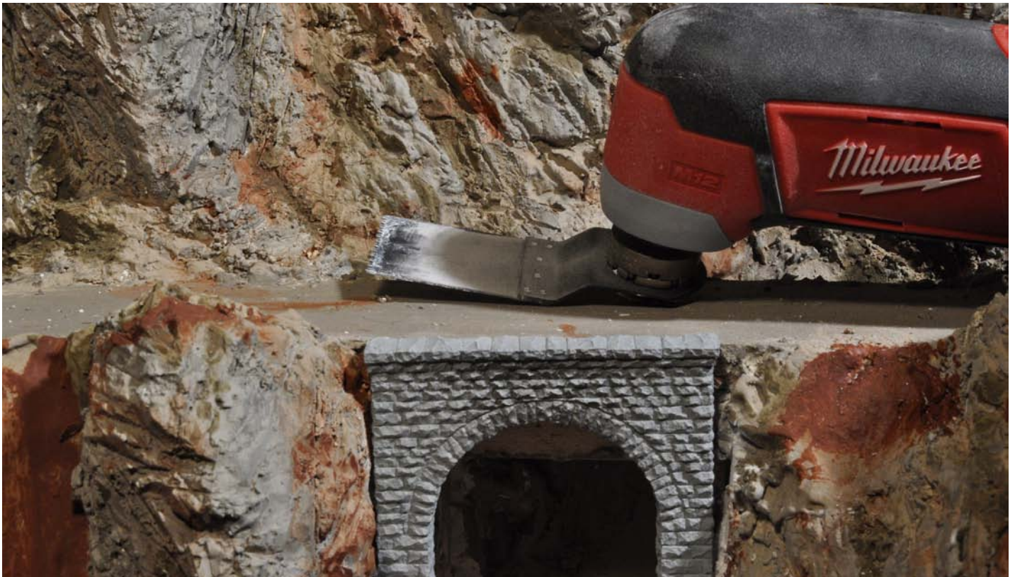
Above. At point we have to clean up our sloppiness. Hydrocal can dull chisels... but what can work even better is an Oscillating Multi-Tool. This works like a vibrating chisel. Practice elsewhere but one can cut through the Hydrocal to remove excess globs, insert culverts, etc. It can be easier to be moderately sloppy and fix than try to be tidy through the whole process.
