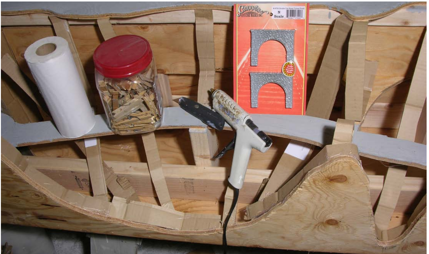
Above. Cut strips of cardboard (carefully!) using a sharp box cutter. The landforms are created by hot-gluing the strips together with clothespins to temporarily hold the pieces together until the glue cools. One of the problems with tight radius is the wide swing on curves. I decided to cheat and use a double portal and use scenery to hopefully hide this. While staring at the Chooch tunnel, I realized they would make great culvert facings for eastern or European right of ways, which were built before cement became common. And using them for culverts helped my time budget.
