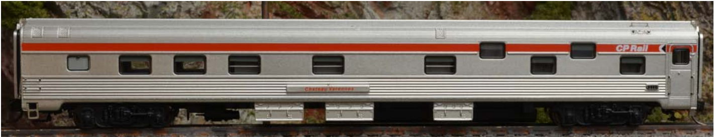
Above. The second Chateau sleeper is Chateau Varennes. Unlike most US sleepers, the expensive spaces are in the center of the car away from the trucks.
