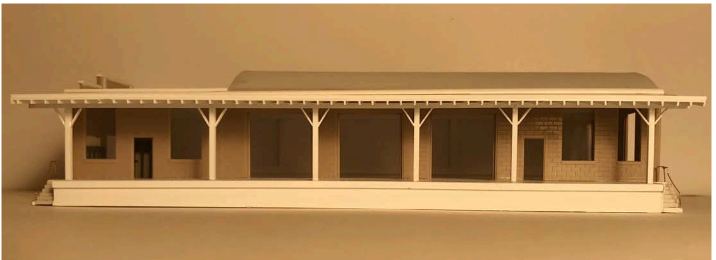
Image 06. The six posts are made from .060" x .060" styrene each at 11' feet long that holds up the rafter along the edge of the dock. Each ceiling joist is made of .020" x .040" styrene with a spacing of 5/32". Note that the posts are strategically placed in between door openings.
