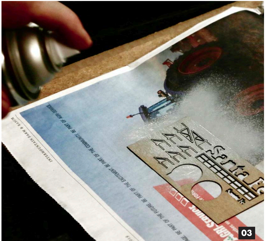
Image 03. Spray the cut pieces to add some strength to the parts.
