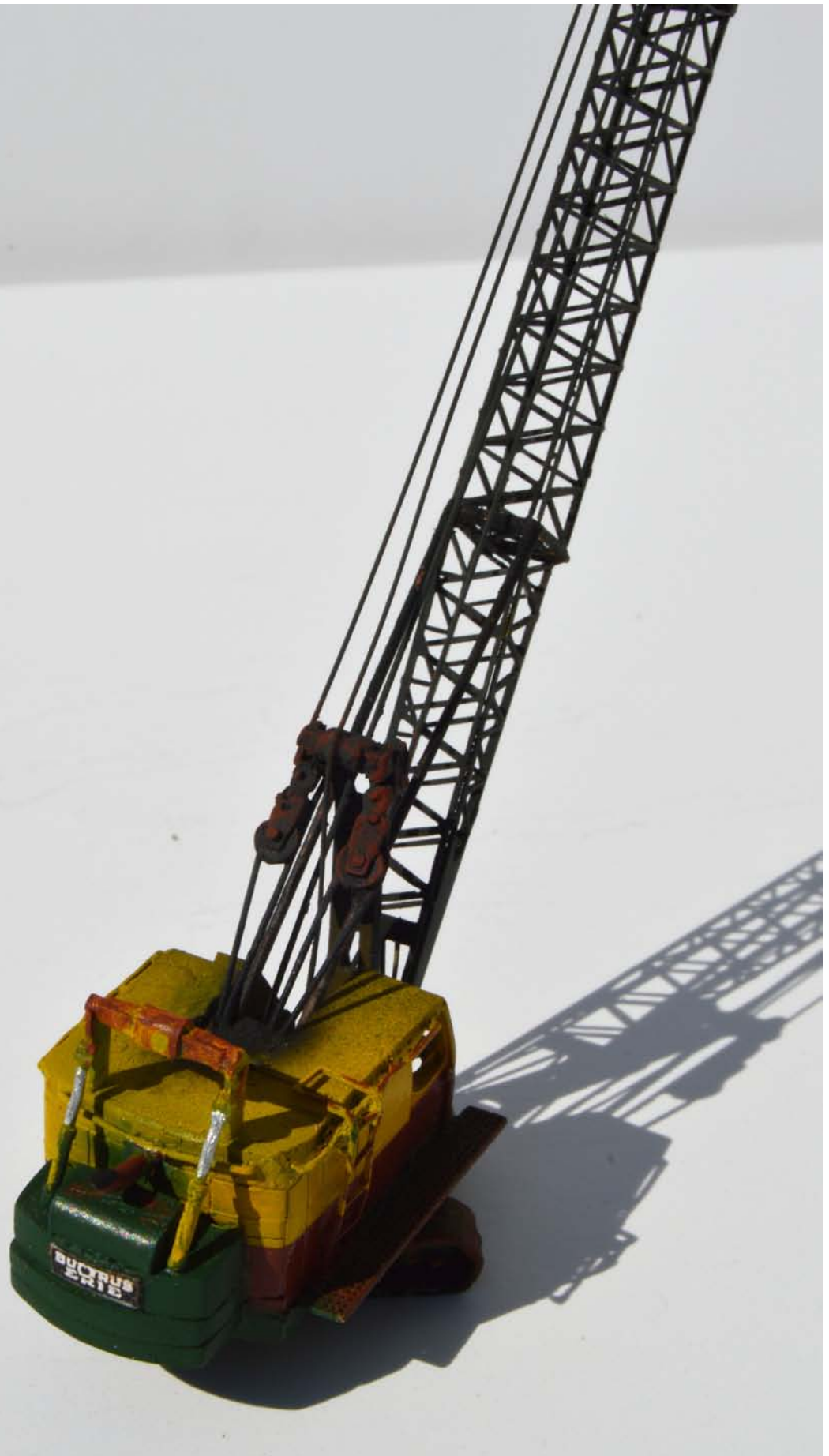
15. The author added extra counterweights and other attachments seen on larger construction cranes for heavy-duty service.
