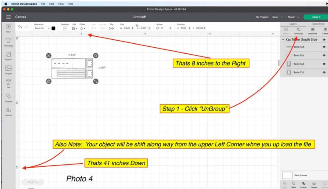
**Image 04.** A screen shot of Cricut Design Space. As the SVG File is up-loaded everything becomes grouped into one object. Note the overall length is 0.645 inches which is too short. The objects will also be a long way from the upper left corner of the Design Space.
