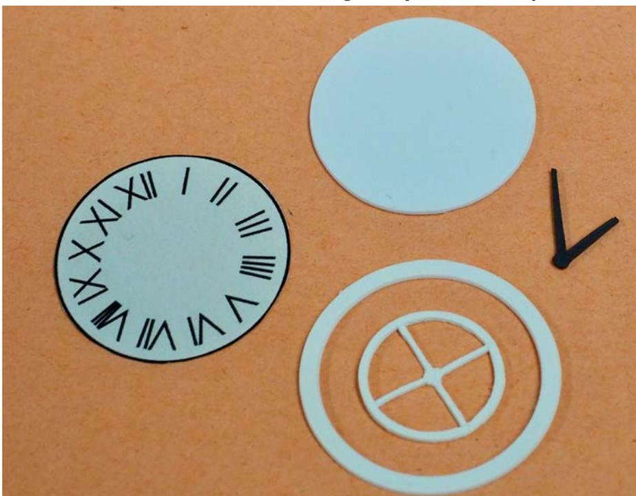
**Image 42.** The clock face was printed on paper while the hands and rings were cut with the Cricut Maker. The Maker is exceptionally good at cutting circle components out of styrene.
