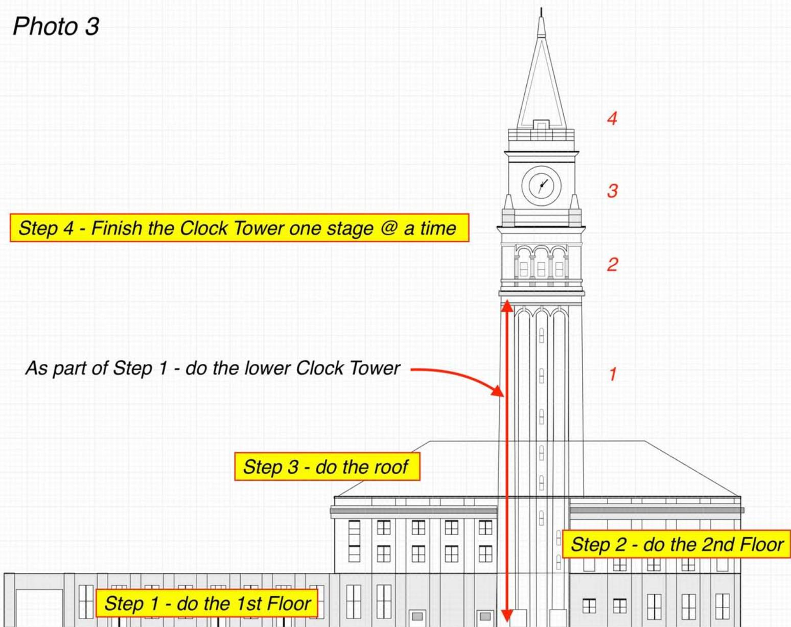
Image 03. One my early illustrator drawings of King Street Station with my basic plan of how I would break down the construction into sections of work.
