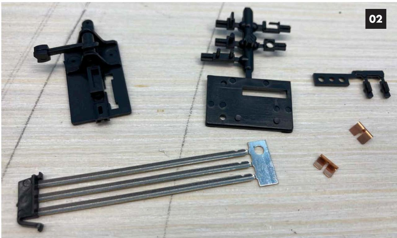
**Image 02.** These are all the goodies in the Caboose Industries package, many of which are not needed.
