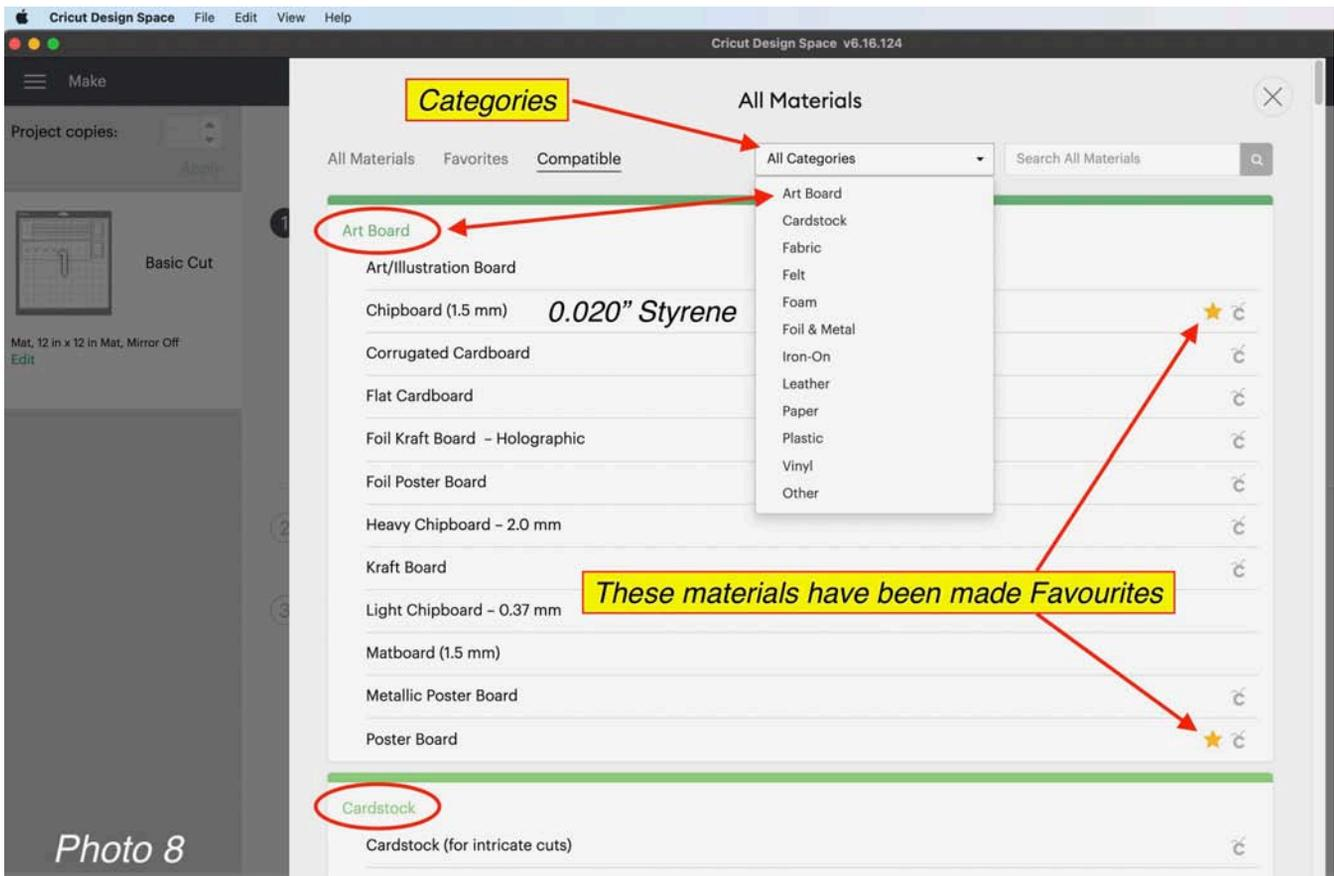
**Image 08.** Pick the type of material that you're going to cut. By marking you're commonly used materials as a Favorite, you will see them as a clickable selection (Star) and reducing the need to scroll through a long list, as shown in the photo.
