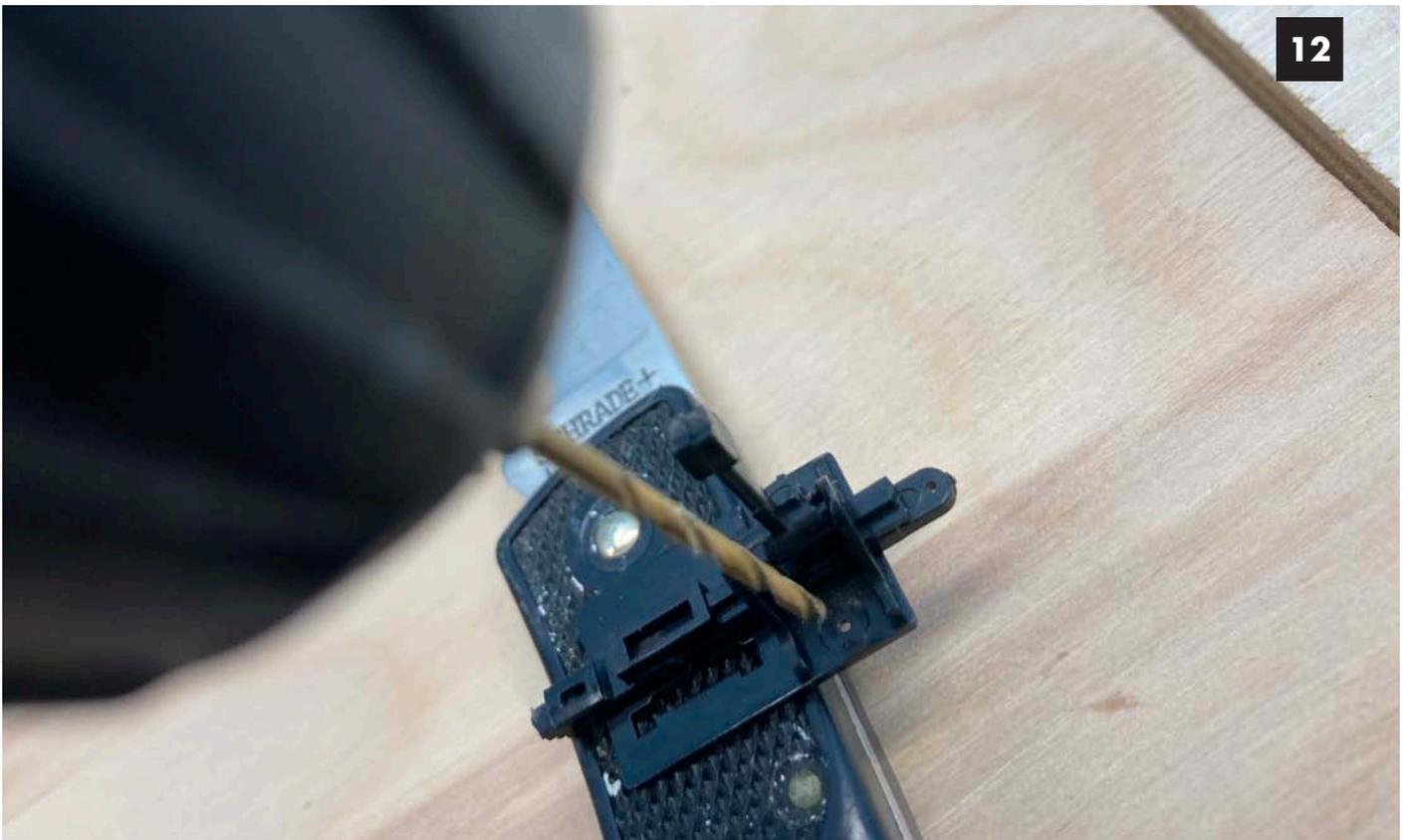
**Image 12.** I use #2 5/8" wood screws to secure the ground throw in place. The holes in the ground throw need to be enlarged for these screws to fit. I again use the #51 drill for this job.
