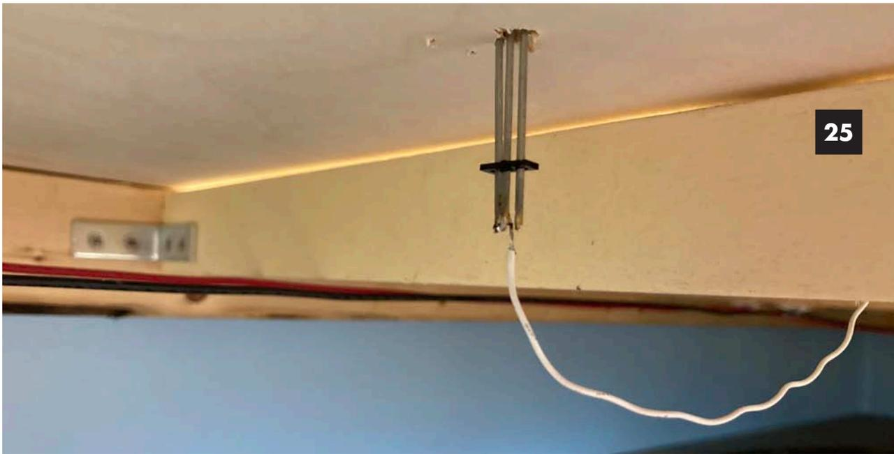
**Image 25.** The wire from the lug for the frog is soldered to the middle post of the wiring connector.
