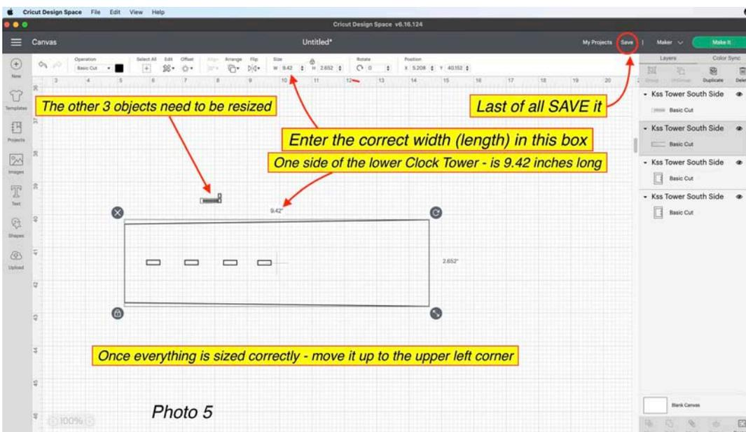
**Image 05.** In Affinity Designer you can see the length & width of an object that you select. I generally only write down the length as I've found that if I enter the length of an object in Cricut Design Space the width was always correct as they are proportional. One wall of the clock tower has been given the correct length (width), the other 3 objects still need to be done..
