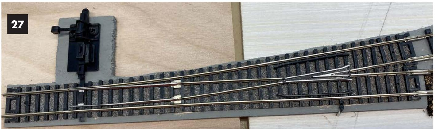
**Image 27.** The final touch is to hide the mounting screws, dull down the frog casting and disguise the frog wiring lug. I found that Tamiya XF-84 Dark Iron, is excellent for this application.
