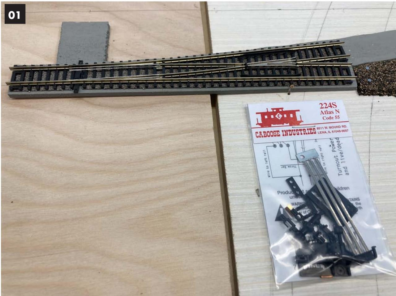
**Image 01.** Here is a pre-ballasted turnout (see NSRR Issue 117 Jan/Feb 2020) and a ground throw ready for installation. I prefer to lay my turnouts on 1/8" basswood.
