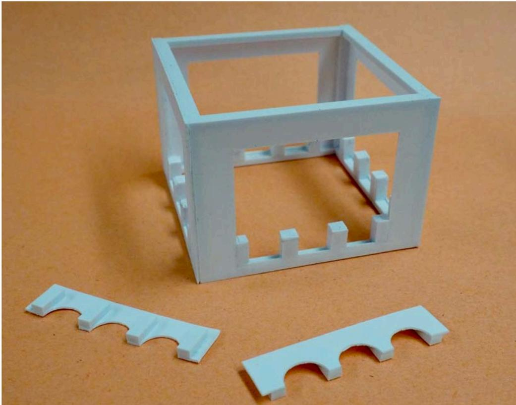
**Image 35.** The 2nd section of the clock tower. The walls were cut by the Cricut Maker along with Evergreen strips for bracing.
