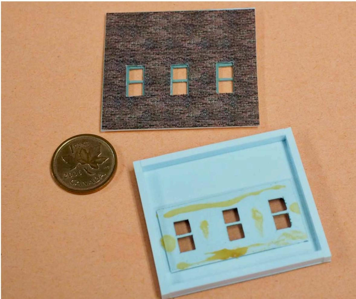
**Image 39.** The 2nd section of the clock tower has an enclosed space inside of the columns. I made the required windows by cutting a separate window piece to go inside the outer walls. As I went up the clock tower I cut what I needed on the Cricut Maker. I had lots of partially cut Evergreen styrene sheets that I could use for these small detail parts.
