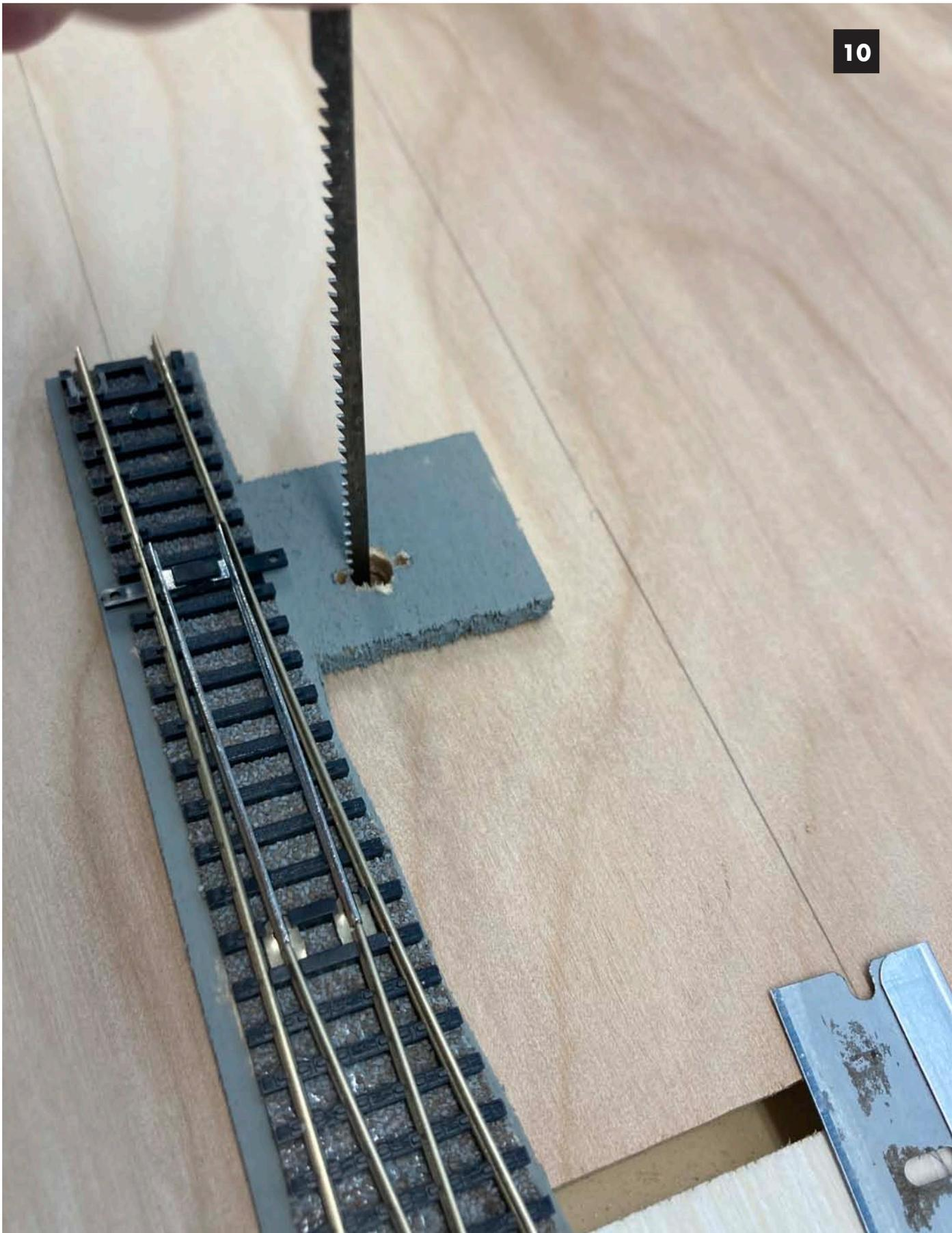
**Image 10.** I use a naked coping saw blade to carefully enlarge the hole into a slot for the wiring connector. This is truly easier than it looks and sounds. My benchwork here is 1/2" Baltic birch plywood, if it were a thicker base, it would be a little more tedious.
