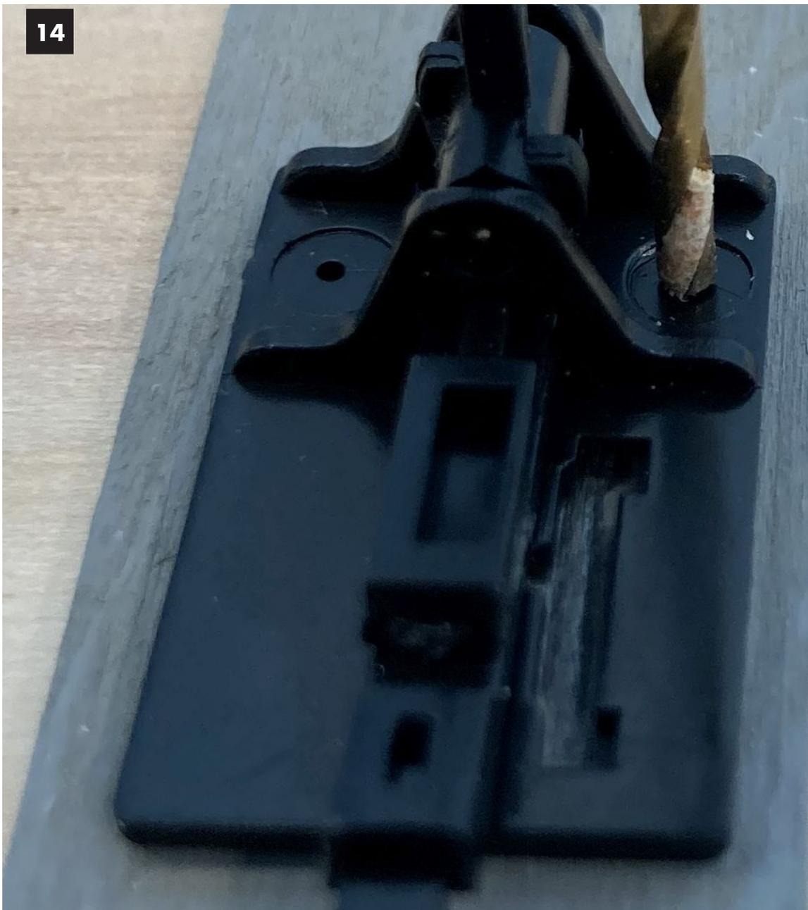
**Image 14.** Position the ground throw the same way as in Image 6 and drill the screw hole through the switch block and the benchwork. I drill one hole, insert the first screw most of the way and then fine tune the alignment. Then I drill the second hole and insert the second screw.
