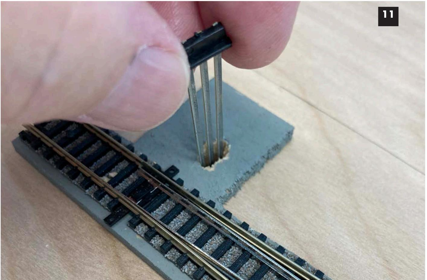
**Image 11.** Test fit the wiring connector and keep sawing until it fits.
