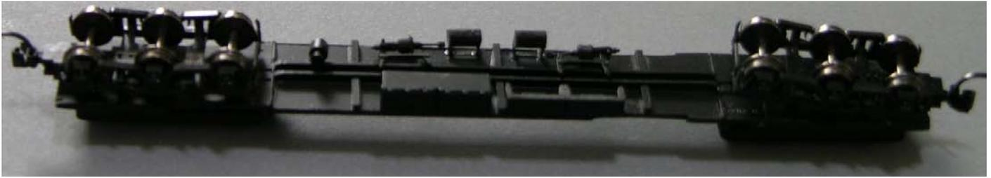
The underbody of the Wheels of Time kit has a low center-beam with cross members typical of "Harriman" style cars, but the holes for truck bolster pins are spaced for the off-center design used on old Micro-Trains 6-wheel trucks with 33" wheels, which are not prototypical for these T&NO cars. The battery box is inset too far from the inner edge of the car's side as well. Rather than making corrections to the resin-cast floor, I opted to construct a replacement floor using the bolster ends
