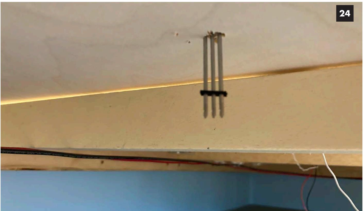
Image 24. Underneath the benchwork to see that the three-hole spacer is placed on the wiring connector.
