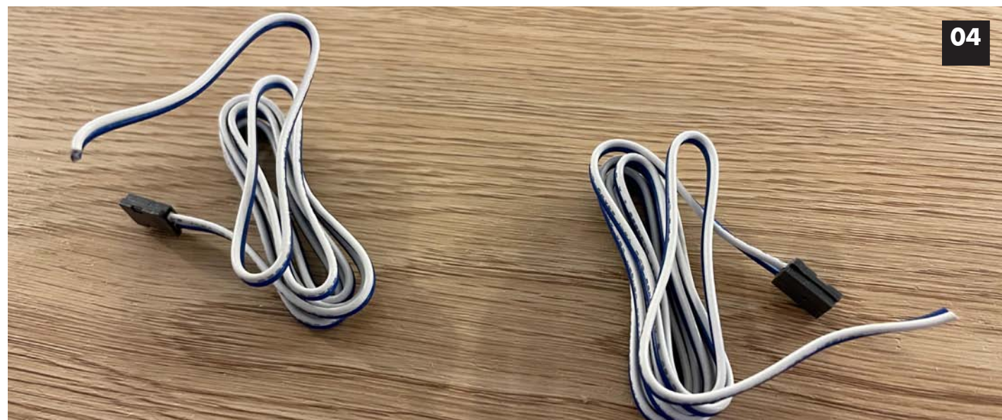
Image 04. Kato Unitrack is normally the easiest to set up. However I want to use multiple types of throttles so I clipped the plugs so I could use Euro connectors.
