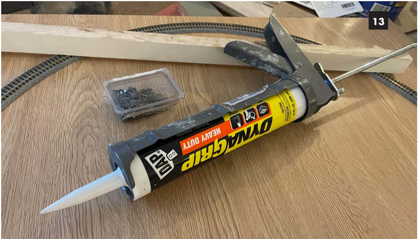
Image 13. Bill cut the door down to 60", which leaves an open end. Bill cut down a scrap wood. Bill used DynaGrip to glue the wood to close the end. Bill used a pair of small nails to close the open end.
