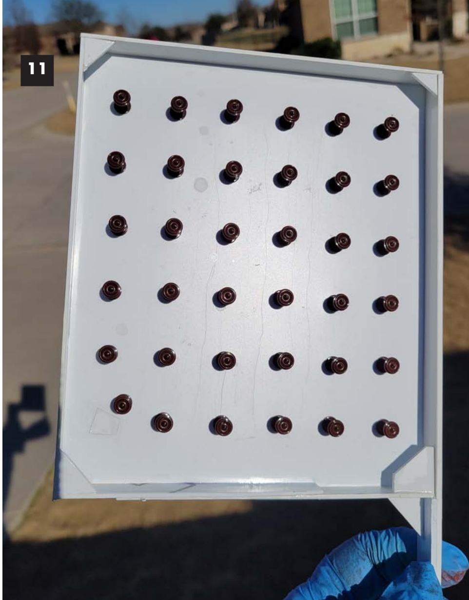
Image 12. Pop the axles out and turn them around so the other side can be painted. You can see the top three rows have been turned while the bottom three have not been turned yet.
