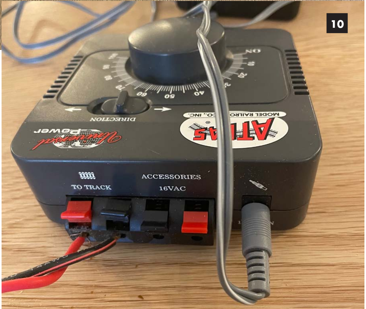
Image 10. I couldn't find my good wire strippers, lugs, and crimp tool... I used this Atlas throttle that used these push/clip system. The wires are stranded and I soldered the ends so they are now solid.
