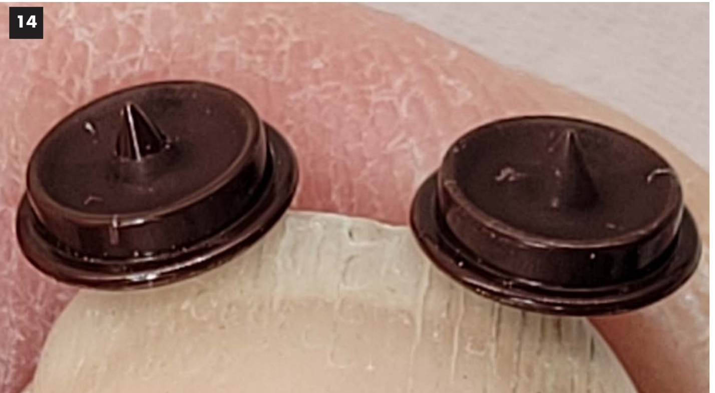
Image 14. I use a cloth to wipe the tread and axle point to be sure both are clean. You can see the cleaned axle point on the left wheel.
