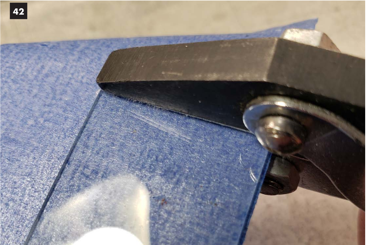
Image 42. With a pair of parallel jaw pliers grab the glass at the score and twist the pliers to snap the glass. This usually renders a straight break and no glass slivers.
