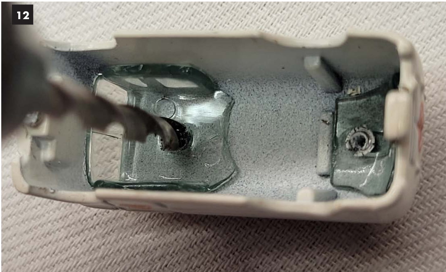
Image 12. If you're planning to paint or flat finish the body drill out the head of the rivet for both pieces of glass. Be careful to
