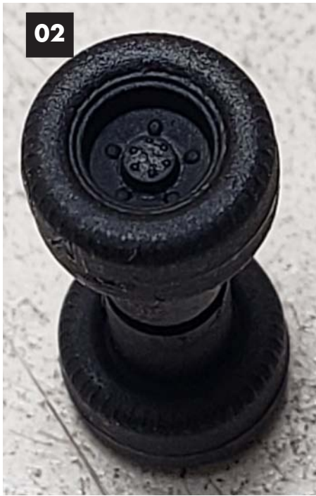
Image 02. For this project the wheels will only be viewed from the side. So that opened up the choices available. The wheels on the short Atlas trailers that come attached to some of their flat cats have nice detail when viewed from the side of the wheel. When viewed from the tread side they look like a single tire that is double width. The axle is huge also. That view won't be visible for this project so they were a perfect choice. To get rid of the shine I painted them flat black.
