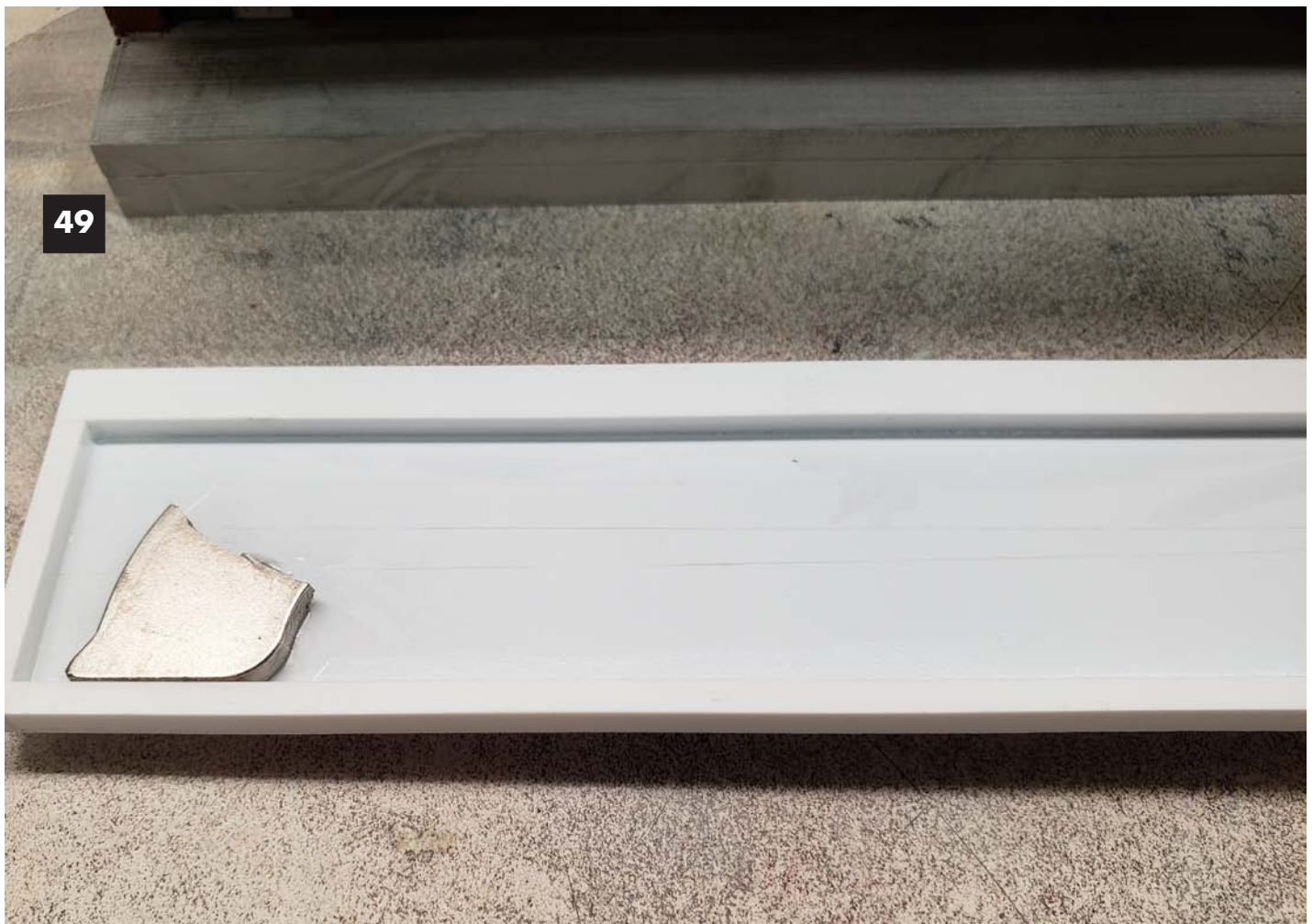
Image 49. On the underside of the parking area I added a magnet at each end. This will be used to pull the parking area snug against the foundation of the dock. As I recall it was just .040"
