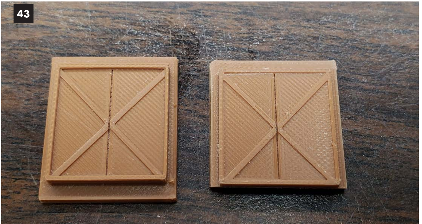
Image 43. Here we see the doors that are now separate pieces. On the left is how they come. The problem is if you installed a floor you have to trim off the flange as shown on the right. An-
