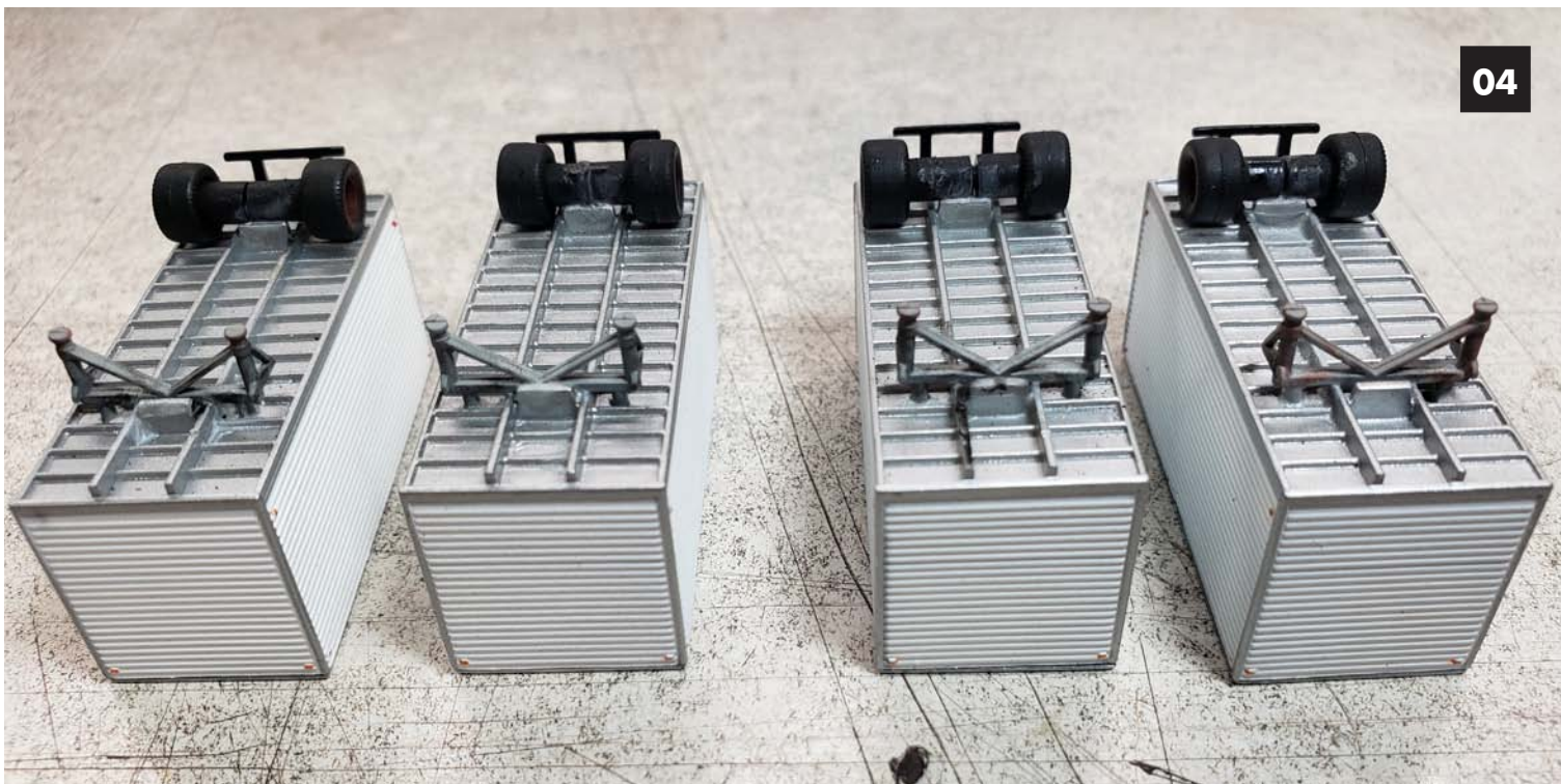
Image 04. The wheels are then glued right to the underside of the trailer.
