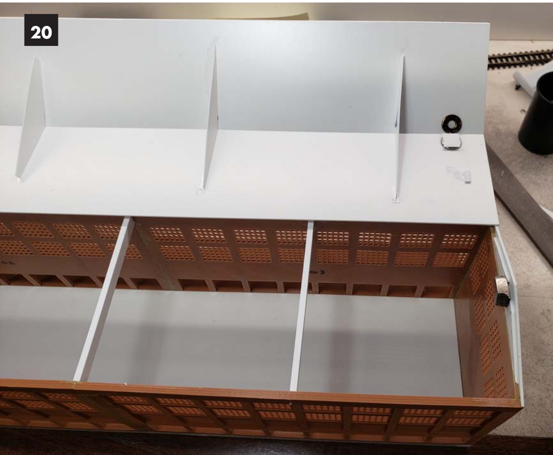
Image 19. Using the same 135 degree angle as the gables I cut several trusses or ribs to give the roof some structure and rigidity. Then glued them on spaced evenly. Some were a little
