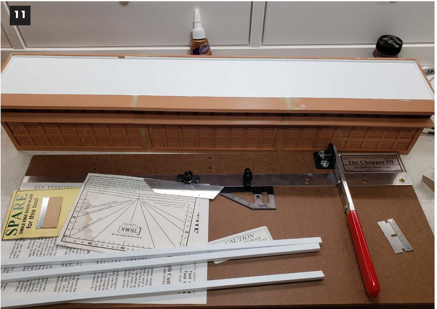
Image 11. .250" strips of styrene were glued to underside of the floor against the wall. This gave a better gluing surface to weld the floor to the walls.
