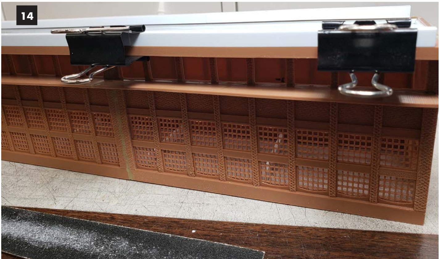
Image 14. Spring clips do a good job holding the styrene strips while gluing. I made a point to avoid seams in walls coinciding with seams in the styrene strips.
