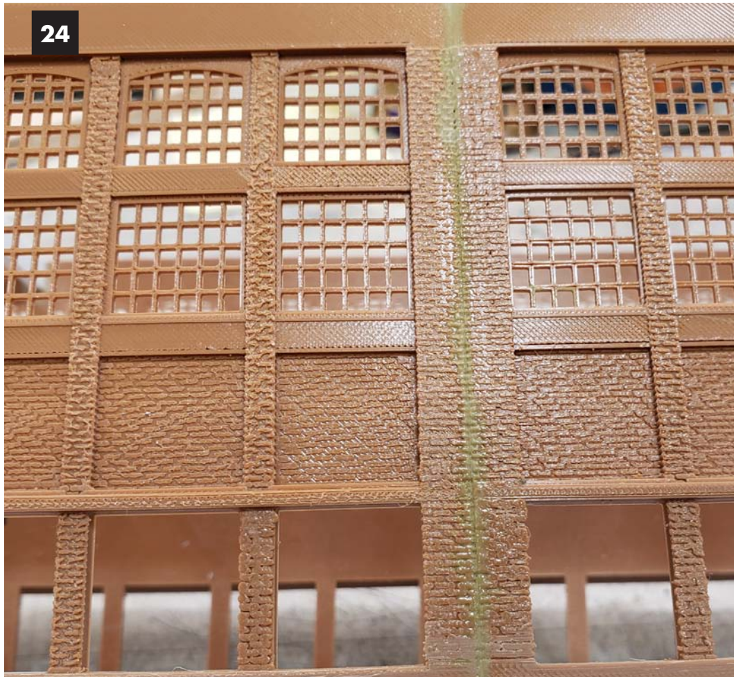
Image 24. This is a view of one of the seams between wall sections. You can see the brick pattern doesn't flow from one wall to the other cleanly. Plus there is more of shine where the solvent rounded off the pattern. BTW when you really look closely it doesn't look like brick at all. But when you back off a few inches it does look like brick.
