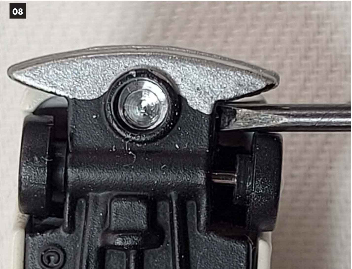
Image 08. Using a small flat blade screwdriver attempt to pry the floor off the body. If it doesn't come easily drill a little more till it does come off easy.
