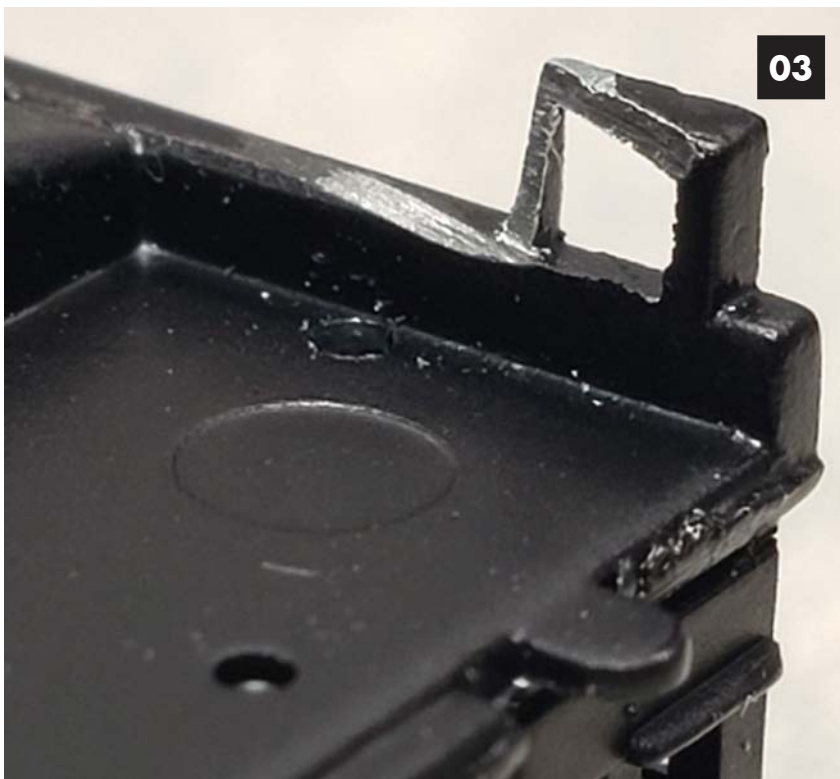
Image 03. I used a small file to thin the stirrups. These file down fairly easily. From the front side it still looks unaltered. I did 32 stirrups with no breakage. I do not recommend using a motor tool due to the concern it's easy to grind away too much before you know it.
