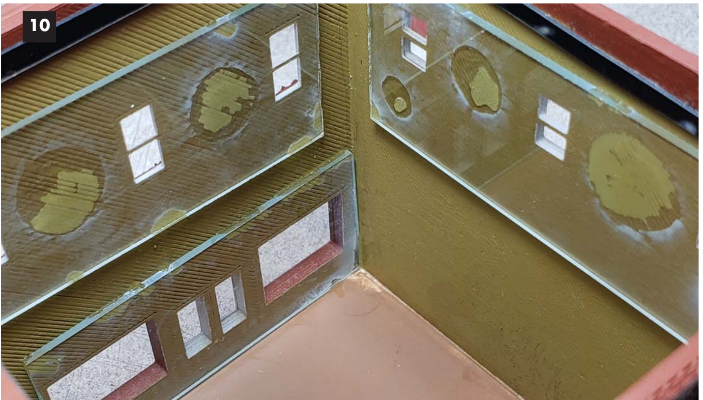
Image 10. I like real glass for windows. Using slide glass is an easy and inexpensive way to cover several windows at a time. I just put dot of CA between the windows to hold it in place.
