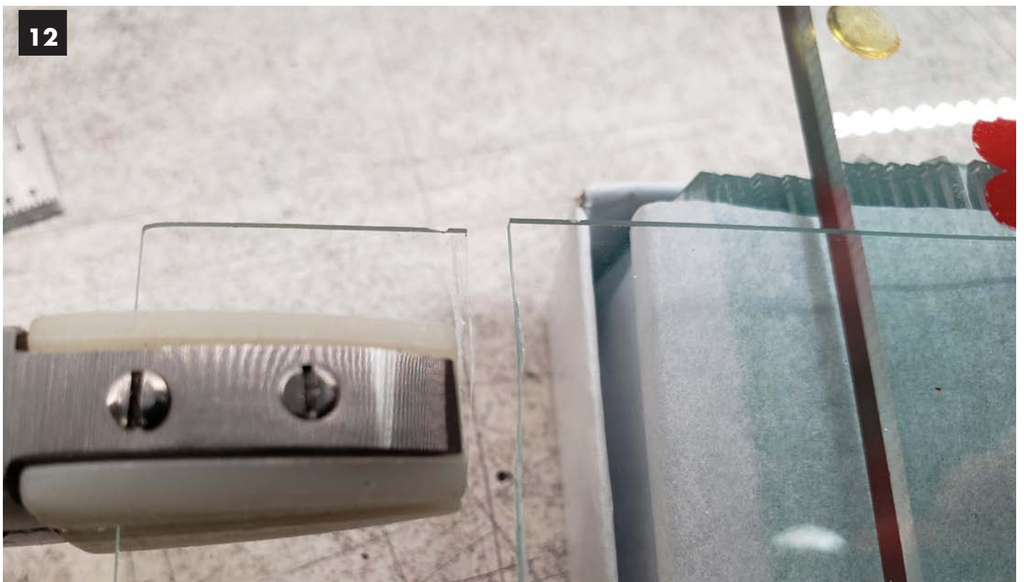
Image 12. Use plastic jaw pliers to snap the slide at the scored line.
