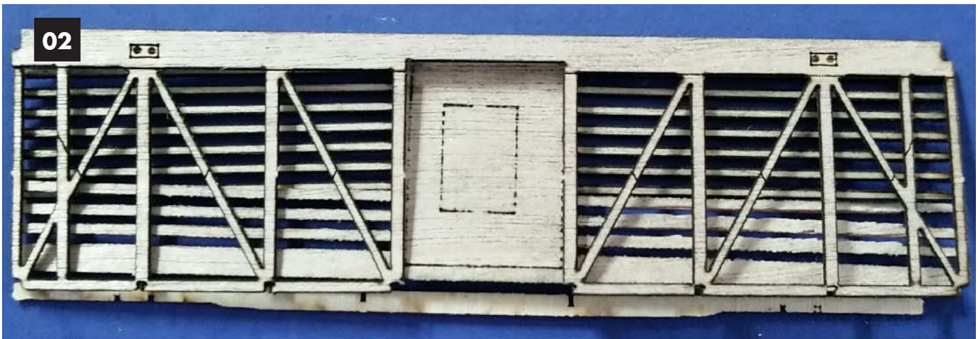
Image 02: Rotated stock car side. The RSLaserkit sides have 6-foot wide stock loading doors of a design that is quite different from those on Southern Pacific's stock cars, including the S-40-2s and S-40-3s. I figured that I'd just have to use them "as is" and installed them on one of the
