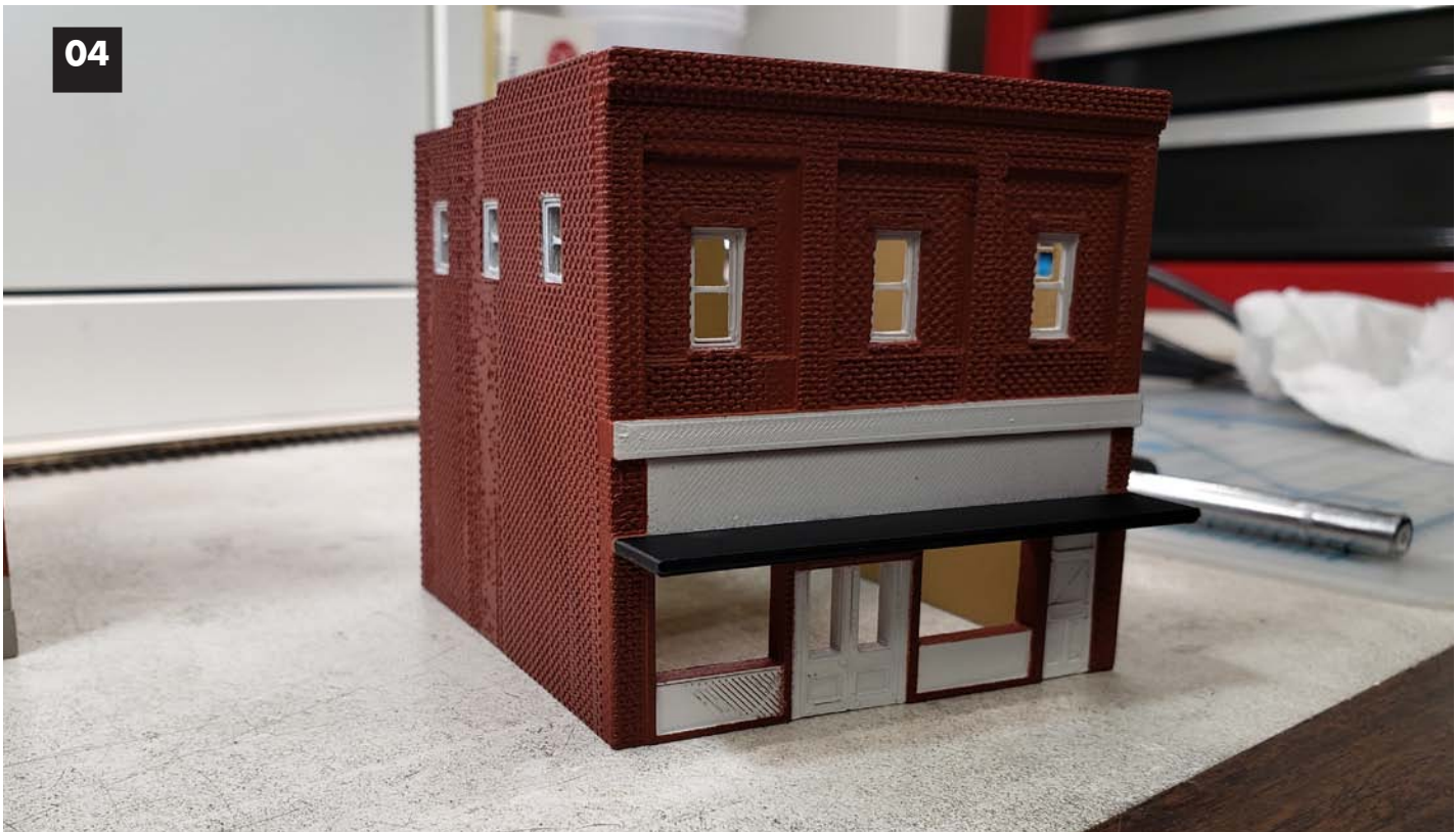
Image 04. After all the masking the building was sprayed with a brick color. Then the masking was removed, rendering a pretty good looking building. The brick pattern flaw on the left
