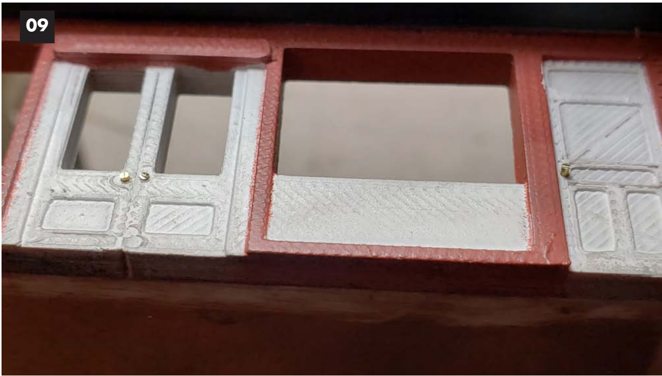
Image 09. Shove the brass rod in the hole and cut off with flush cutters. While it doesn't look like a door knob this close. When you get 12" away you can tell there is a brass door knob. This is a very easy detail to put on most any building.
