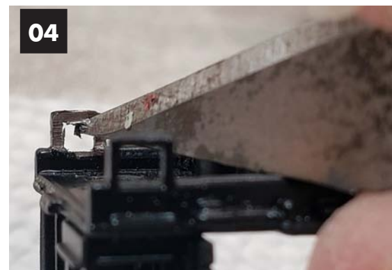
Image 04. Use a hobby knife to clean up the flash from the filing process. It comes off fairly easy.
