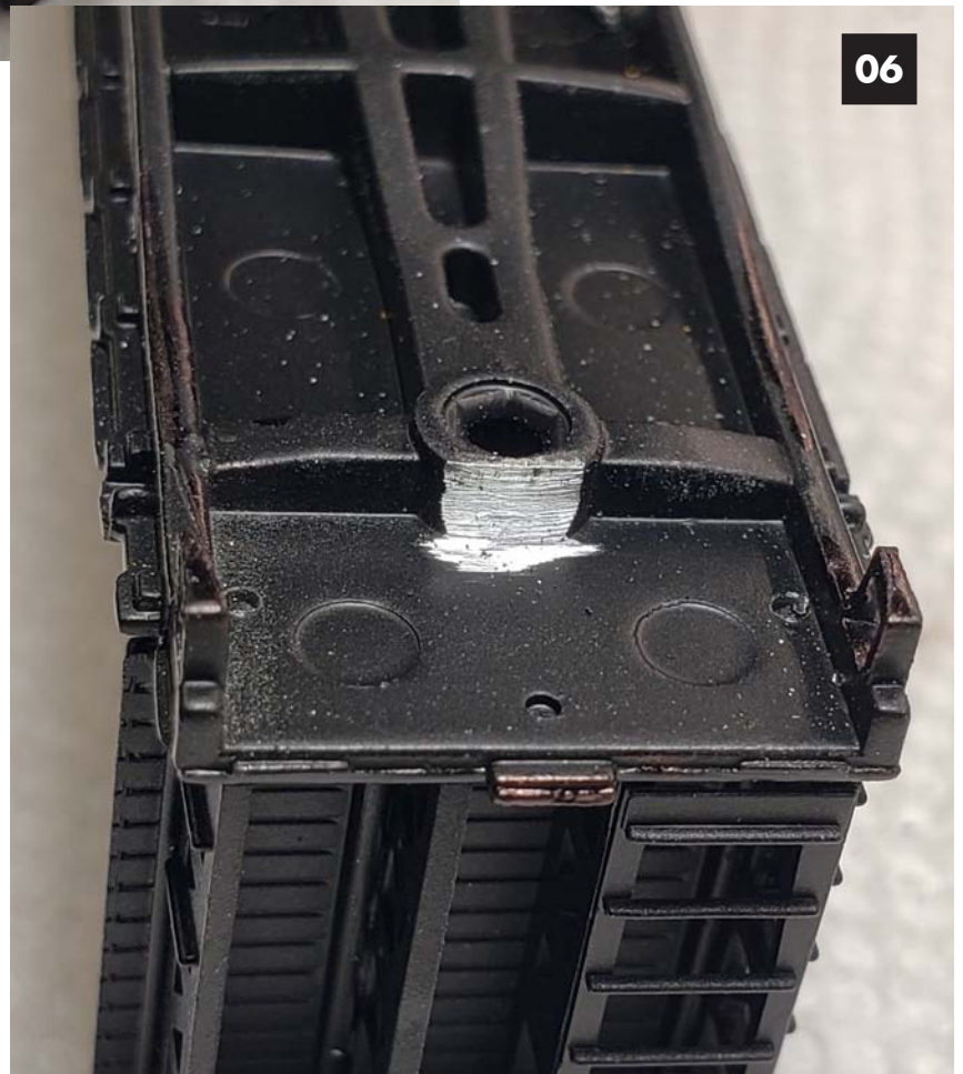
Image 06. After putting the Micro Trains trucks back on I was still experiencing derailments going through turnouts. At first glance the trucks were now swiveling OK. But as I rotated them I noticed the coupler moving. The problem was the back end of the coupler was rubbing against the bolster. In image 2 you can see the hole for the bolster is offset towards the center of the car. Thus making the bolster thicker on the coupler side than most bolsters. So the solution is to grind away some of the bolster to prevent the back of the coupler from touching the bolster. I highly recommend using a motor tool for this task.
