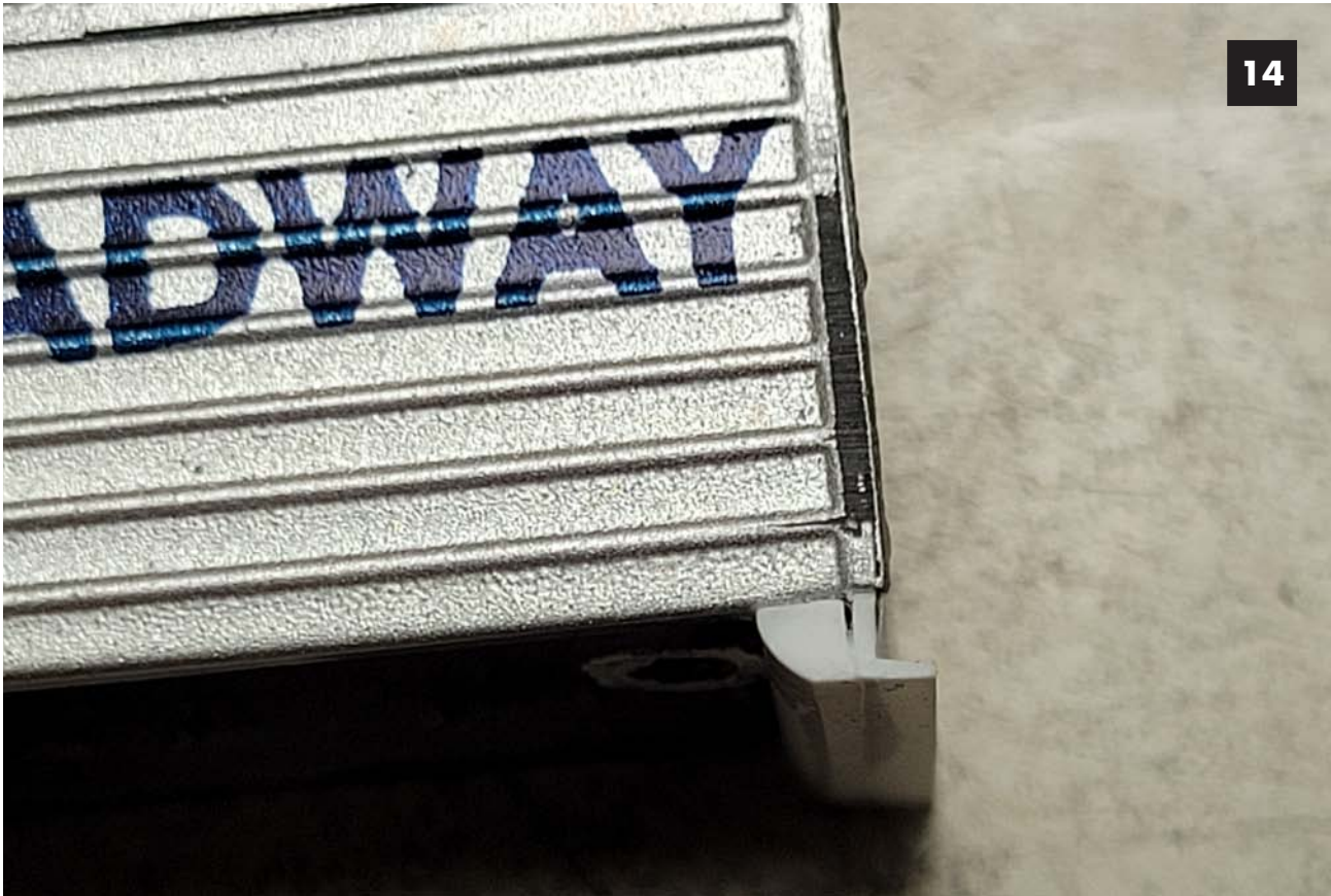
Image 14. After the solvent dries file the bottom of the step so the quarter round is even with the angle.
