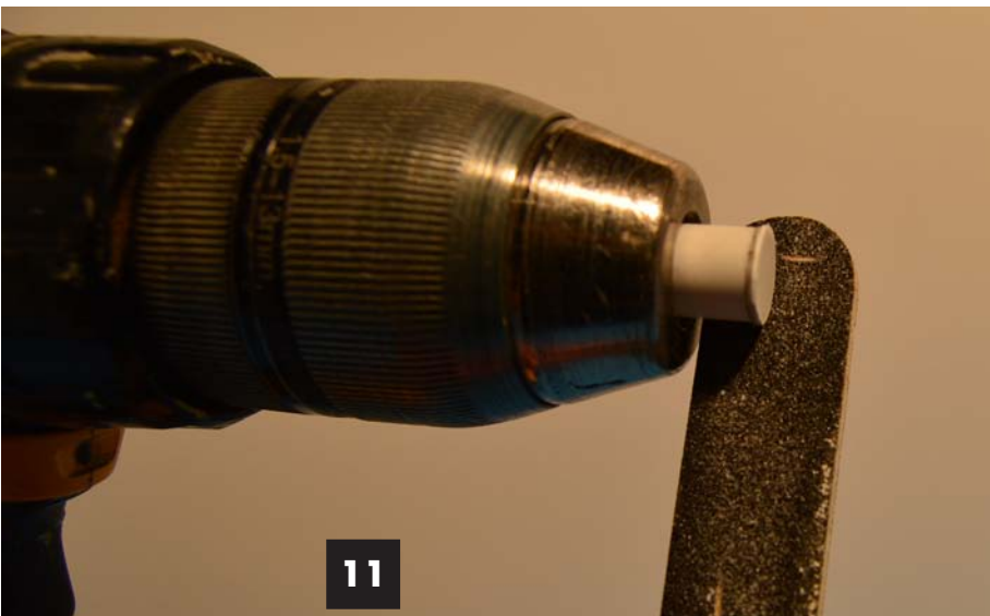
Image 10. Glue a piece of .020 styrene to each end of the silo and file down the cap to the contour of the tube.
