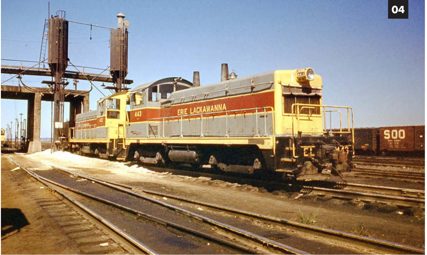
Image 04. (Croxtan Yard Secaucus, NJ Nov. 1979 Mike Pagano Collection) With all the road units now serviced, the yard switchers can finally start preparing the servicing tasks by first taking in some sand and then passing under the coal tower foundation to receive fuel for the day's work. Adding a pile of sand around the base of the sand towers is an easy detail to add.
