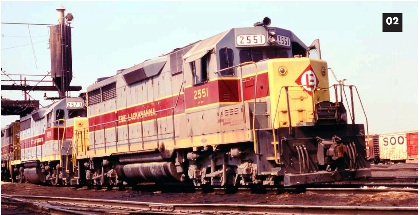
Image 02 (Croxtan Yard Secaucus, NJ April 1976 by Bob Yanosey) Erie Lackawanna GP-35s line up under the sand tower before starting their day heading out west of the Croxtan yard. Notice the weathering on the top of the silo vent cap.
