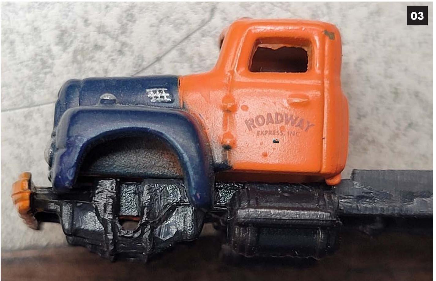
Image 03. This is before elongating the hole for the axle to allow the wheel to rise in the wheel well.
