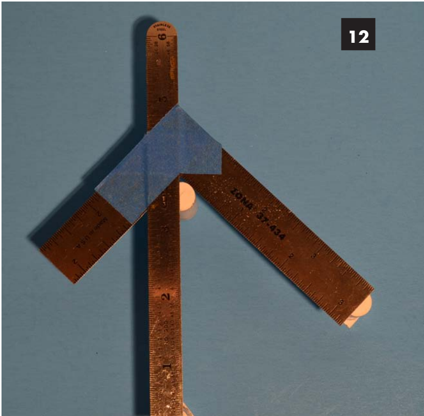
Image 12. Temporarily mounting a straight edge at 45° in between a square will make a great tool to find a center of a circle.
