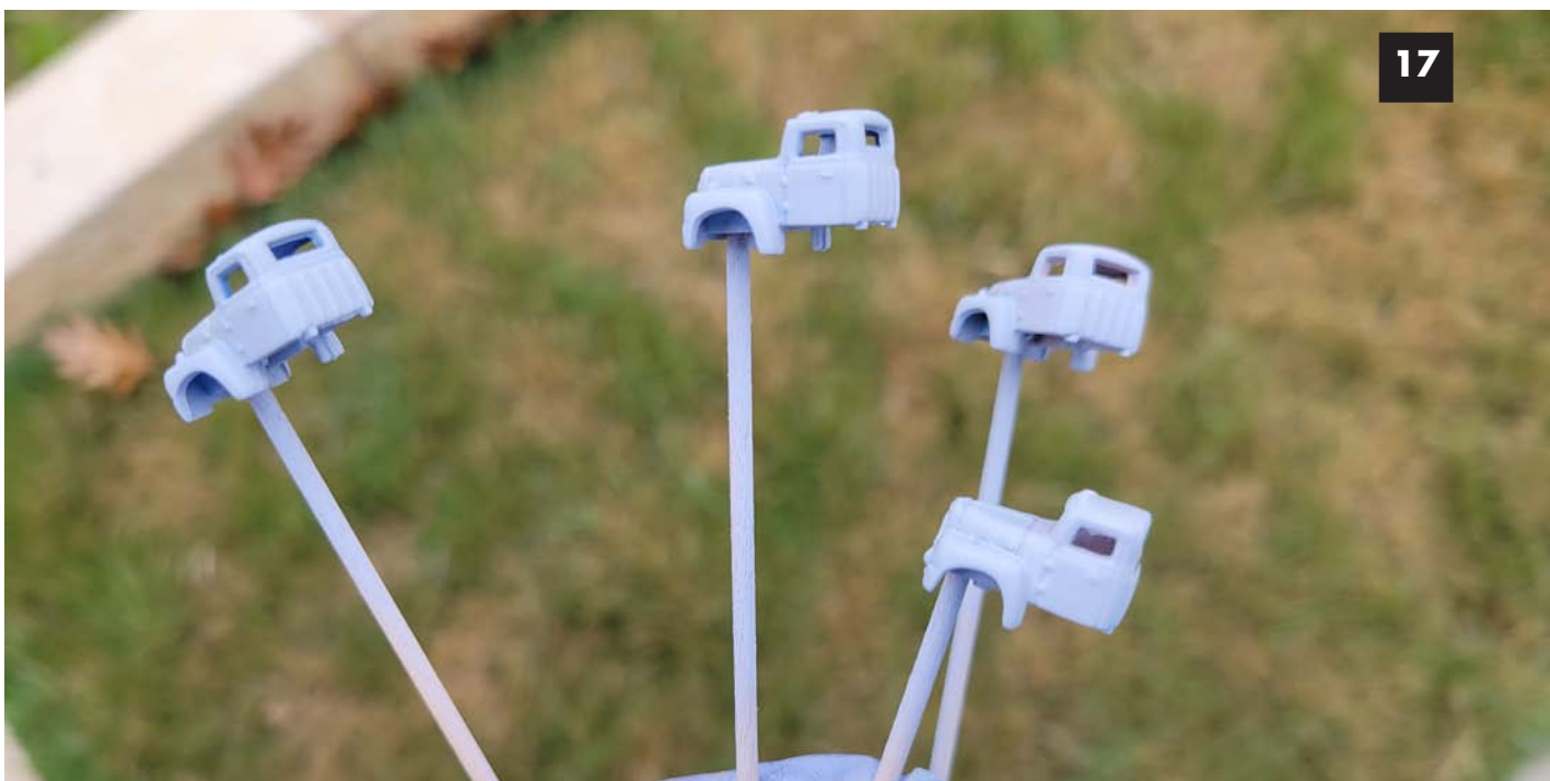
Image 17. I find it easy to just step outside with Tamiya Fine Gray Primer and give the cabs a quick coat to provide an even surface for the final colors. Wearing a glove is a good idea if you don't want your nails to be primer gray for a few days.
