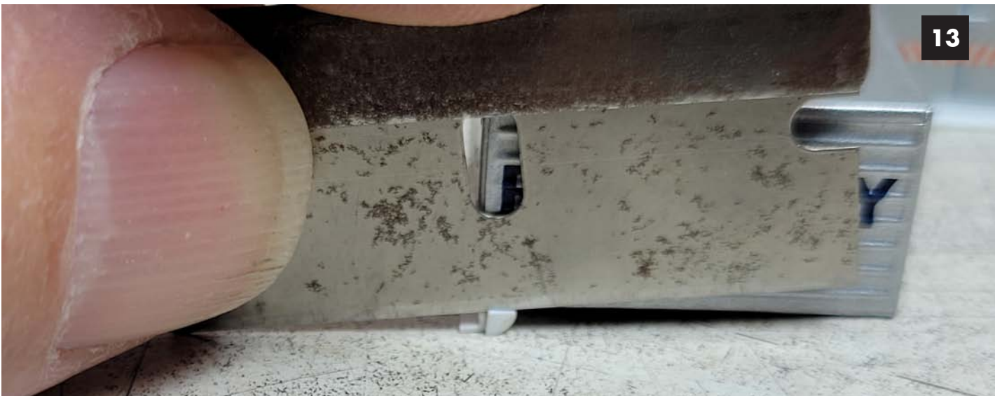
Image 13. Rather than try to cut the angle and quarter round the right size it's easier to make them a little longer then trim flush with the side after the glue sets.
