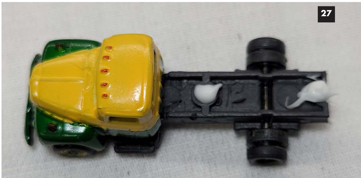
Image 27. Put a dab of Aleene's glue on the bolsters to hold the box on. Also put glue on the post to secure the cab to the chassis.
