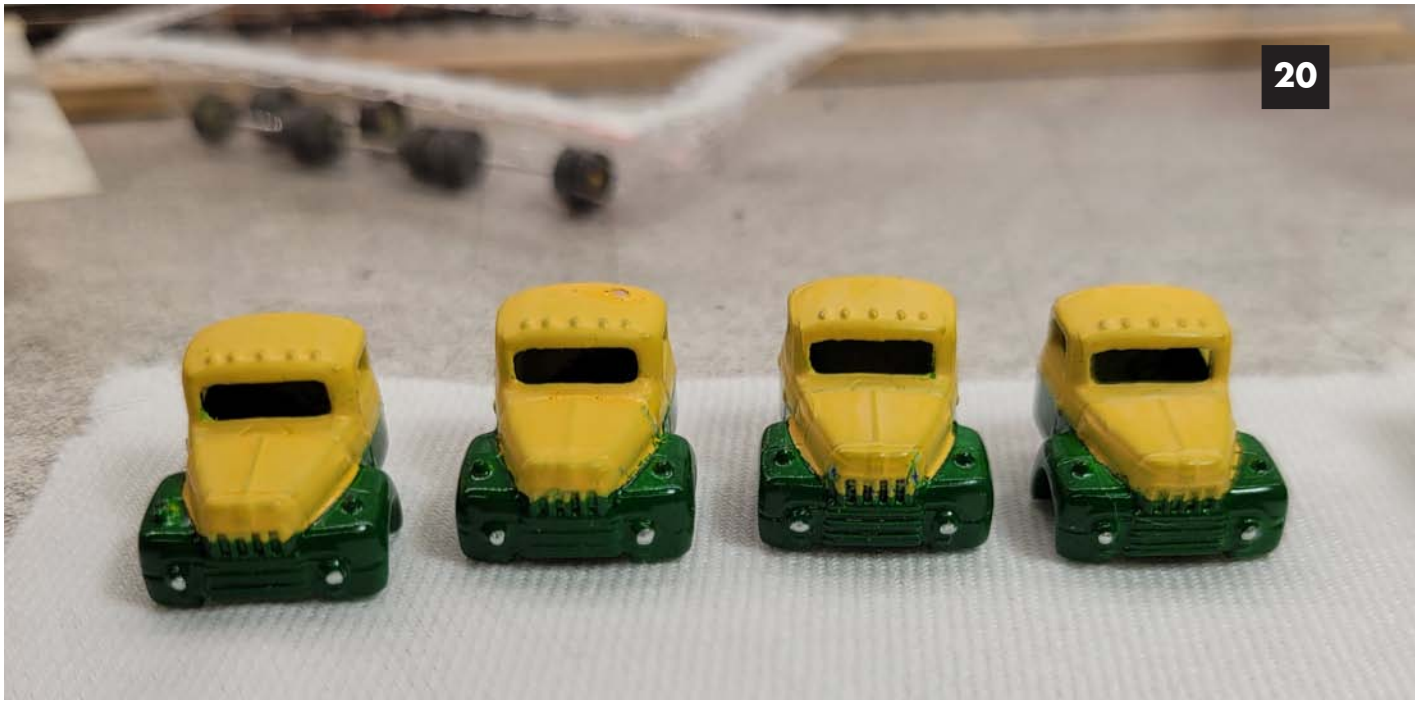
Image 20. I used the wrong masking tape and it shows. The mask lines allowed some green to seep under. I put a spot of silver where the headlights are to make them stand out.
