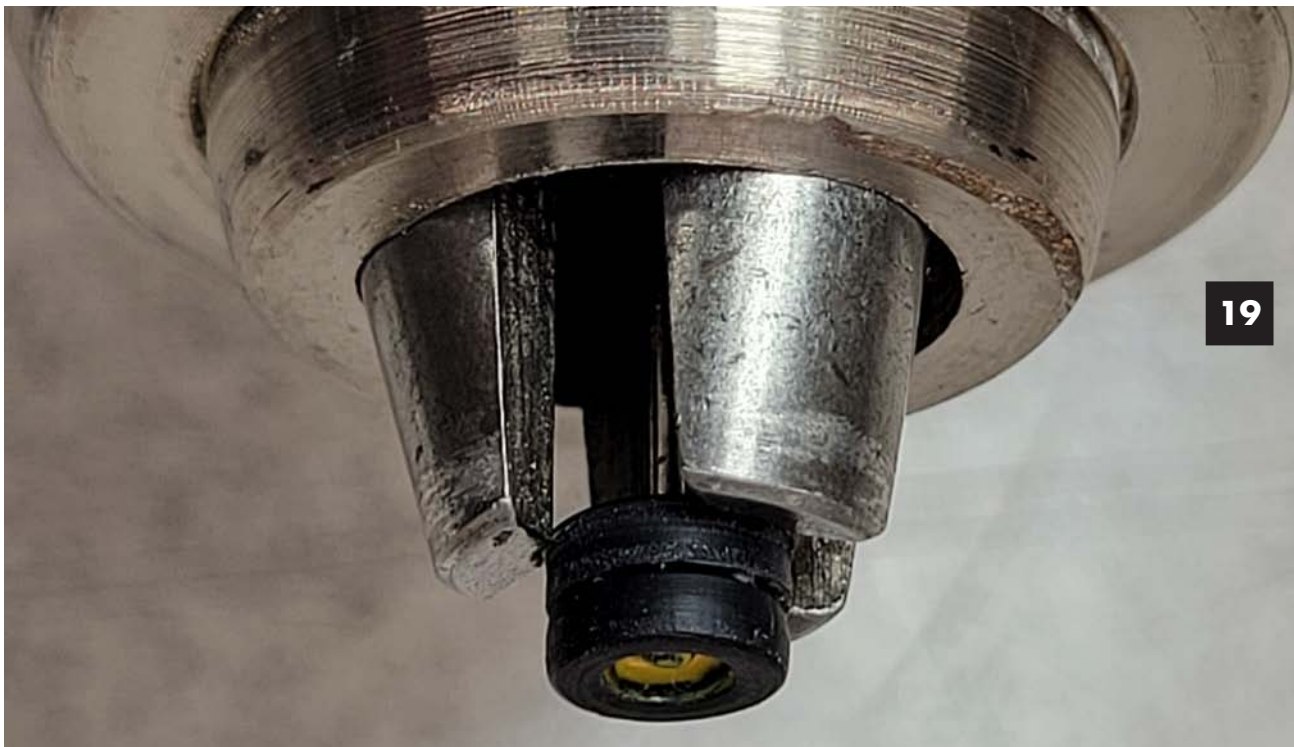
Image 19. I also shot the wheel yellow to try and get the rim yellow. It was only partially successful. But that's OK. Adding some weathering on the rim will look right. To remove the over sprayed yellow I put the wheel in a drill chuck then scraped off the unwanted yellow with a hobby knife while it was spinning. This also took the shine off the tire which was a plus.
