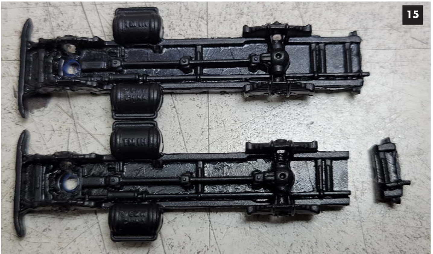
Image 15. In image 8 you see the chassis nearly comes to the end of the box. Now that the quarter round has been added the chassis needs to be shortened. The chassis on the right is the original length. The chassis on the left has been trimmed to provide clearance for the step.
