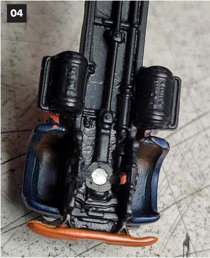
Image 04. Using a hobby knife I cut the hole for the axle even with the underside of the chassis.
