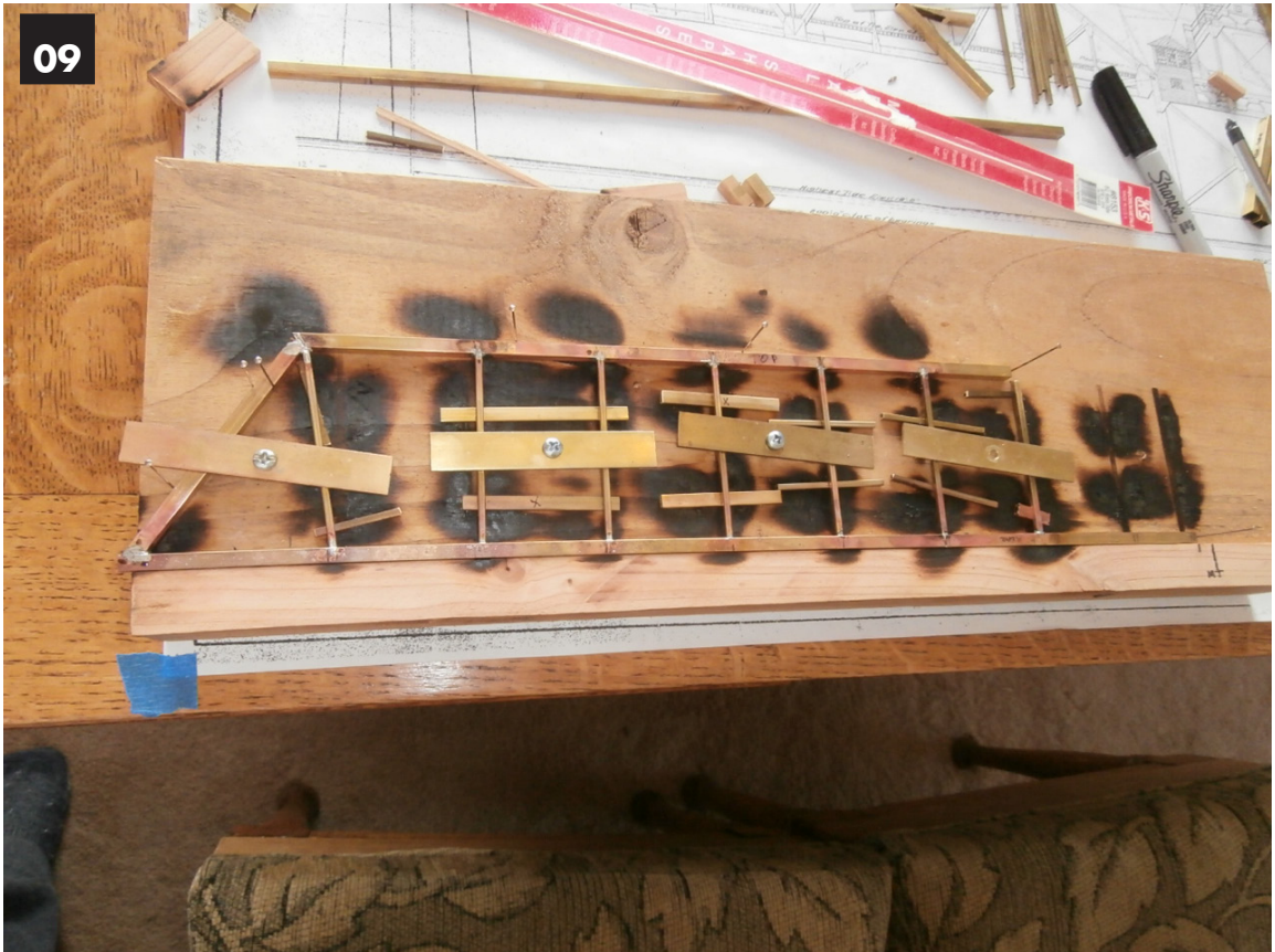
Image 09: East side of the bridge secured to the 2 x 6 the 1 x 2 board forms a straight edge for securing the parts. 1/2 x .062 plates to secure the components 1/16th square stock is used to space up the diagonals and verticals.
