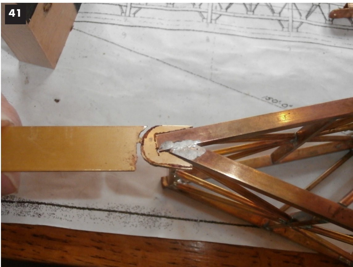
Image 41: The parts can be held in place while being silver soldered to the structure then they can be removed from the stock.
