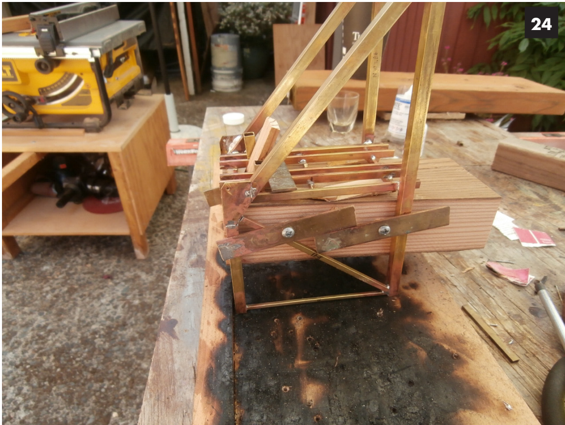
Image 24: Tower side X bracing is being silver soldered in place. At the center of the diagonal you can see the reference marks for the opposing braces which will be put in place next.
