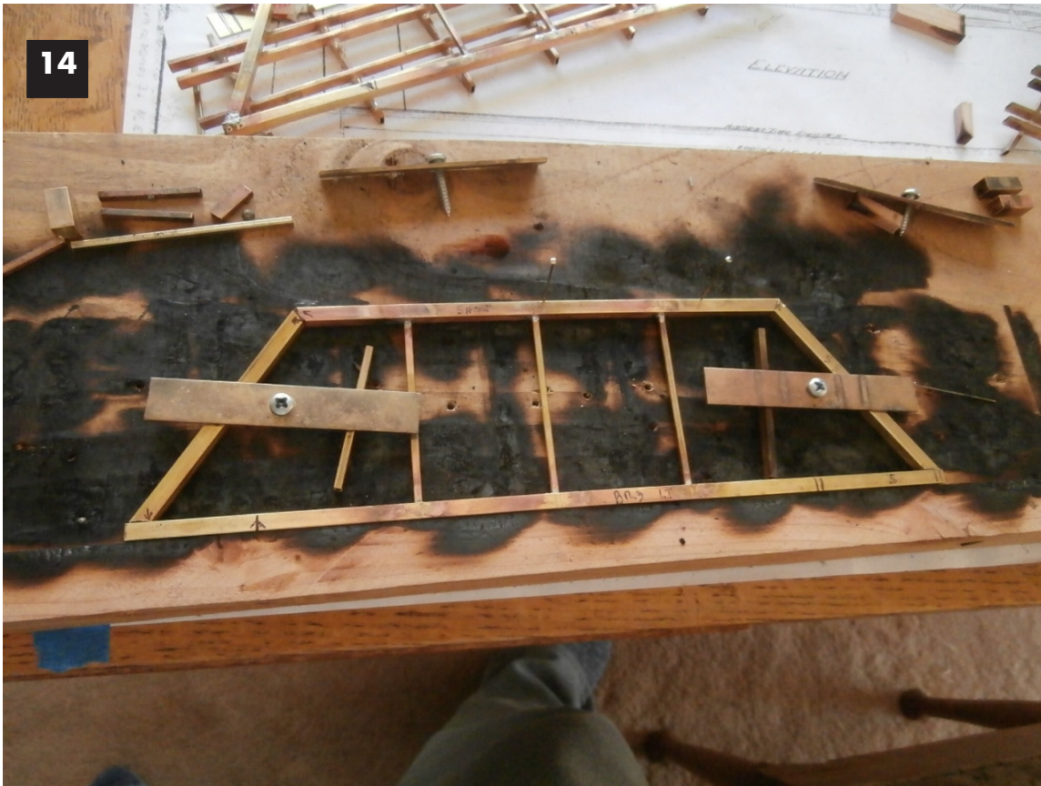
Image 14: Side of fixed span secured for silver soldering.
