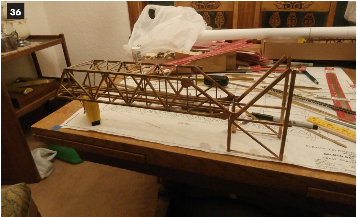
Image 36: This view shows a single rod crossing the tracks at rail level. This has to be replaced by separate pins so the tracks are not obstructed.
