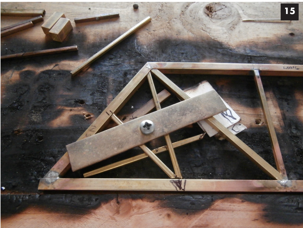
Image 15: Fixed span diagonals prior to silver soldering. Notice the beveled ends of each component and reference marks at adjoining locations. Also notice the left diagonal with a double bevel at the lower end.
