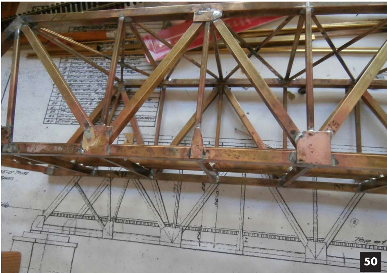
Image 50: Gussets silver soldered in place.
