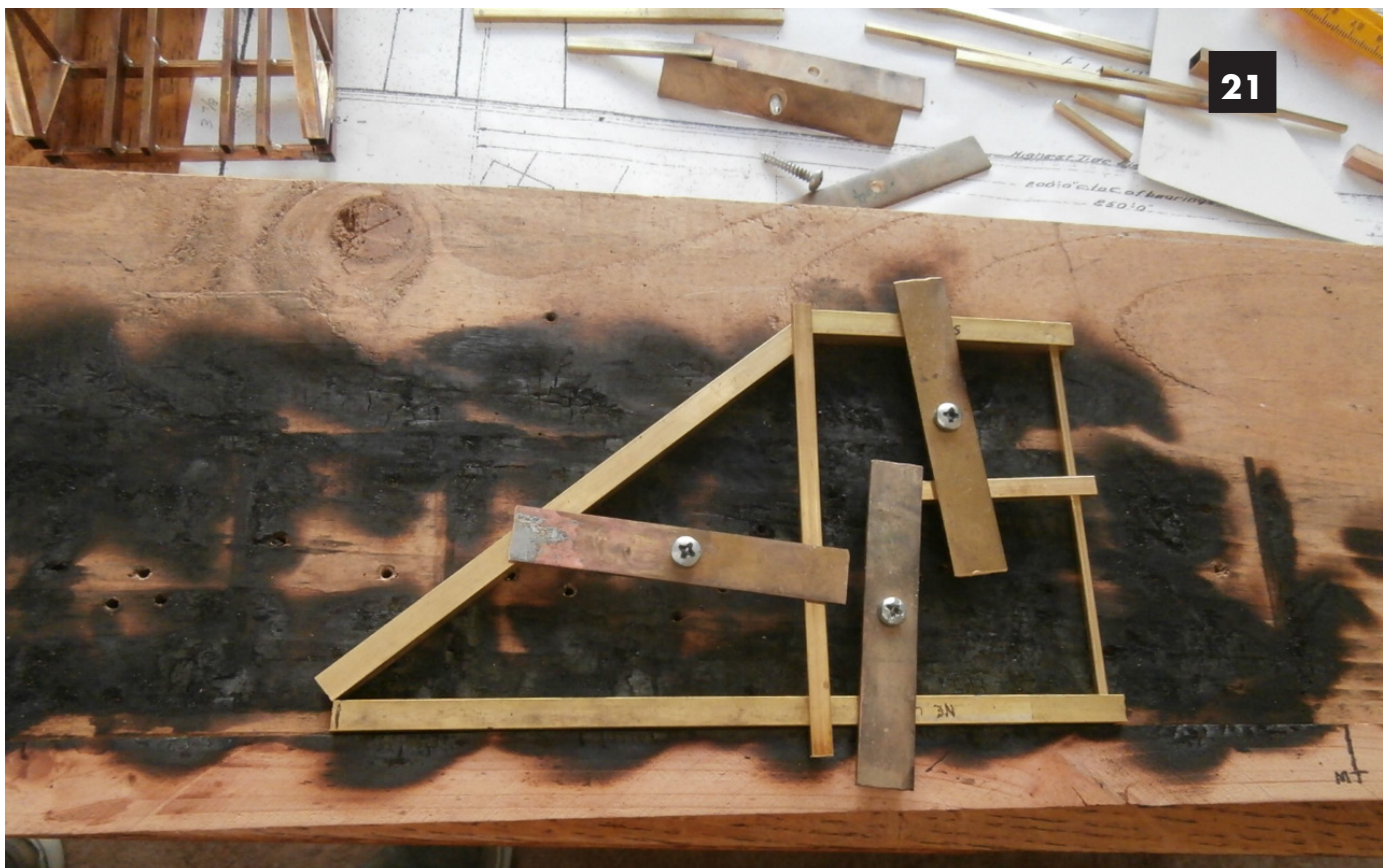
Image 21: North tower side components being located on 2 x 6 board.
