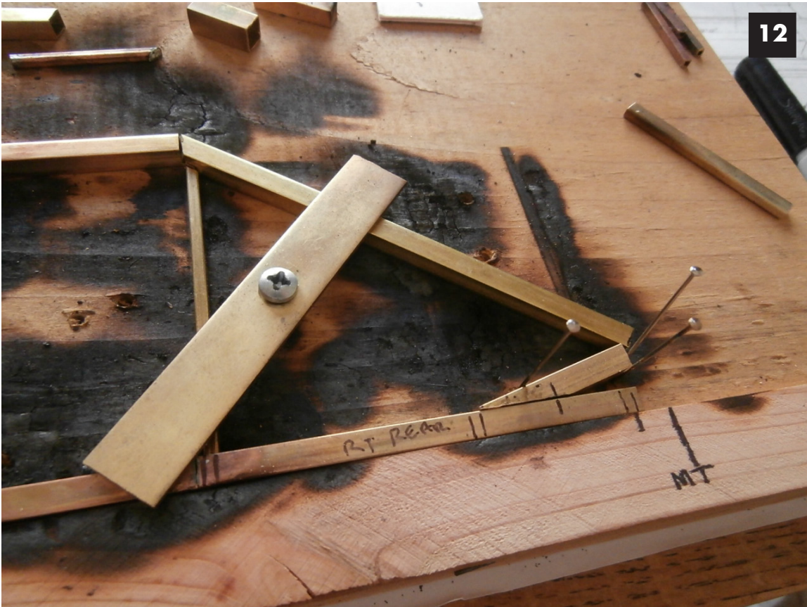
Image 12: North end truss detail pieces prior to silver soldering. These parts were cut with a 409 Dremel cut off disk.
