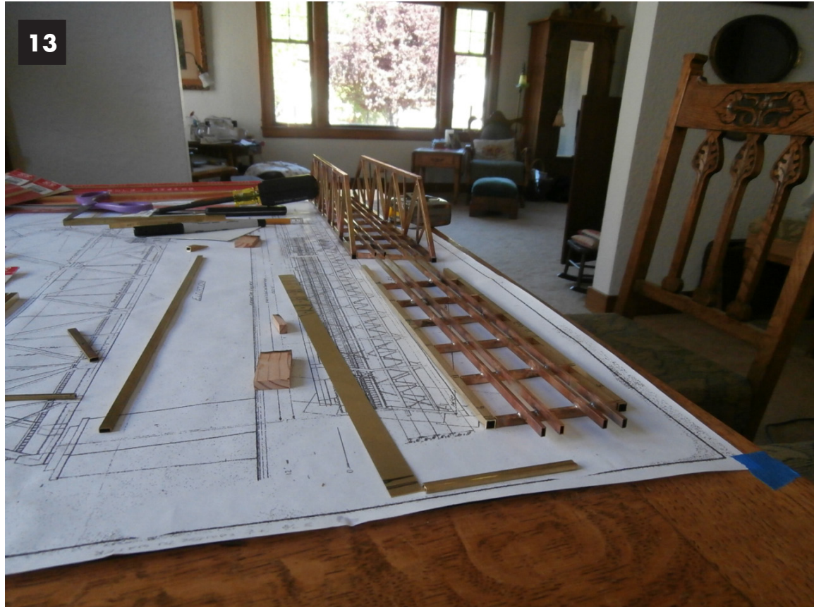
Image 13: Base of south fixed bridge. End nearest the camera is square. The far end is diagonal matching the lifting span.
