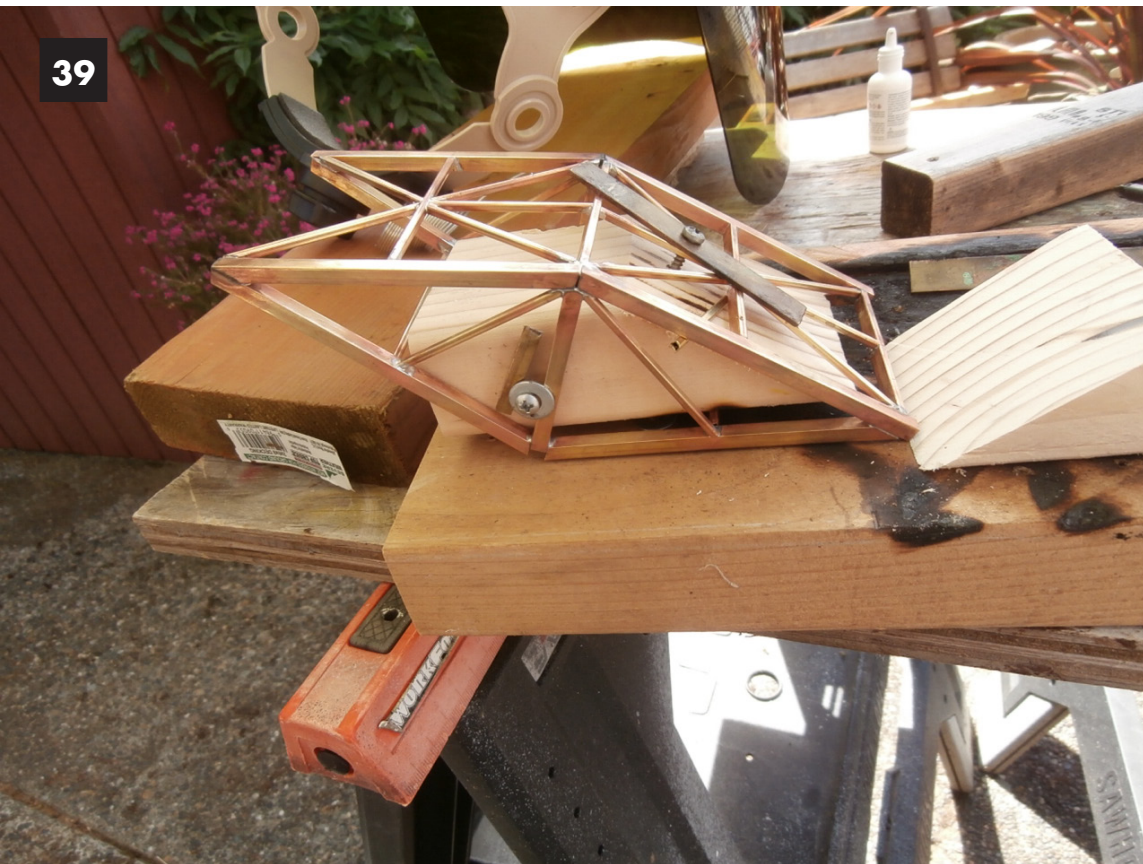
Image 39: Adjusting the block within the counterweight frame. One brace was removed so the block could be extracted then the brace was replaced without using the block.
