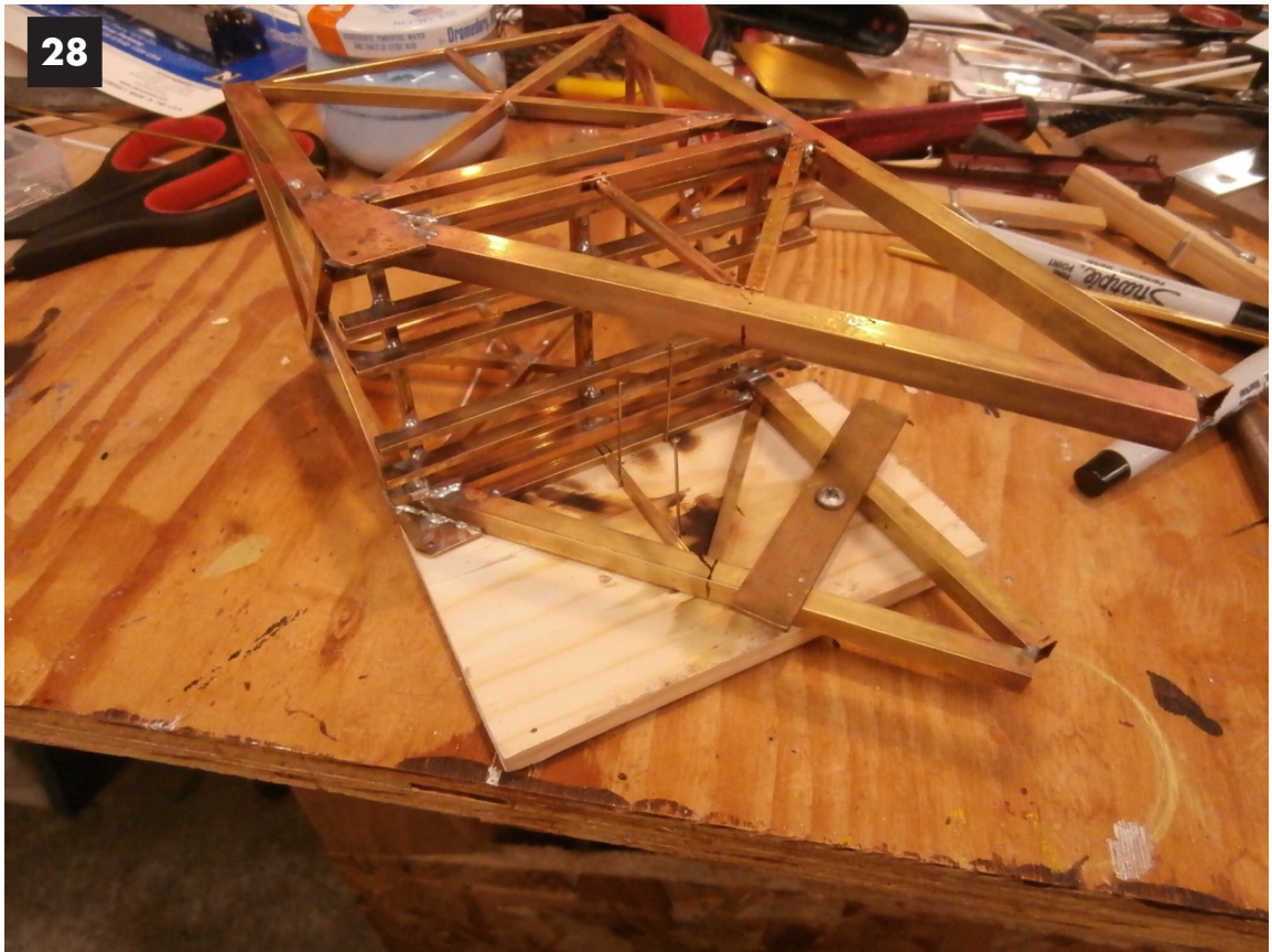
Image 28: Putting in two different sizes of bracing using straight pins instead if screws.
