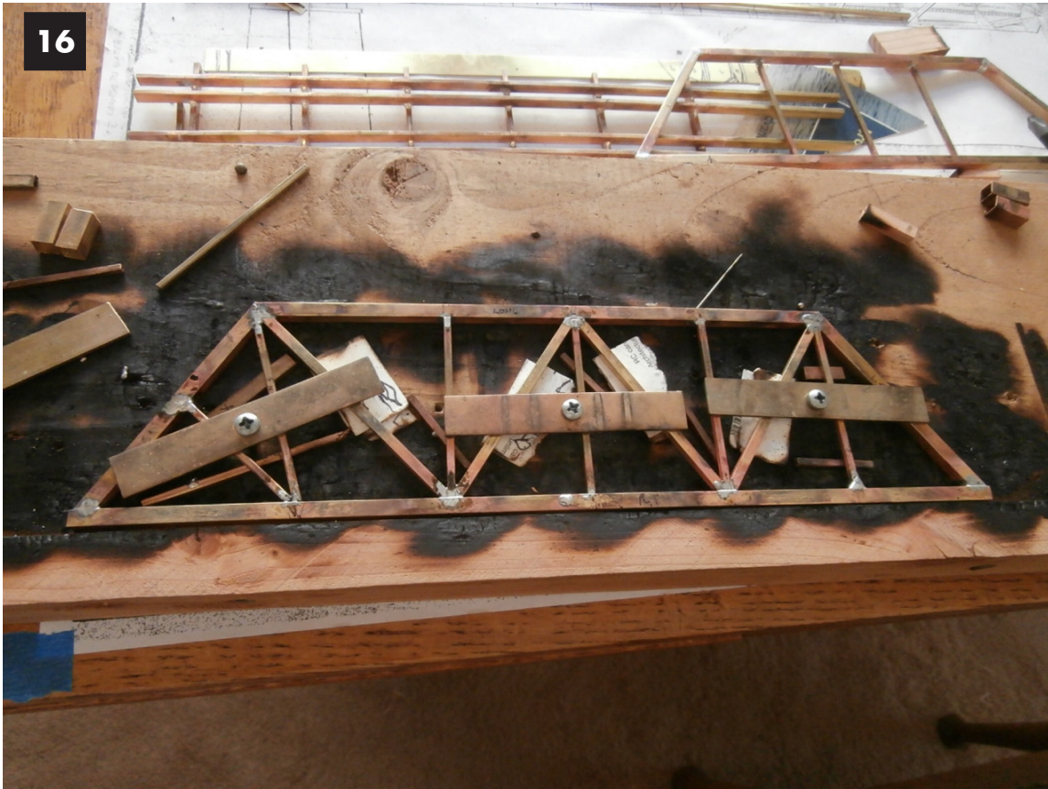
Image 16: Fixed span side after silver soldering.
