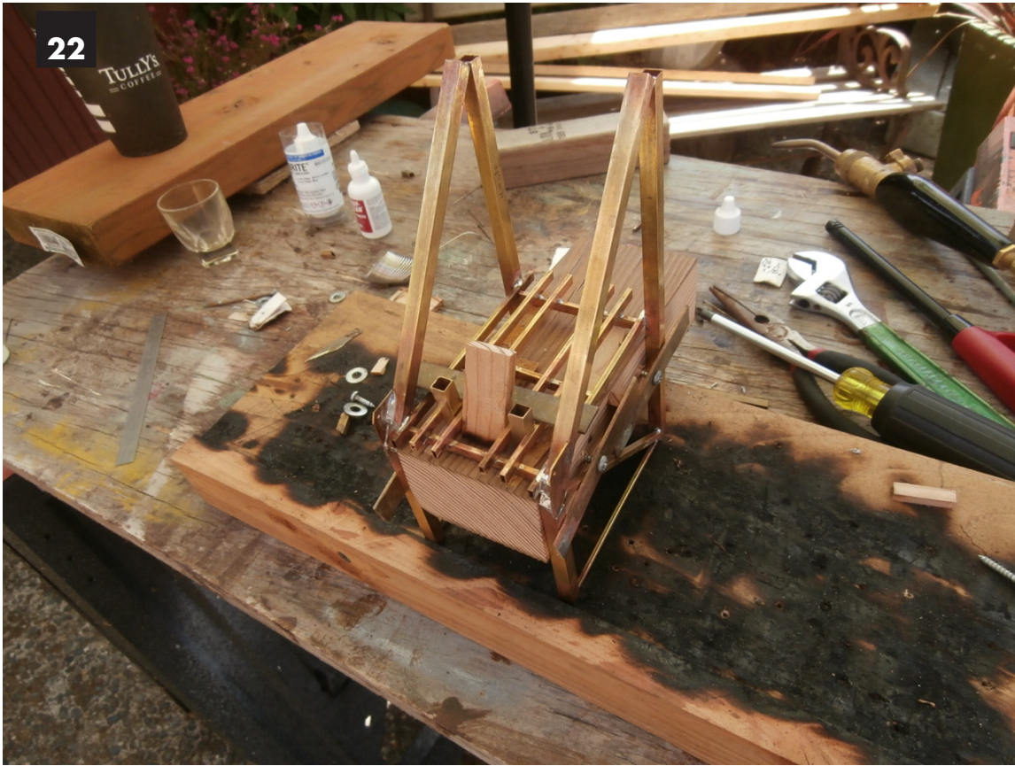
Image 22: Setting up the north tower sides and base. Care is taken to make sure that the sides sit flat and the track frame is level both ways. This view also shows the spacers used to locate the beams that hold the track. At the rear of the tower (far north end) the beam stick out ¼ inch beyond the frame so they can mesh into slots in the 1/2 inch plywood sub roadbed leading to the Ballard hill.
