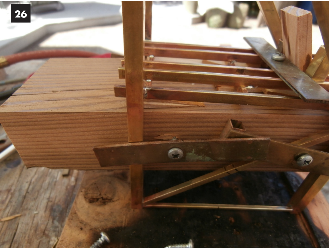
Image 26: Notice a small shallow wooden wedge which helps to accurately locate the assemblies.
