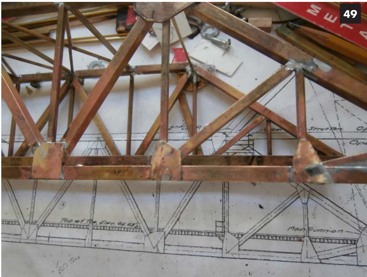
Image 49: Gussets silver soldered in place.
