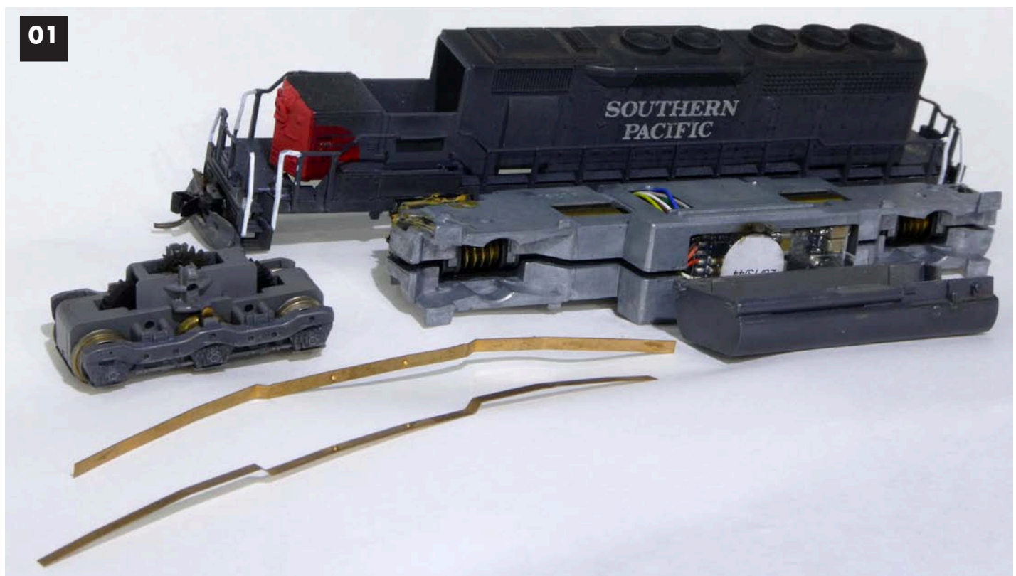
The shell and walkways should lift off with a little gentle prying from underneath. The tank also pops off and this allows the leaf contacts to come free. See figure 1 .
