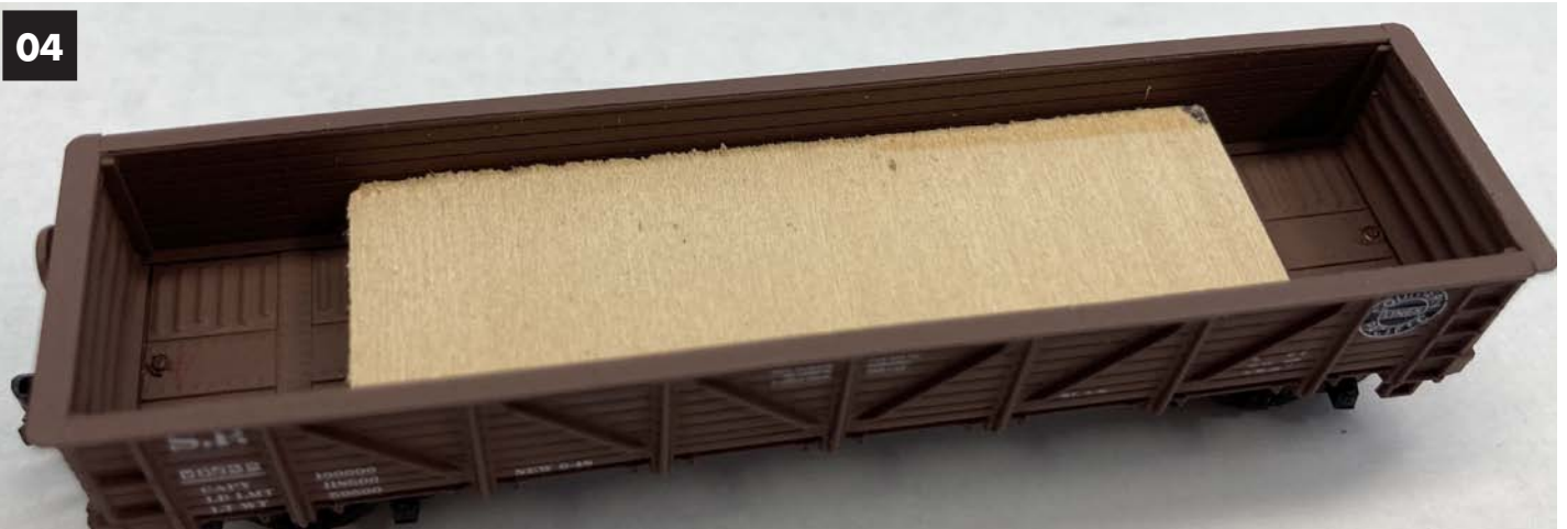
Image 04 shows the spacer needed to raise the load up to proper height in the car. For the original configuration GS car a 3/16" thick piece of basswood does the trick.
