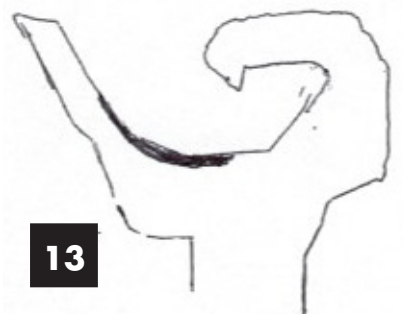
Image 13. Kato 11-702. Remove material in darkened area. A new X-acto #10 blade works best or a Dremel 409 disk. Turn it slowly!
