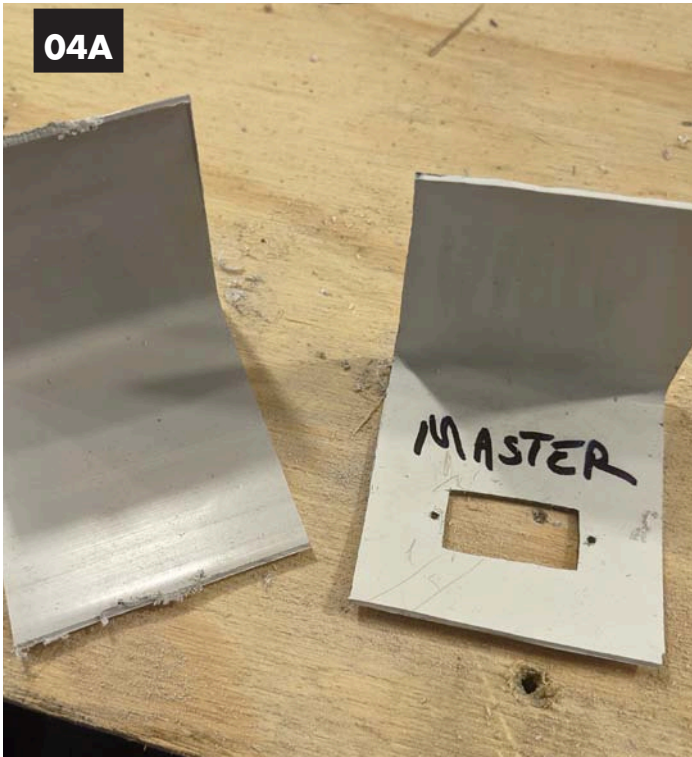
Image 04A, 04B. Line up the Master template to mark for the Servo opening.
