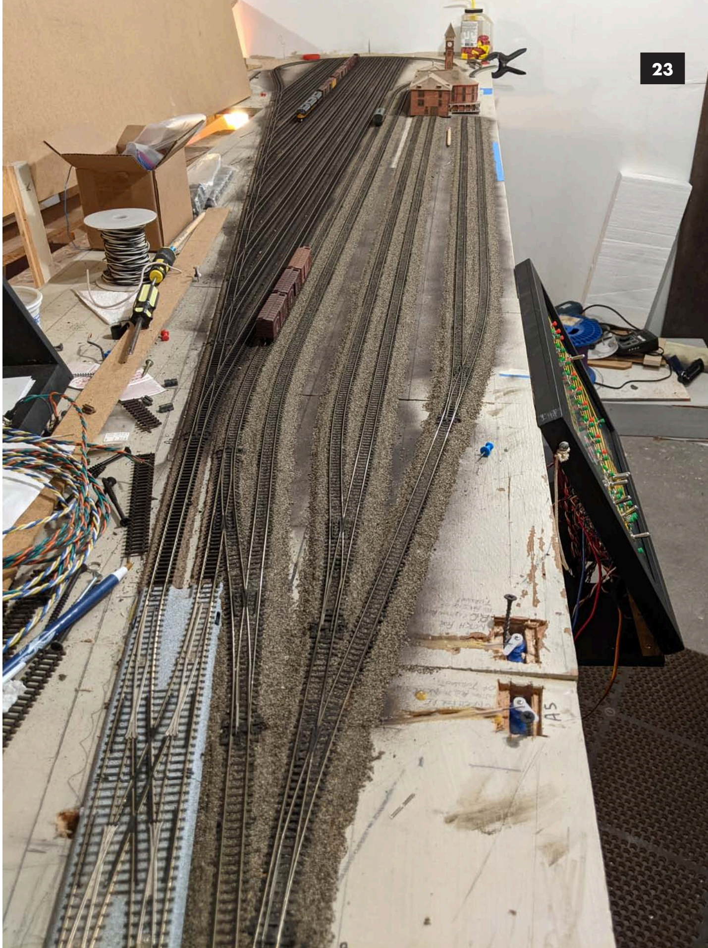
Image 23. The Portland yard throat. Notice a couple surface mounted servos bottom right. Sub roadbed bracing prevented them from being added under the turnout. They will be covered to hide their placement.
