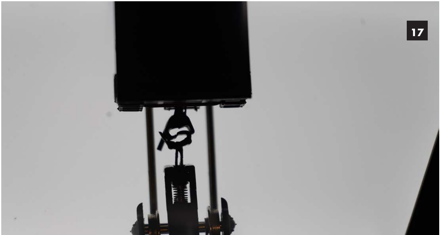
Image 17. Atlas gondola with coupler attempts to couple with unmodified a Kato 11-702 but couplers lockup before joining.
