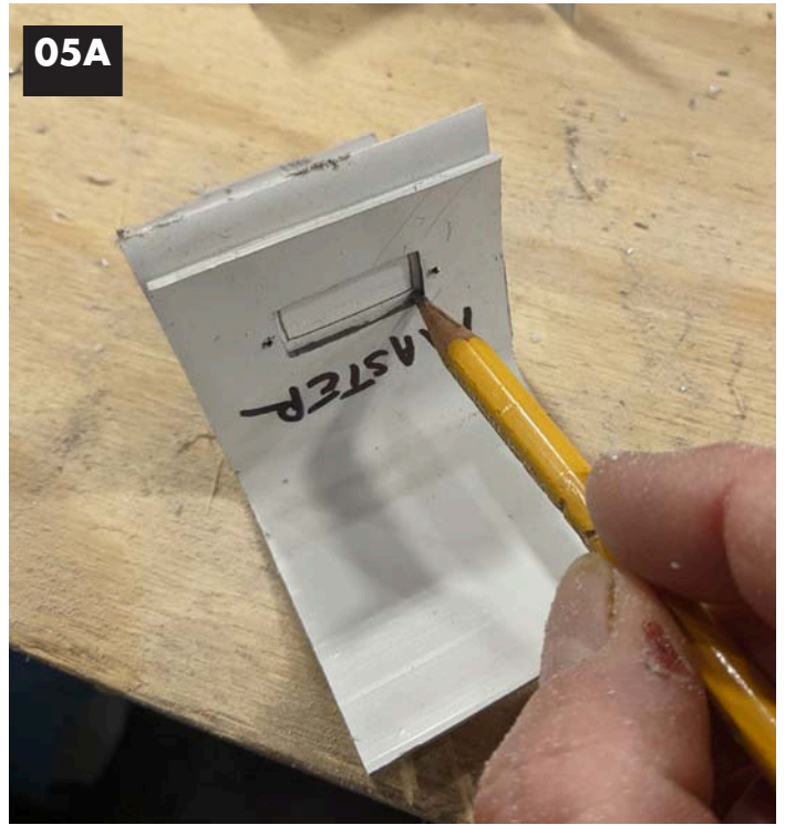
Image 05A, 05B. Mark the new bracket from the Master by backing the two pieces together.
