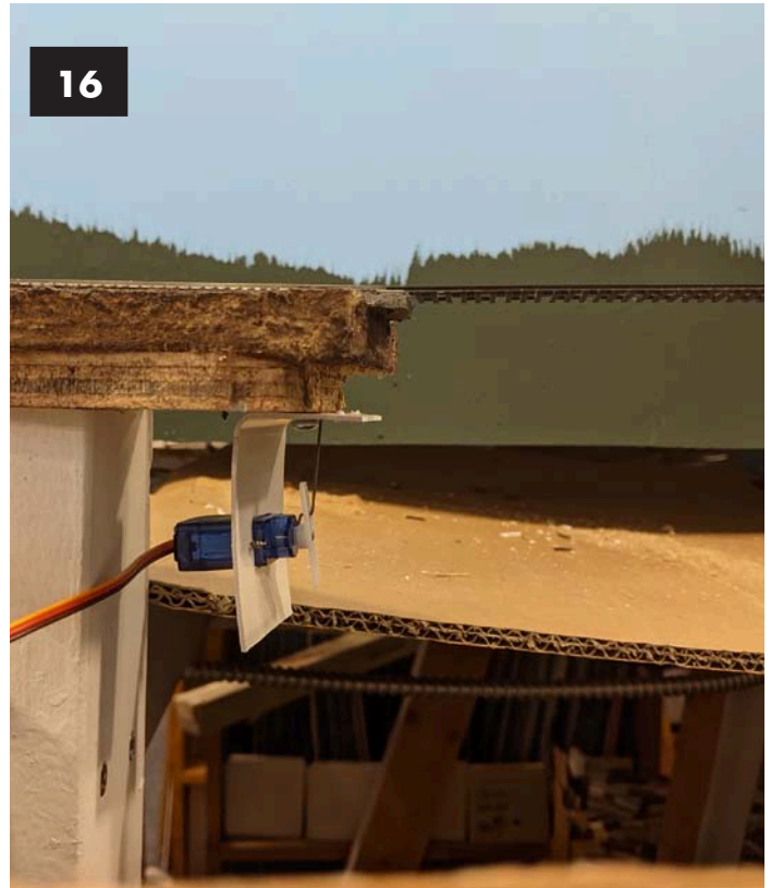
Image 16. After drilling a hole through the sub -roadbed under the Throw Bar hole I mounted the Servo Bracket under the turnout, fit the Throw Wire through the hole in the Throw Bar and made sure it was centered without obstructions, then tightened the mounting screws.
