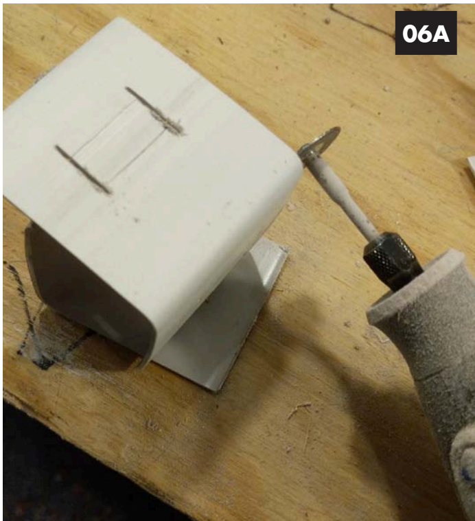
Image 06A, 06B. Cut the rectangular opening with a cut-off disc. You really don't have to worry about over-cutting the short side a bit as it doesn't affect the strength of the bracket.
