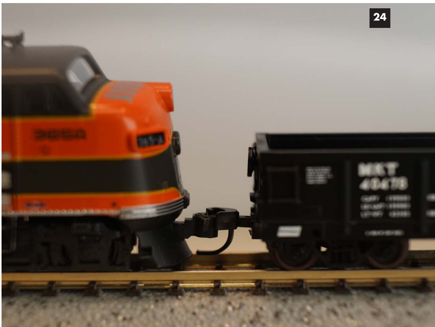
Image 24. Kato F7 with Kato coupler with Atlas car and AccuMate coupler and Truck. Notice excessive coupler height on this AccuMate also the close proximity of operating arm to locomotive pilot.
