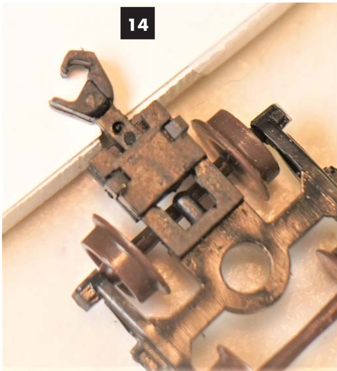
Image 14. Fixture for holding AccuMate coupler to trim two tiny points on the knuckle.
