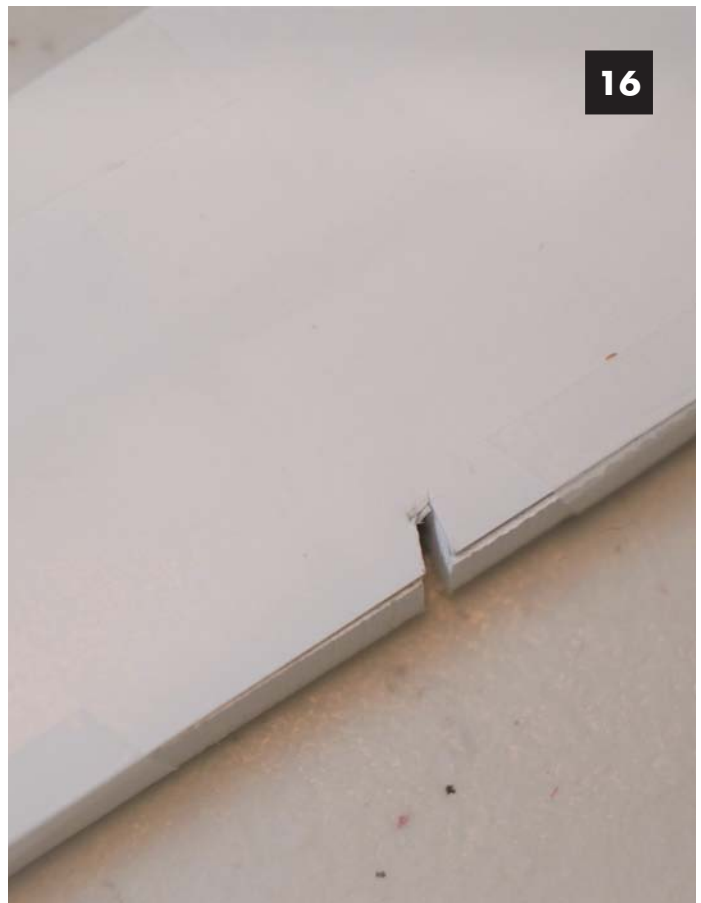
Image 16. The fixture consists of a PVC sheet with a sheet of paper taped on top to cover part of the slot for greater clarity in the photos.
