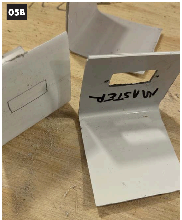
Image 05A, 05B. Mark the new bracket from the Master by backing the two pieces together.
