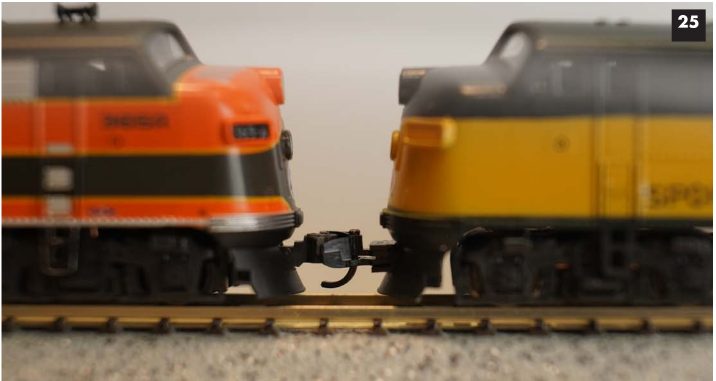
Image 25. Kato F7 with modified Magnetic coupler on left coupled to Kato F3 with MT underslung body mount coupled with slightly shortened coupler pin.
