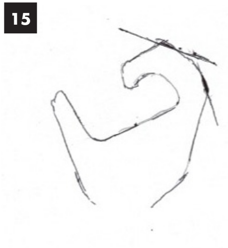
Image 15. AccuMate modification. Remove material in darkened areas. A new X-acto #10 blade works best. High magnification improves accuracy in removing material.
