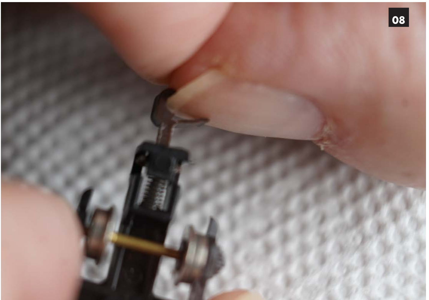
Image 08. Bending a Unimate with thumb nail to relax the coupler's grip. Bend slowly and be careful not to over-bend. You can always bend it again if you don't bend it too far.
