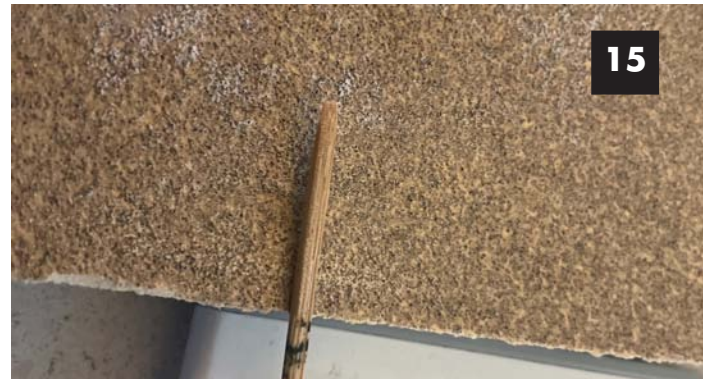
15. Then I sanded opposite sides to flatten the round skewer.
