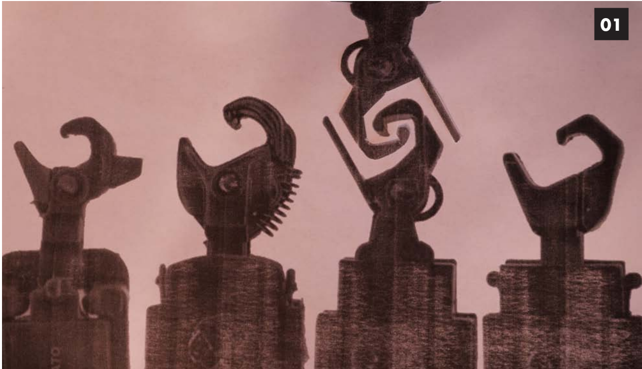
Image 01. Photo of enlarged image from Mike Fifer / Peter Wisniewski article with cut out. MT coupler for comparison. From left to right: Kato's current magnetic coupler, McHenry, Micro-Trains N coupler, and the Atlas Accu-Mate.
