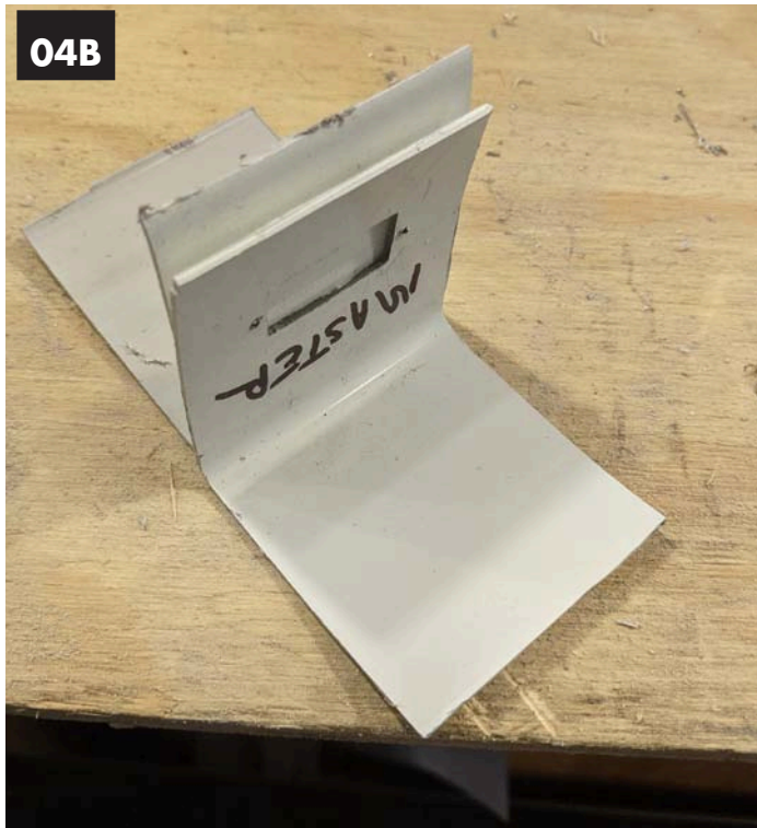
Image 04A, 04B. Line up the Master template to mark for the Servo opening.
