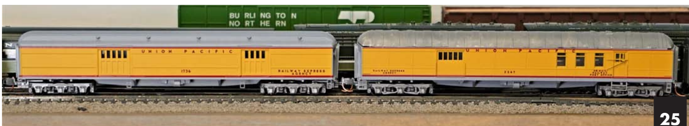
Image 25. Both cars with modified MTL 1018s coupled together. At this point we're not worried about close coupling like we're concerned about derailing in the tight radius track when backing up to reverse the consist.
