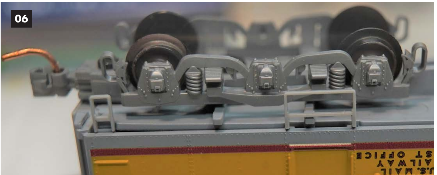
Image 06. 3 axle MTL body mount RPO truck with center axle removed and coupler in place.
