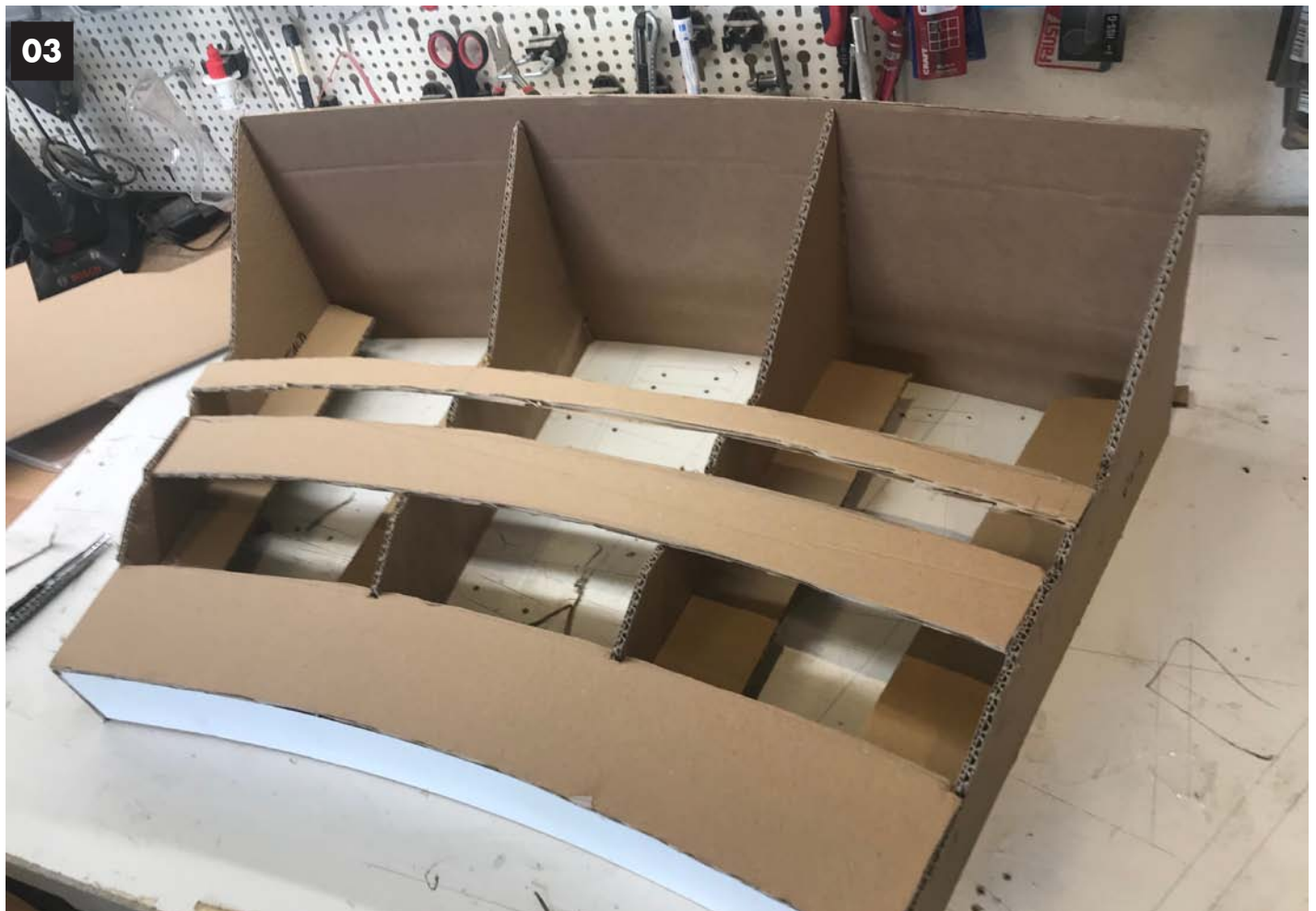
Image 03. Adding front and back walls plus strips of cardboard for the track, street and river. I used hot glue throughout construction as it dries very fast. It starts to look like a module, though without a proper landform it was still difficult to visualize how trains and cars would look like.
