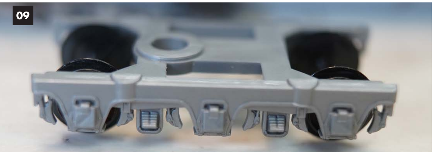
Image 09. MTL Baggage car body mount truck.
