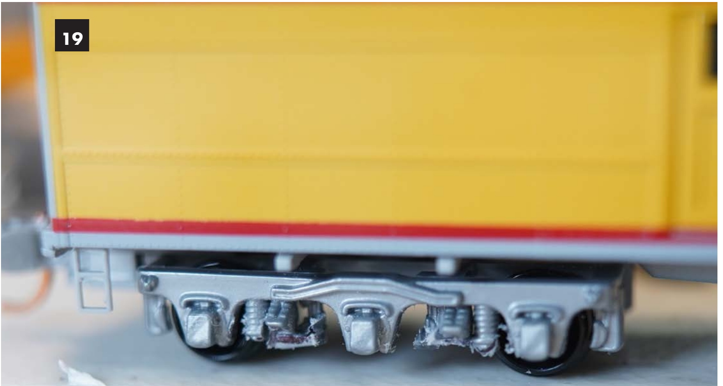
Image 19. Modified MTL1018 on MTL baggage car.
