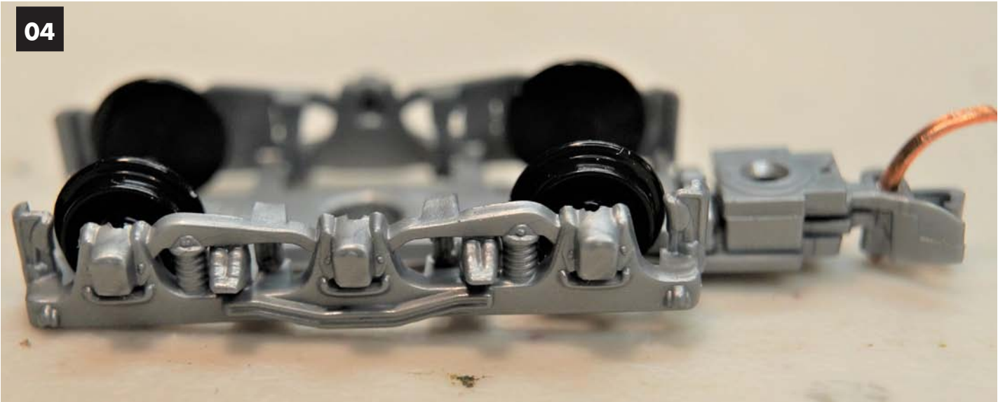
Image 04. MTL1018 3 axle truck with center axle removed.
