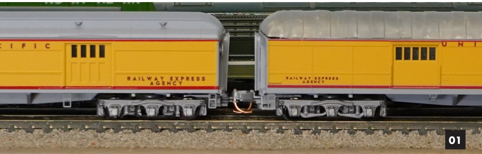
Image 01. The MTL Baggage/Express and RPO/Express cars with truck mounted couplers.
