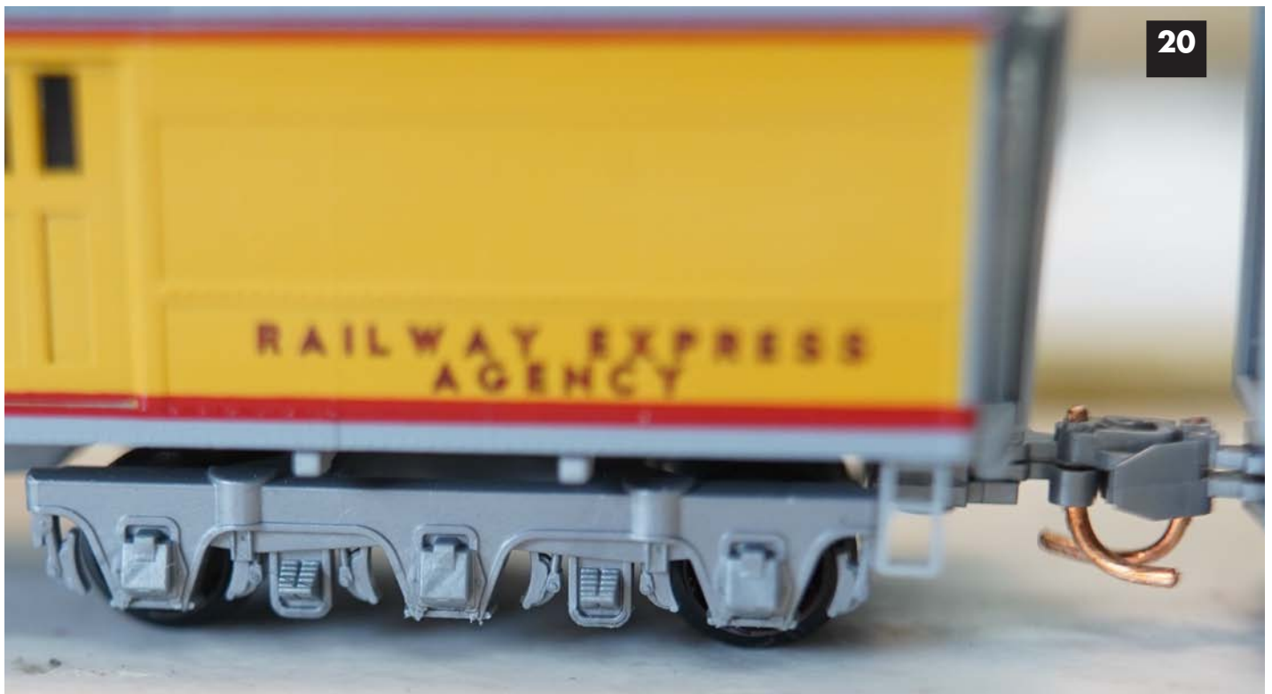
Image 20. 3 axle body mount truck and coupler on baggage car.
