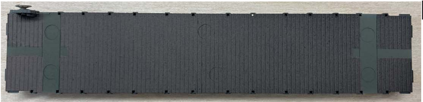
Image 05. I let the Smoke dry for about one-half hour then get out the Tamiya TS-80 “Flat Clear”. If this is a new item for you and you have used Testor’s Dull Cote before, be in for a surprise. The Tamiya sprays far better and does not yellow over time. All my freight cars get a flat clear finish before being layout ready.
