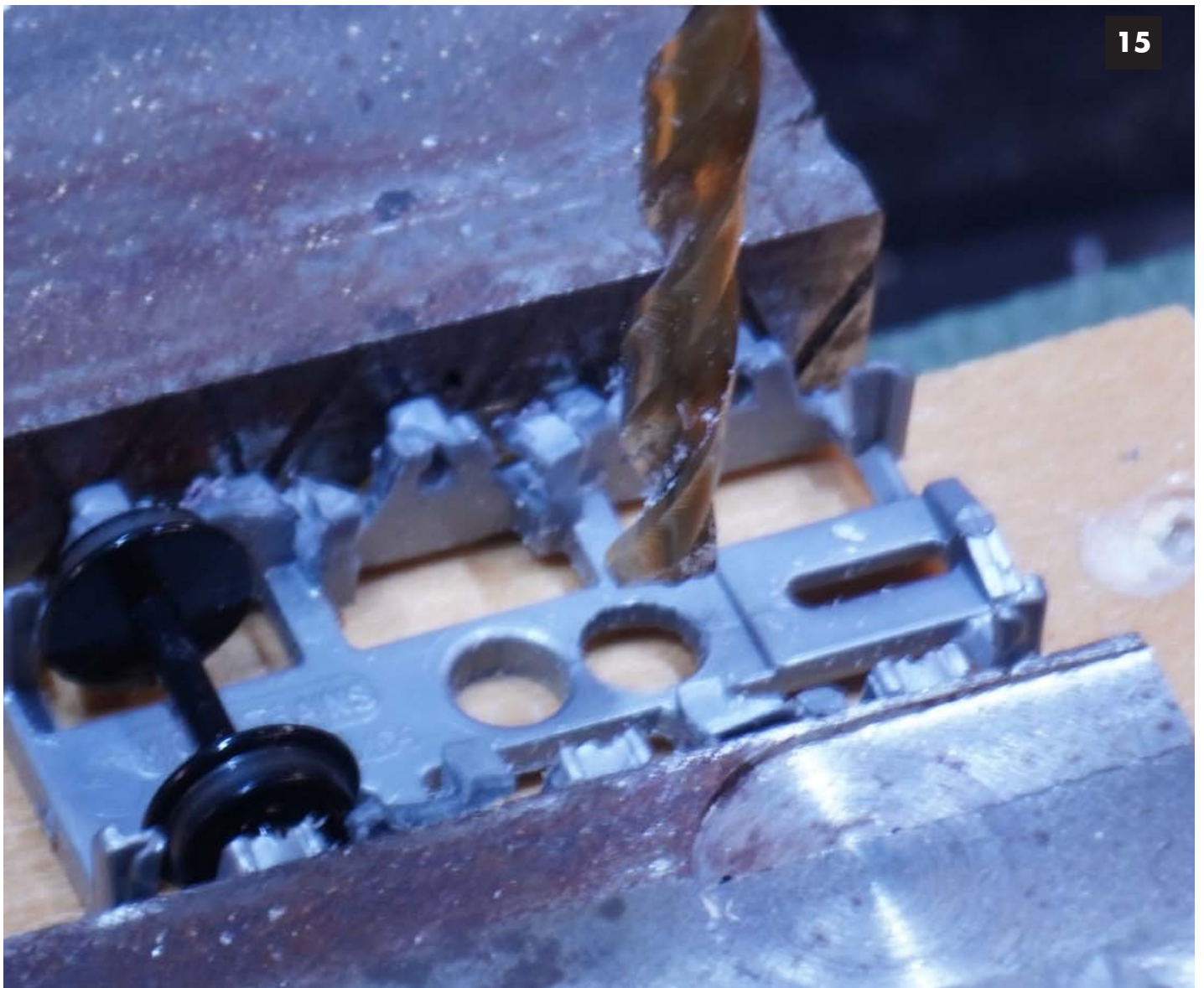
Image 15. Finishing the new bolster pin hole with a #42 drill. The pilot hole was moved over with a tiny round file prior to finish drilling.
