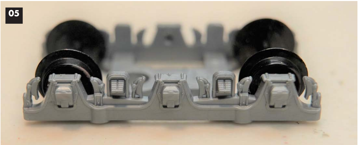
Image 05. 3 axle MTL body mount truck with MTL 1007 wheels and center axle removed.
